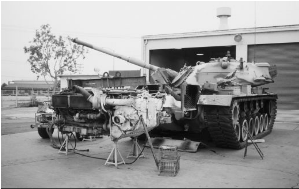
The Continental 12-cylinder supercharged AVDS-1790-2D air-cooled diesel engine and transmission have been removed from the California Army National Guard M48A5PI tank pictured. Top speed of the M48A5PI tank on a level road was 30mph (48kph) and it had a cruising range of about 300 miles (483km). Michael Green
