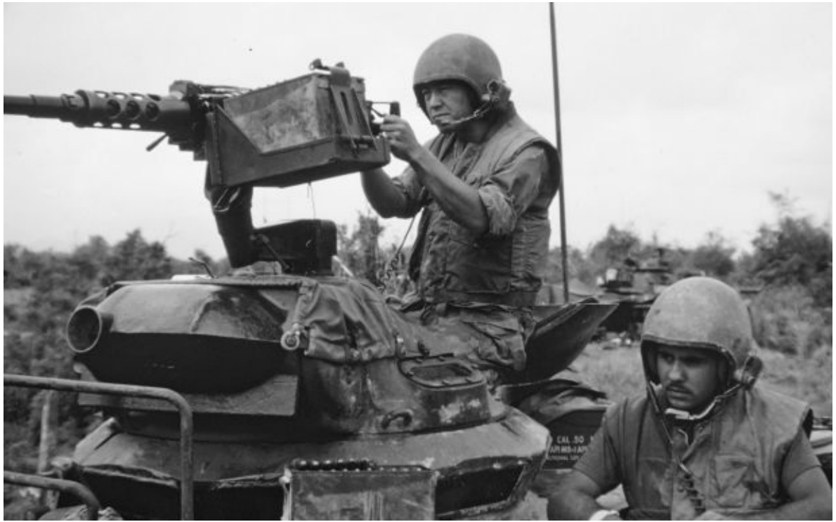
A close-up photograph of the mounting arrangement of a .50 caliber (12.7mm) machine gun on an M48A3 (Mod B) tank fitted with the G305 turret riser. The machine gun mount is welded to the front of the M28 periscope sight located in the roof of the M1 cupola that was used to aim and fire the weapon when mounted inside the cupola. Patton Museum
