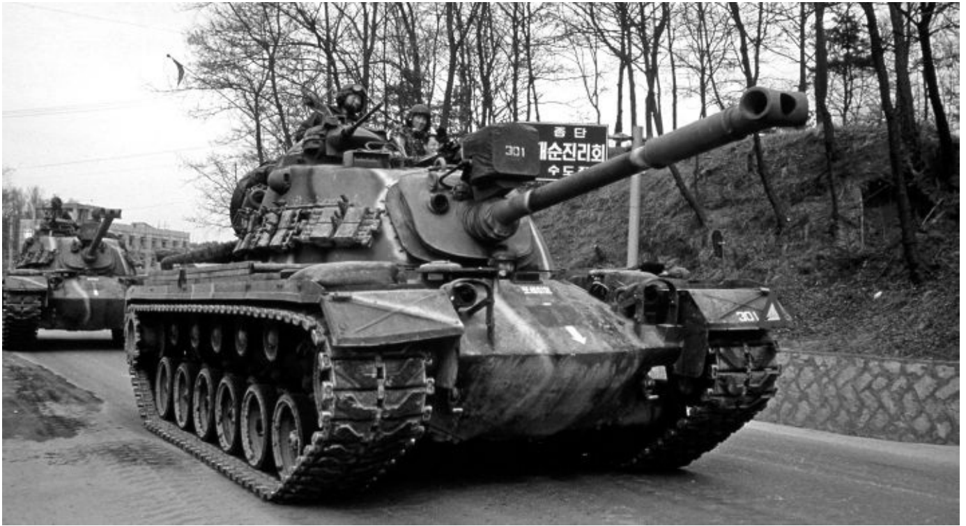
A convoy of South Korean Army M48A3 tanks passes by the photographer during a training exercise. The vehicles are fitted with an IR/white light searchlight. It is reported that the South Korean Army M48A3 tank inventory has been fitted with an indigenously-designed fire-control system. Vehicles so modified are designated as the M48A3K tank. DOD
