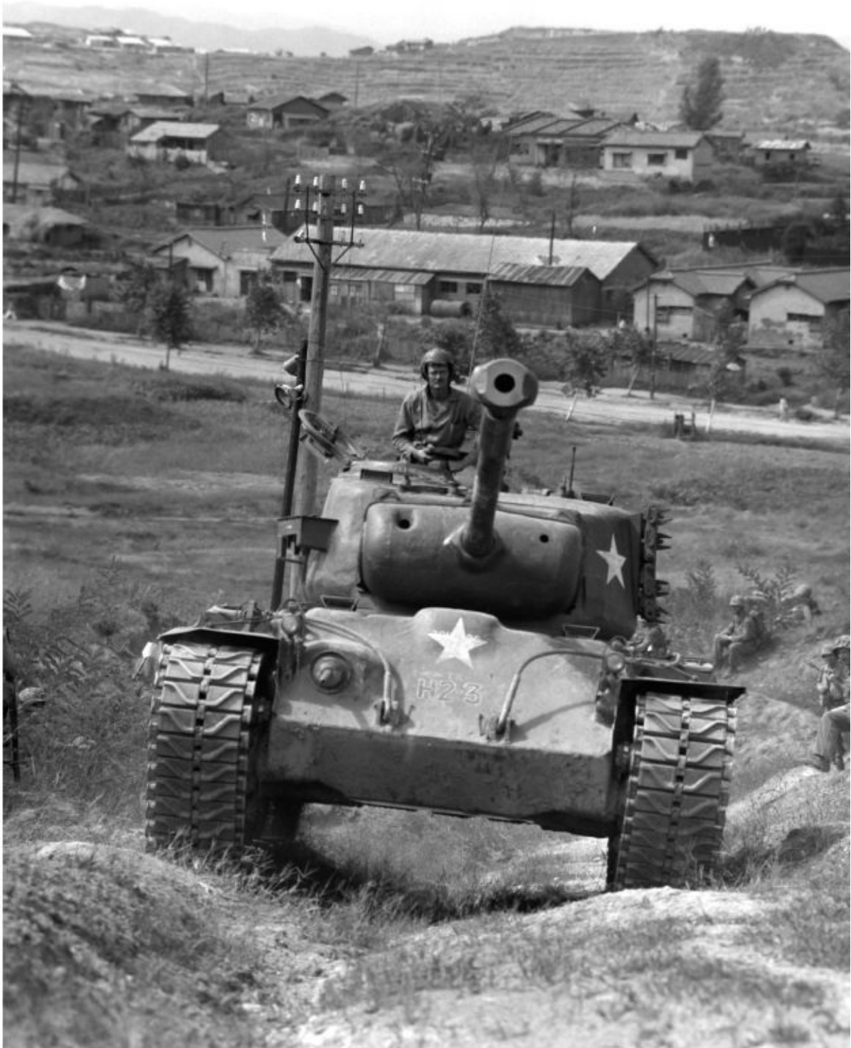
A U.S. Marine Corps M46 tank is pictured doing a bit of hill-climbing during the Korean War. The smaller of the two holes in the tank's gun shield is the opening for the .30 caliber (7.62mm) coaxial machine gun. The larger hole is for the gunner's magnified telescope sight. The gunner also had a magnified overhead periscope sight. Patton Museum
