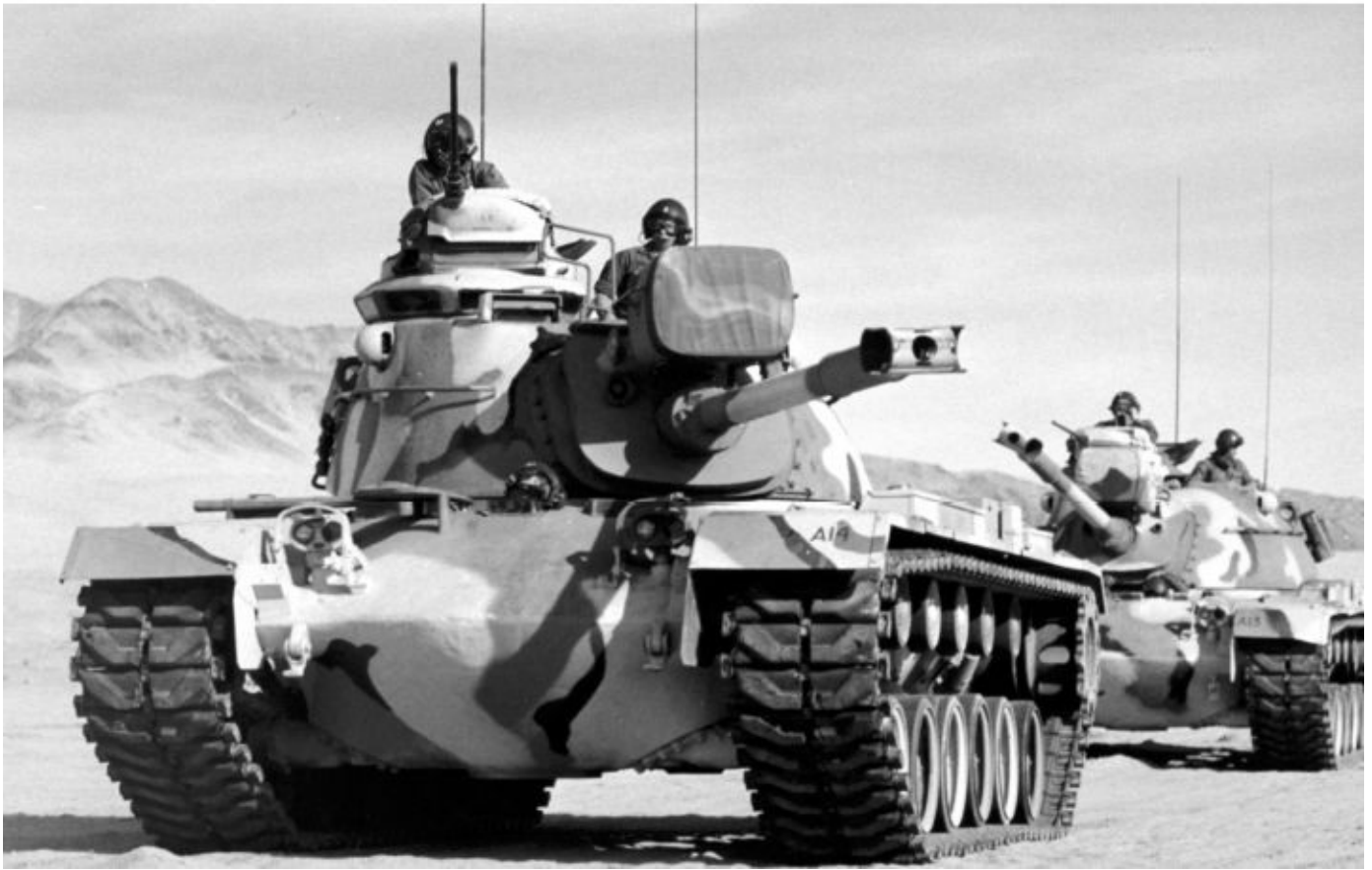
In this picture can be seen two late-production M48A3 (Mod B) tanks in service with the U.S. Marine Corps during a training exercise. Late-production M48A3 (Mod B) tanks can be readily identified by their identical headlight clusters and squared brush guards that first appeared on the M48A2 tank. DOD
