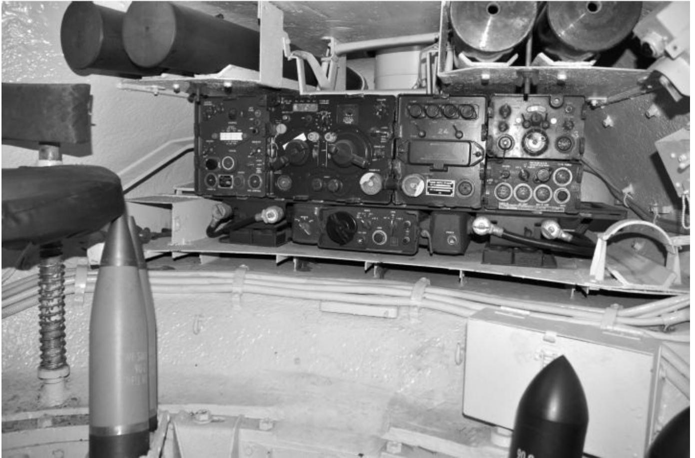
An interior picture of a restored M47 tank belonging to the Military Vehicle Technology Foundation (MVTf) shows the vehicle's radio rack and radio with storage space for four main gun rounds above it. Behind the radio is the tank's electrically operated ventilation blower. Chris Hughes
