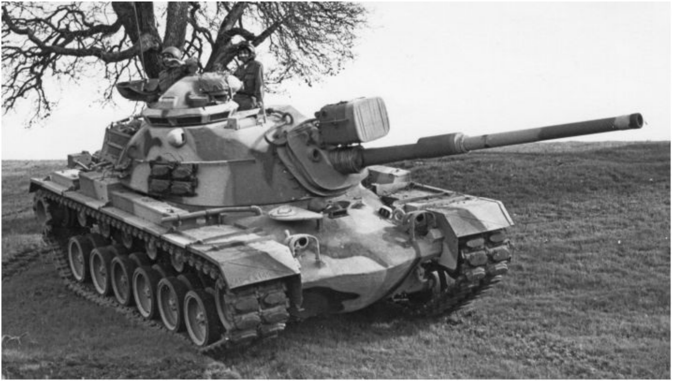
The bulk of the U.S. Army's inventory of M48A5 tanks served with U.S. Army National Guard and U.S. Army Reserve units up till the 1990s. The vehicle pictured belonged to the California National Guard and is equipped with the G305 turret riser it inherited from a M48A3 (Mod B) tank. Michael Green
