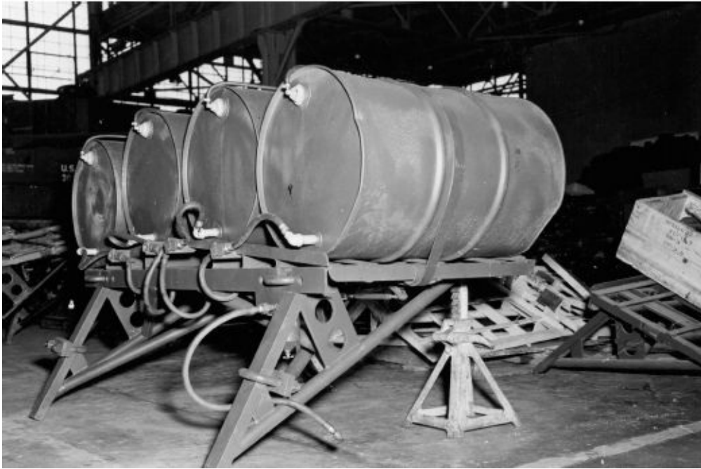
This picture shows the arrangement of the four unarmored 55 gallon fuel drums that were attached to rear of the M48A1 tank and connected to the vehicle's fuel system. The additional fuel supply nearly doubled the operational range of the M48A1 tank to 135 miles. Patton Museum
