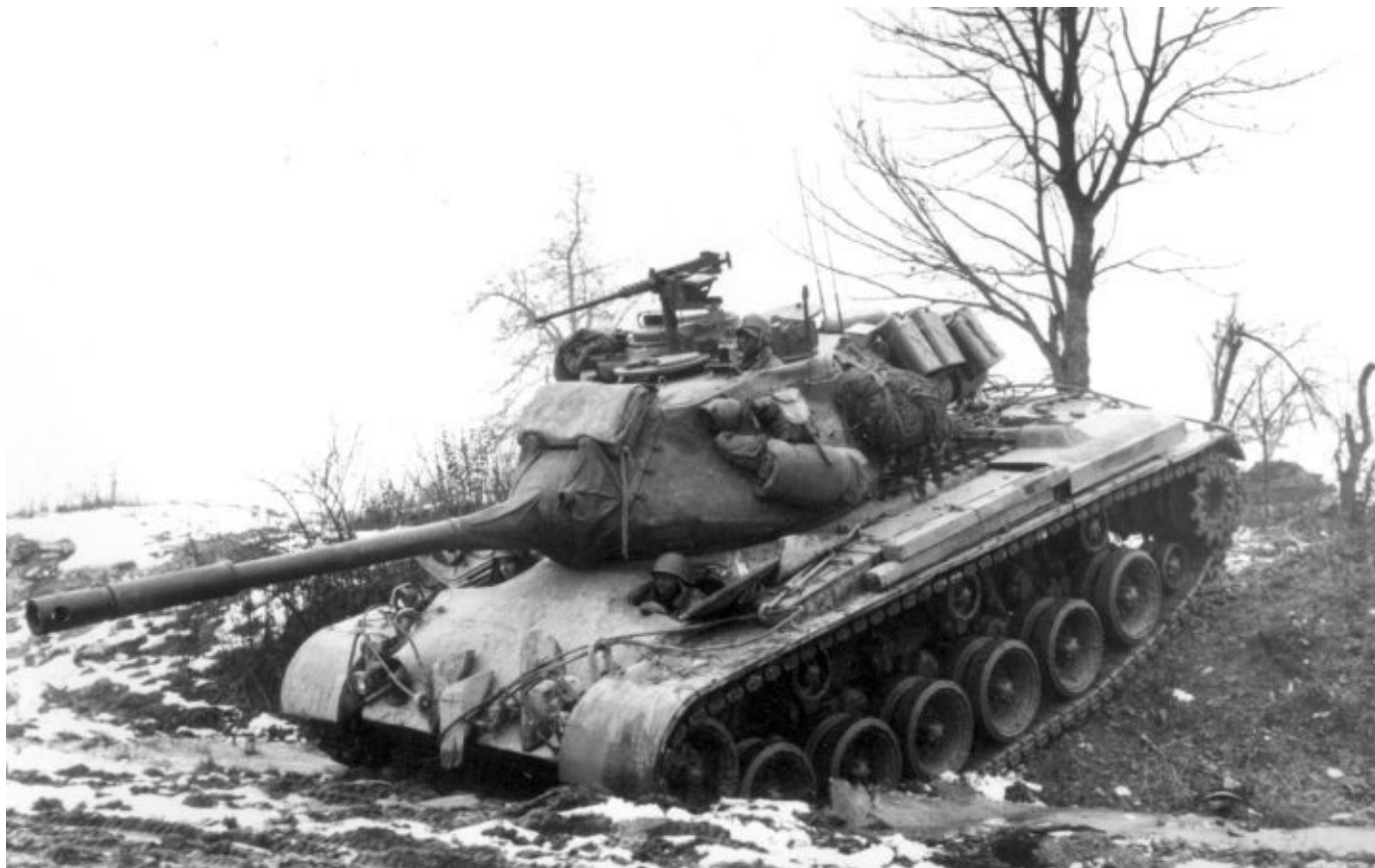
This U.S. Army M47 tank is on field maneuvers. There were 1,700 rounds of ammunition carried onboard the vehicle for the .50 caliber (12.7mm) machine gun that was mounted on the turret roof. The weapon had a rate of fire of 450 to 550 rounds per minute. Patton Museum
