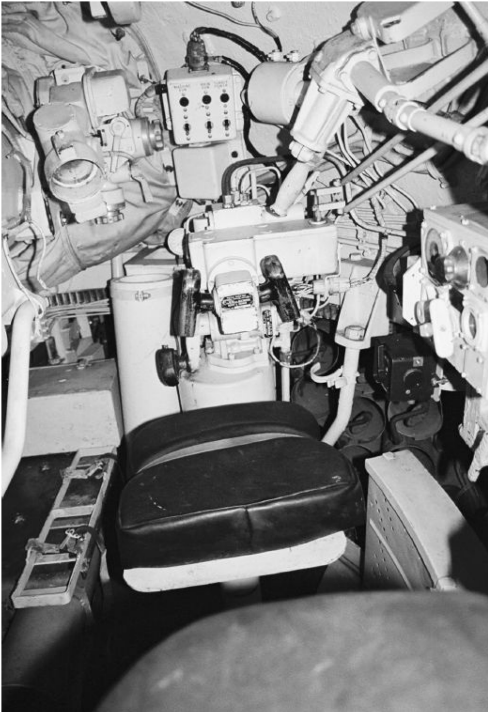
Visible from the tank commander's position on an IDF Magach 3 is the gunner's seat. Directly in front of the gunner's seat are the black hand grips of his main gun control handles, nicknamed the "Cadillacs" by American tank crews because they were designed and built by the Cadillac Gage Company. Michael Green
