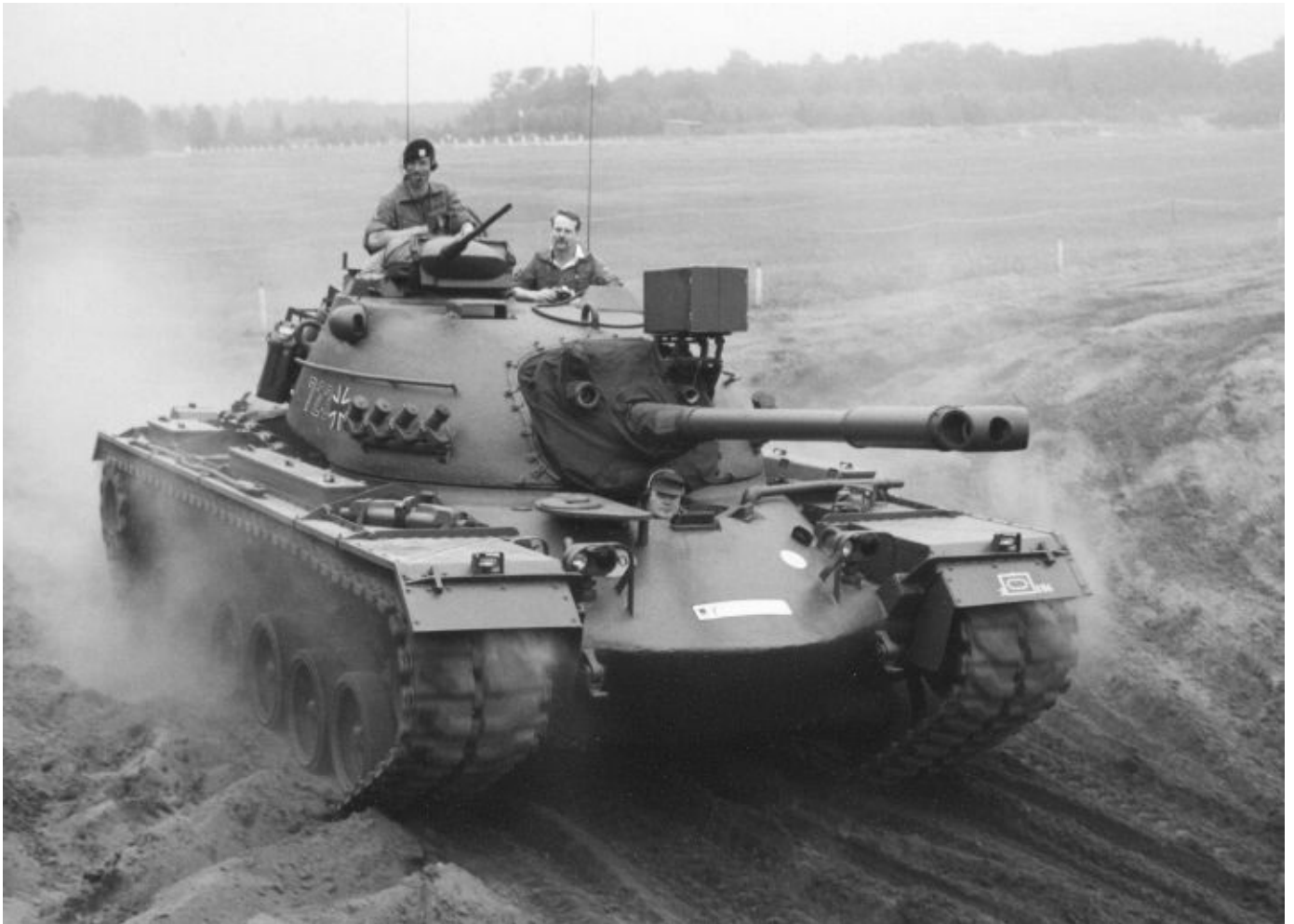
On a demonstration run is an operational M48A2C tank belonging to the German Army tank museum. The first M48 series tanks were delivered to the West German Army in 1958. The German tankers considered them much more reliable than the M47 tank. Thomas Anderson
