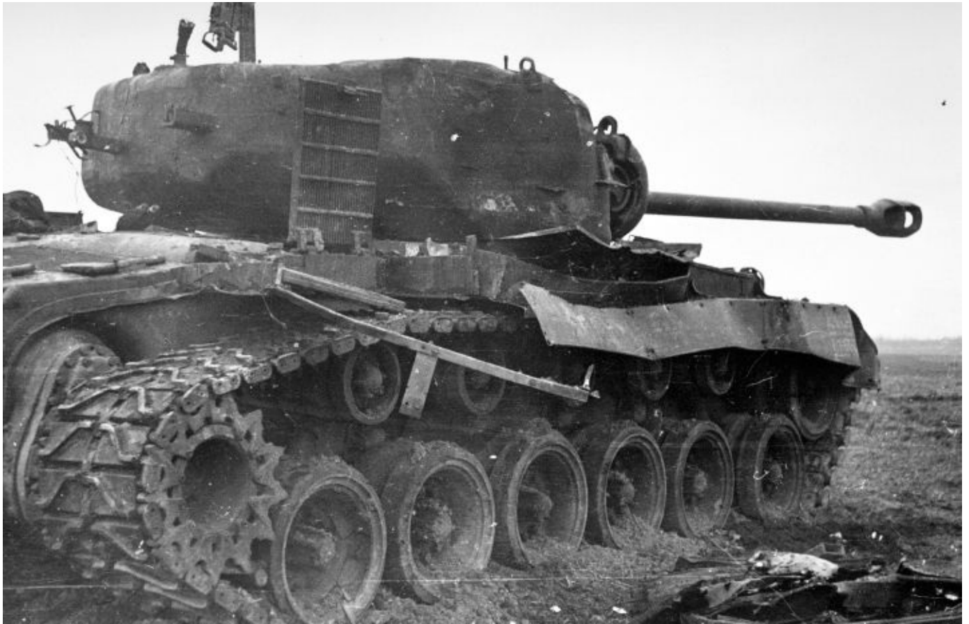
On March 1, 1945, another U.S. Army T26E3 tank (serial number 22) was knocked out by two German high explosive (HE) rounds that caused extensive damage to the vehicle's turret and running gear as seen in this picture. Notice the tank commander's cupola on the ground next to the vehicle. Patton Museum
