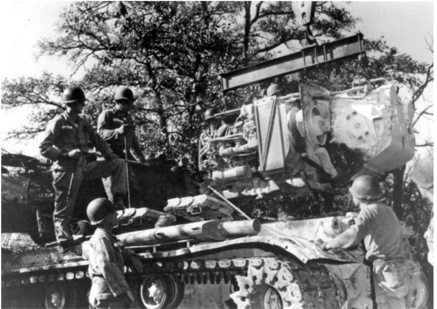
A group of U.S. Army soldiers are shown removing the power pack of an M47 tank, which consisted of a Continental 12-cylinder air-cooled, gasoline-powered, AV-1790-5B engine and an Allison Cross-Drive CD-850-4 transmission. The vehicle's engine is on the left and the transmission is on the right. Patton Museum
