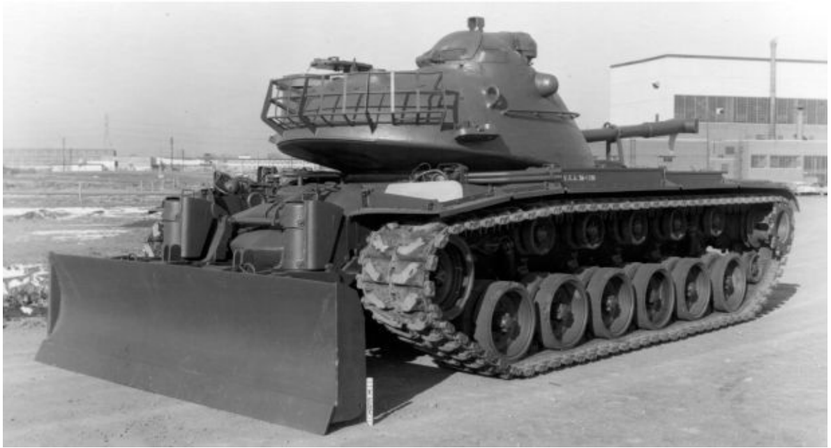
A factory photograph taken at the Detroit Arsenal shows an M48A1 tank with the tank-mounting, bulldozer M8, shown in its lowered position. What is interesting in this picture is the fact that the headlight arrays have been moved to the vehicle's front fenders. TACOM
