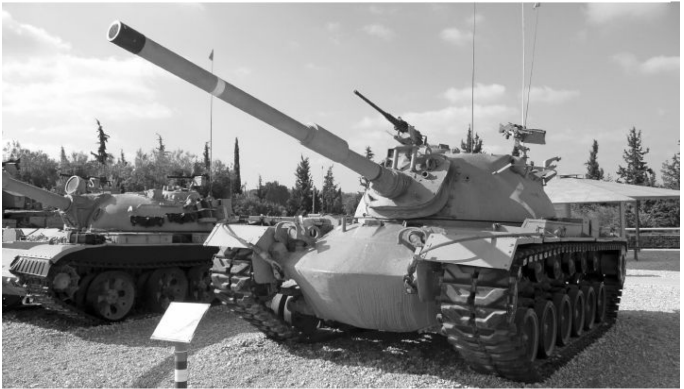
Forming part of the collection of the Israeli Armored Corps Memorial Site and Museum is this Magach 3 with an Urdan low-profile cupola. The .50 caliber (12.7mm) machine gun fitted directly over the vehicle's gun shield was intended to take out targets that did not merit a main gun round. Vladimir Yakubov
