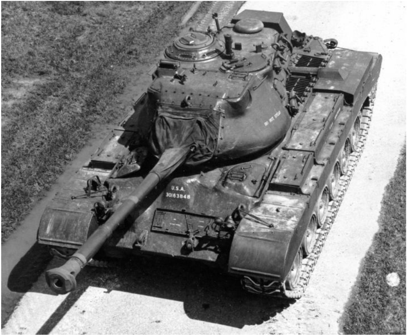
Prior to approving production of the M47 tank, a single pilot vehicle was created that mated a T42 tank turret onto an M46 tank chassis. The hybrid vehicle was designated the medium tank M46E1 and is shown here. TACOM
