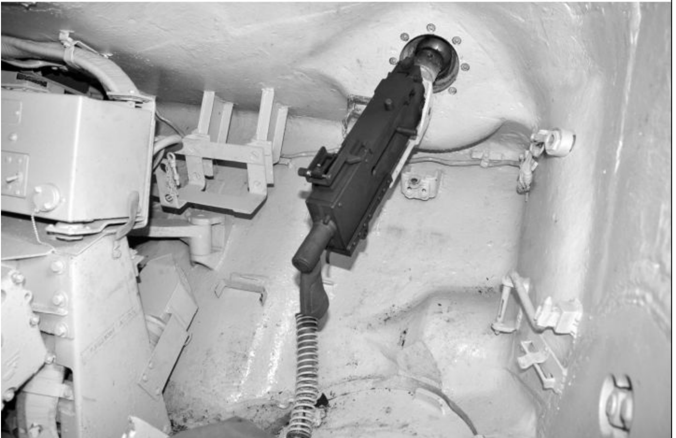
This picture shows the bow gunner's position in an M47 tank belonging to the Military Vehicle Technology Foundation. Unlike the bow gunner's position on the M46 series tank there was no duplicate driver's controls for the bow gunner on the M47 tank. Chris Hughes
