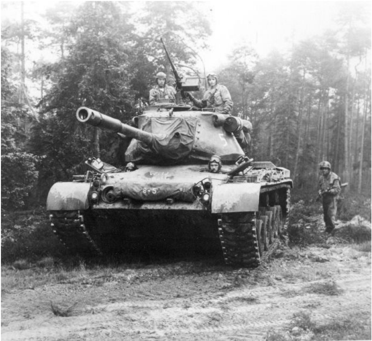
A series production M47 tank is pictured during a training exercise. Notice the small, rounded protrusions on either side of the upper frontal portion of the turret. They are the vision ports for the tank's stereoscopic rangefinder operated by the vehicle's gunner. Sadly, the stereoscopic rangefinder took a great deal of training to master and was not popular with crews as a result. Patton Museum
