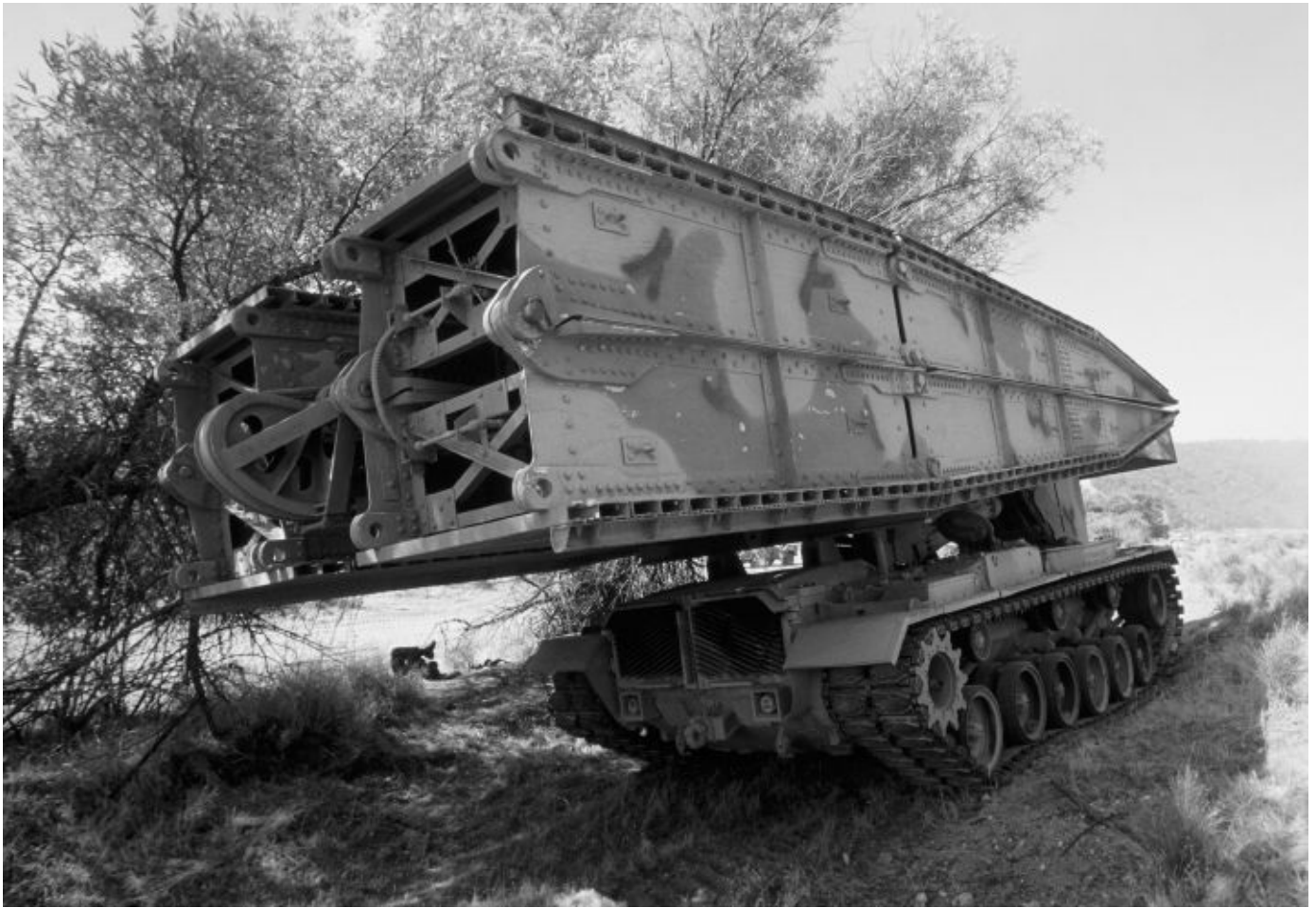
A rear view of an AVLB, based on the chassis of an M48A5 tank, which is evident from the boxlike M60 dry type air cleaner mounted on the right fender of the vehicle shown. Visible at the rear of the stowed bridge are the large hinge and associated cables that allow the two bridge sections to unfold and deploy. Michael Green
