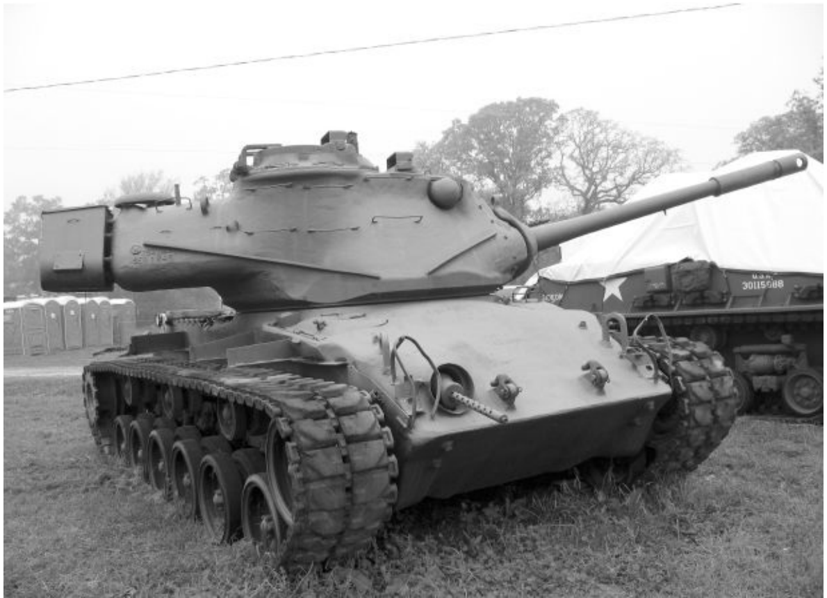
Belonging to a private American collector is this M47 tank that is missing its fenders. Notice the fender support brackets on the right side of the vehicle's hull. The rain gutters and the various handholds on the tank's turret mark it as a former West German Army vehicle. Michael Green
