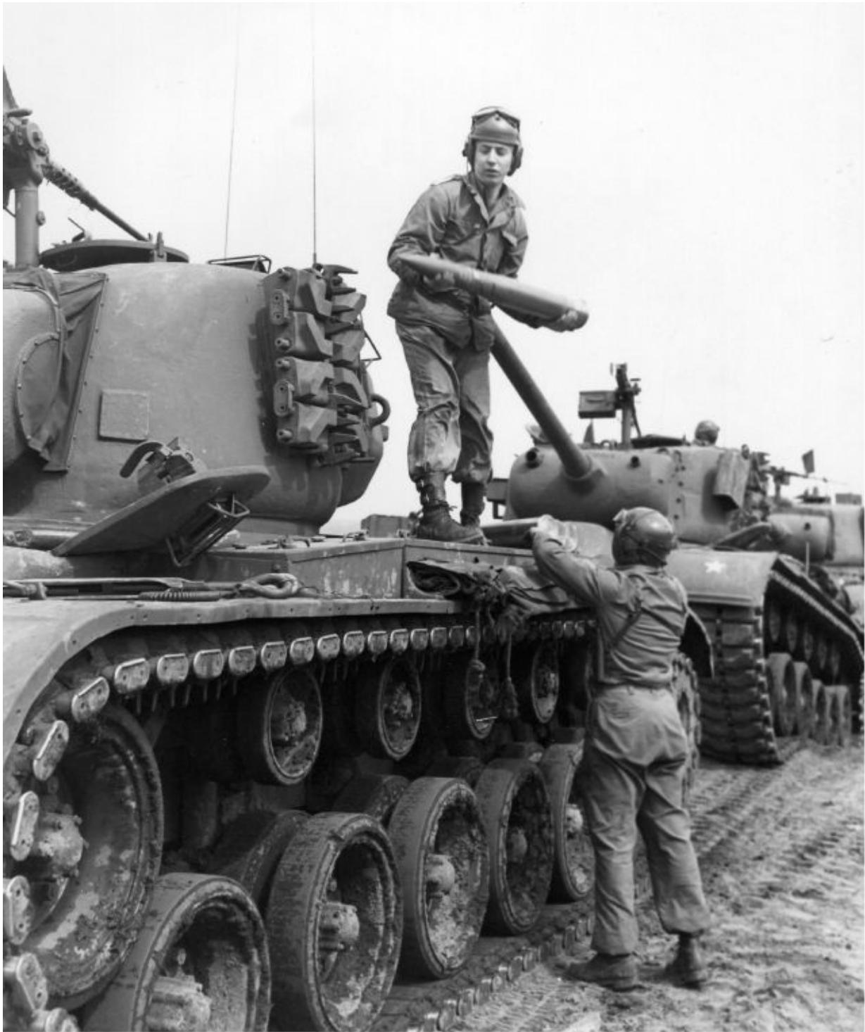
The crewmen of a postwar U.S. Army M26 tank are shown loading their vehicle with main gun ammunition. There was storage space in the M26 tank for 70 main gun rounds. The running gear of the vehicle consisted of 12 individually sprung dual road wheels (six per track) with 10 dual track return rollers (five per track). The tank rode on a torsion bar suspension system. Patton Museum
