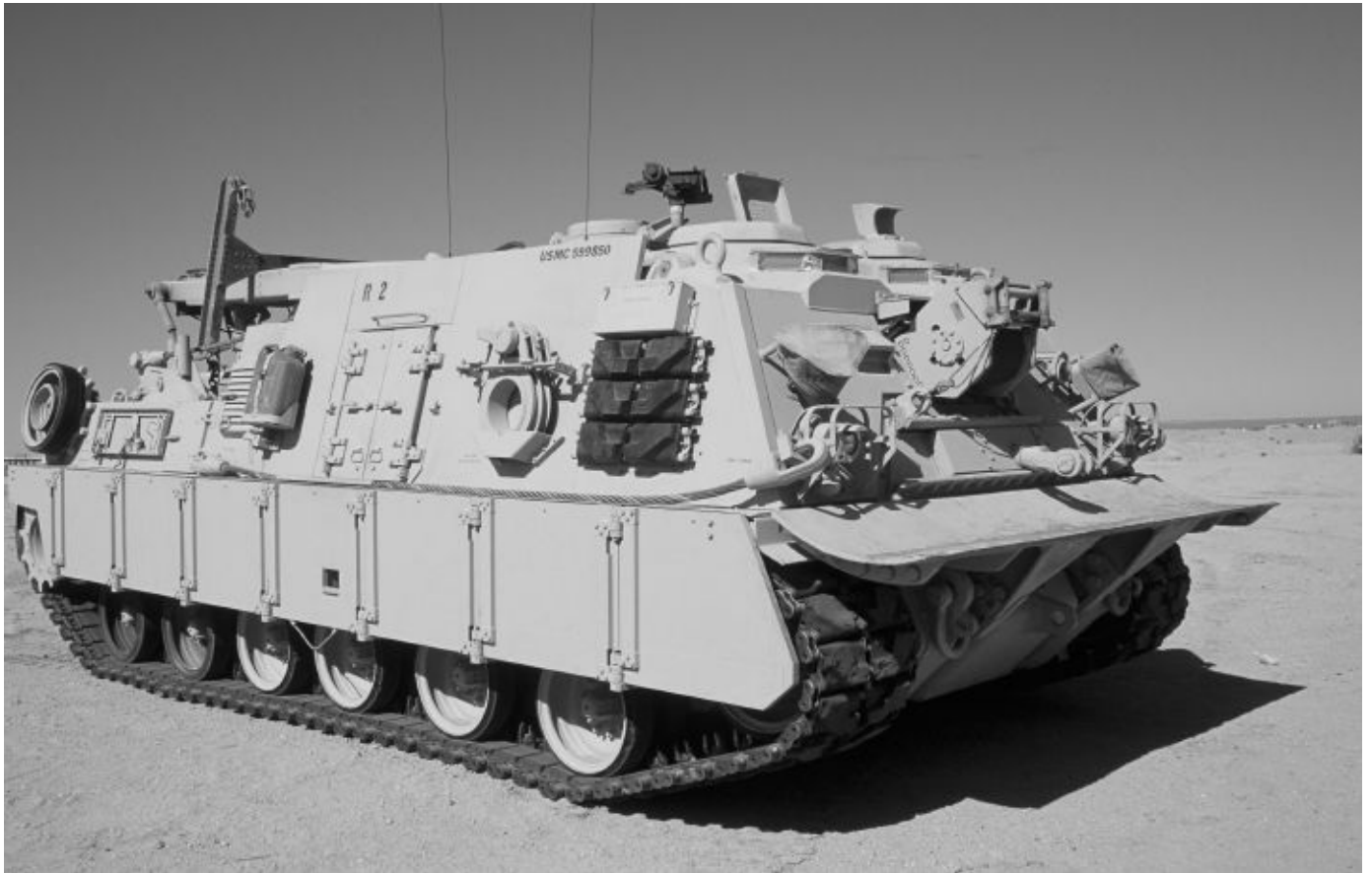
Awaiting its next mission is a U.S. Marine Corps M88A2 ARV, officially nicknamed the “Hercules.” This up-armored vehicles weighs 70 tons and is powered by an air-cooled, 12-cylinder Continental AVDS 1790-8CR engine producing over 1,000 horsepower. Notice the armored side skirts not seen on its predecessors. Michael Green
