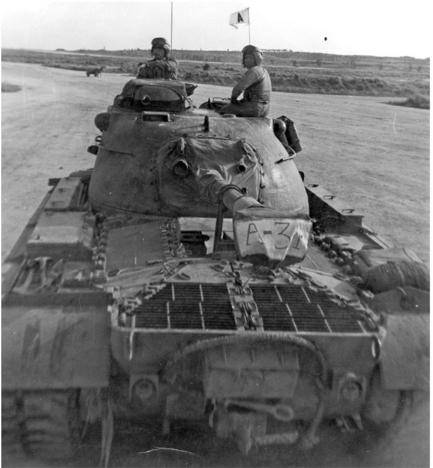
This photograph of a U.S. Marine Corps M48A1 tank with its turret reversed, shows the main gun mounted in the gun travel lock, which supports the gun (near the blast deflector) when the vehicle is traveling and not in a combat situation. There was no stabilizer system on the M48A1 tank's main gun. RC McInteer collection
