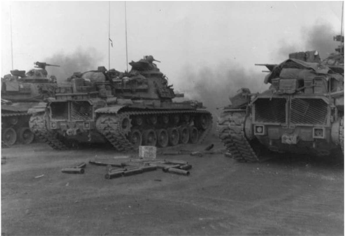
Here we see a number of late-production M48A3 (Mod B) tanks identified by their square brush guards around the rear tail lights on a firing range in South Vietnam. The rear engine decks of the vehicles shown are covered by a wide variety of gear. Patton Museum
