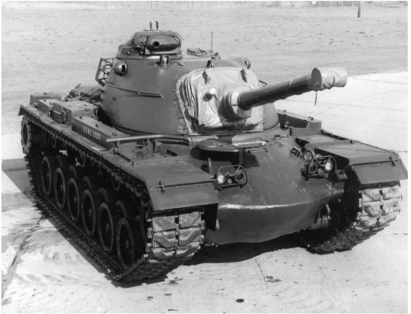
Pictured is a U.S. Marine Corps full-tracked combat tank, flame thrower M67A2, which was based on a modified M48A3 tank chassis. Notice the flattened brush guards on the front hull-mounted headlight clusters to allow for more depression of the flame tube. Marine Corps
