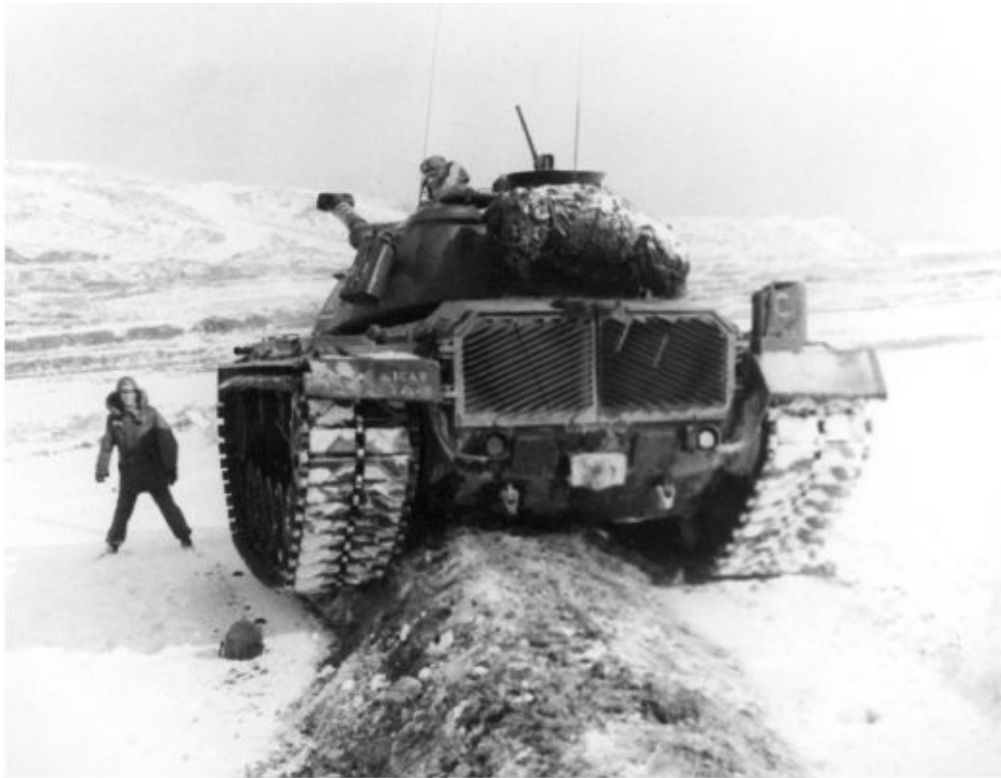
Pictured on the rear hull of this M48A2C tank that has managed to get itself stuck on a frozen rice paddy dike in South Korea are the two large louvered doors that deflect the engine exhaust gases horizontally, thereby improving the vehicles infrared signature. Patton Museum
