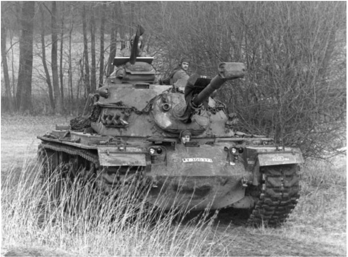
A West German Army M48A2 tank is pictured on a training exercise. Both the .50 caliber (12.7mm) machine gun mounted in the M1 cupola and the blast deflectors have been covered with canvas tarps to protect them from the elements. Patton Museum
