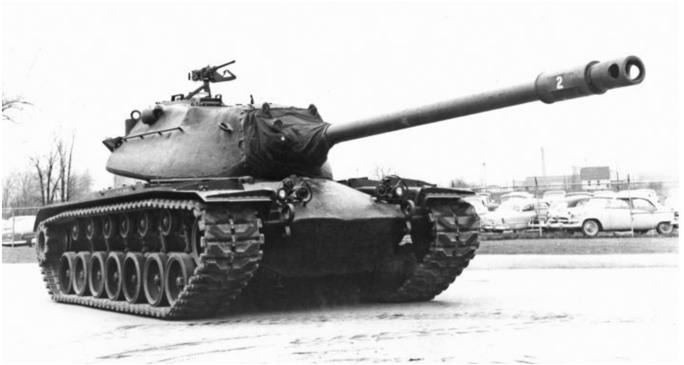
The second pilot of the 120mm gun tank T43E2 is shown. After further modifications it was designated the 120mm gun, full tracked, combat tank M103A1. The elliptically shaped cast homogenous armor (CHA) hull for the T48 tank was copied from the M103A1 tank as was the upper rear hull design. Patton Museum
