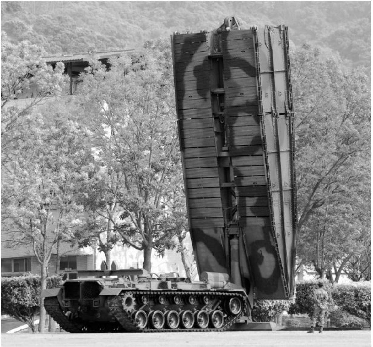
On display at a Taiwan Army open house day is this AVLB, based on the chassis of an M48A5 tank. The 63-foot span aluminum scissoring type-bridge is seen at its full deployed height before it is either deployed or retracted. The bridge sits upon a large I-beam arrangement that is visible over the rear engine deck of the vehicle shown. Mai Sen
