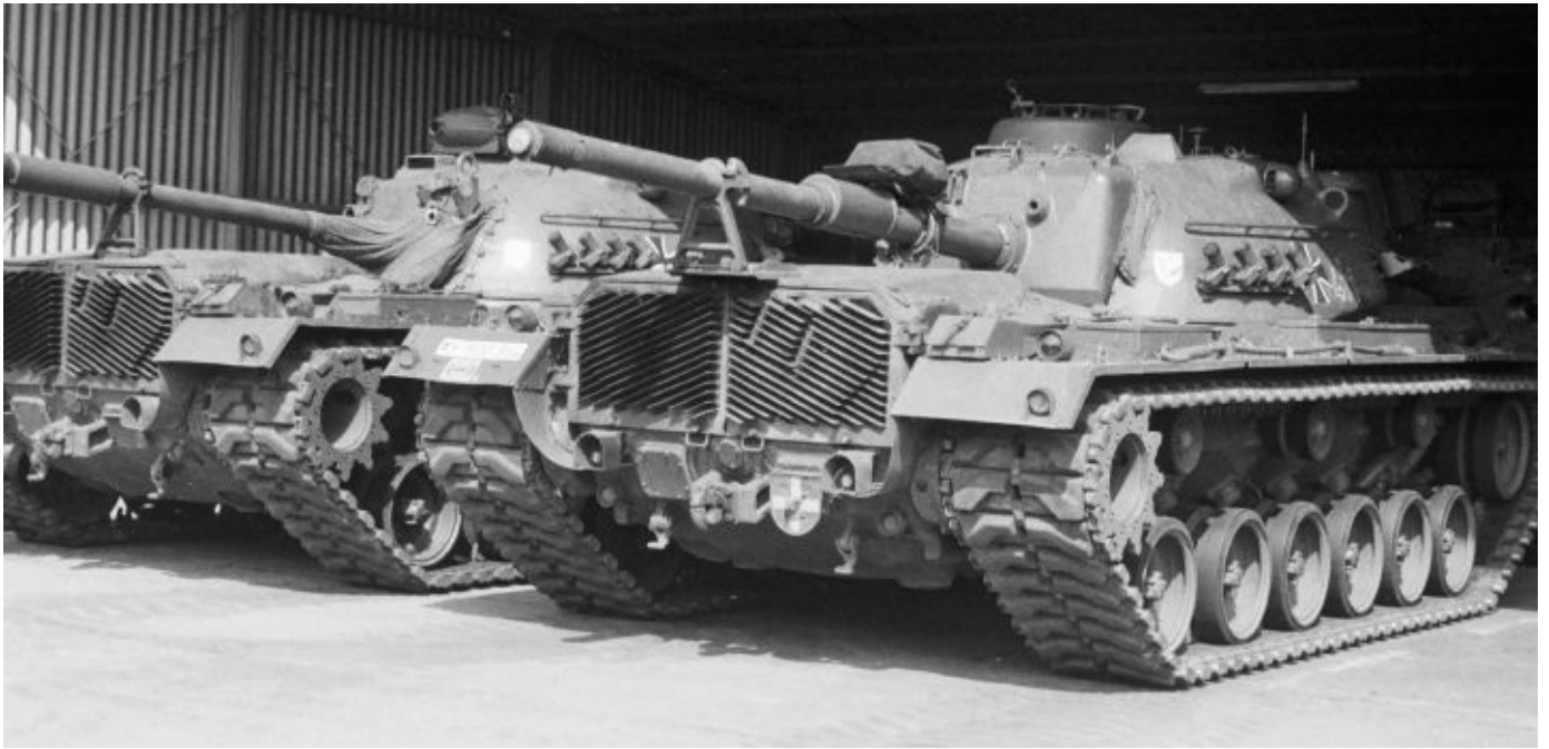
Pictured are two West German Army M48-series tanks in an open air shed. The one on the left is an M48A2C tank and one on the right is an upgraded M48A2GA2 tank. Clearly visible is the much larger and thicker gun shield on the M48A2GA2 tank and the mid-position bore evacuator of its 105mm main gun. Michael Green
