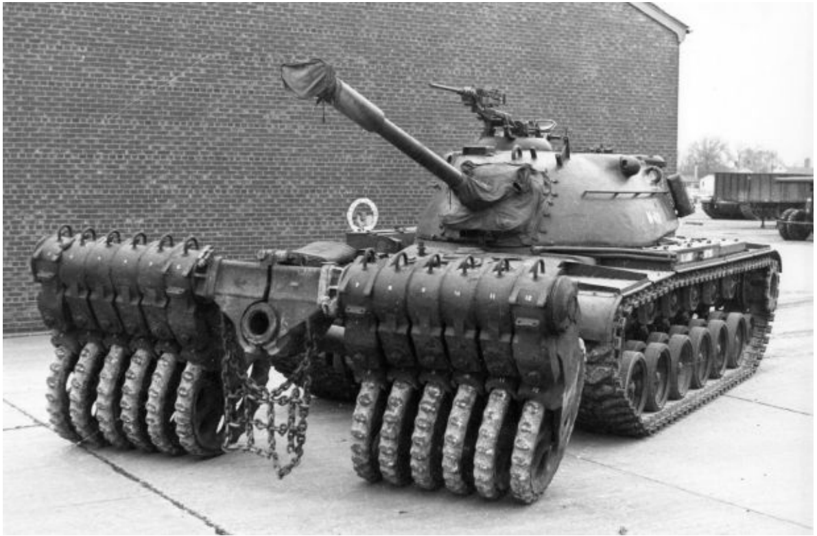
The first postwar roller type mine exploder tested by the U.S. Army was nicknamed the “Larruping Lou” and is seen here mounted on the front of an M48 tank. A boom assembly attached to the front of the tank’s hull guided twelve large steel discs to hopefully detonate any mines in the vehicle’s path. Patton Museum
