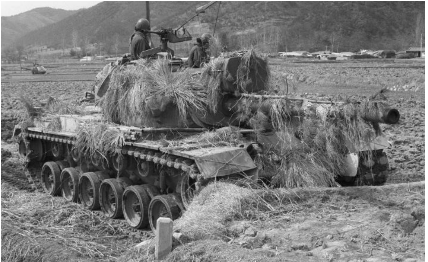
This picture is of a heavily camouflaged South Korean Army M48A5PI tank. Notice that the two 7.62mm M60D machine guns and their mounts are missing. In their place is a single .50 caliber (12.7mm) machine gun on a different type of mount. This vehicle is also fitted with a smoke grenade launcher system. DOD
