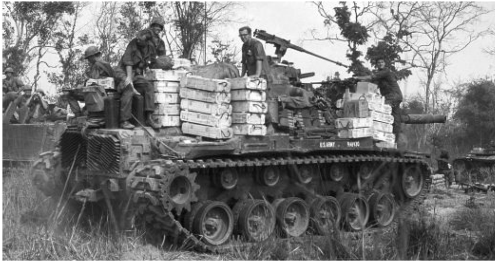
A U.S. Army M48A3 tank is shown in South Vietnam loaded down with boxes of main gun ammunition after a helicopter resupply mission. Main gun rounds were transported in fiber containers packed two to a 131 pound wooden crate. Kent Hillhouse
