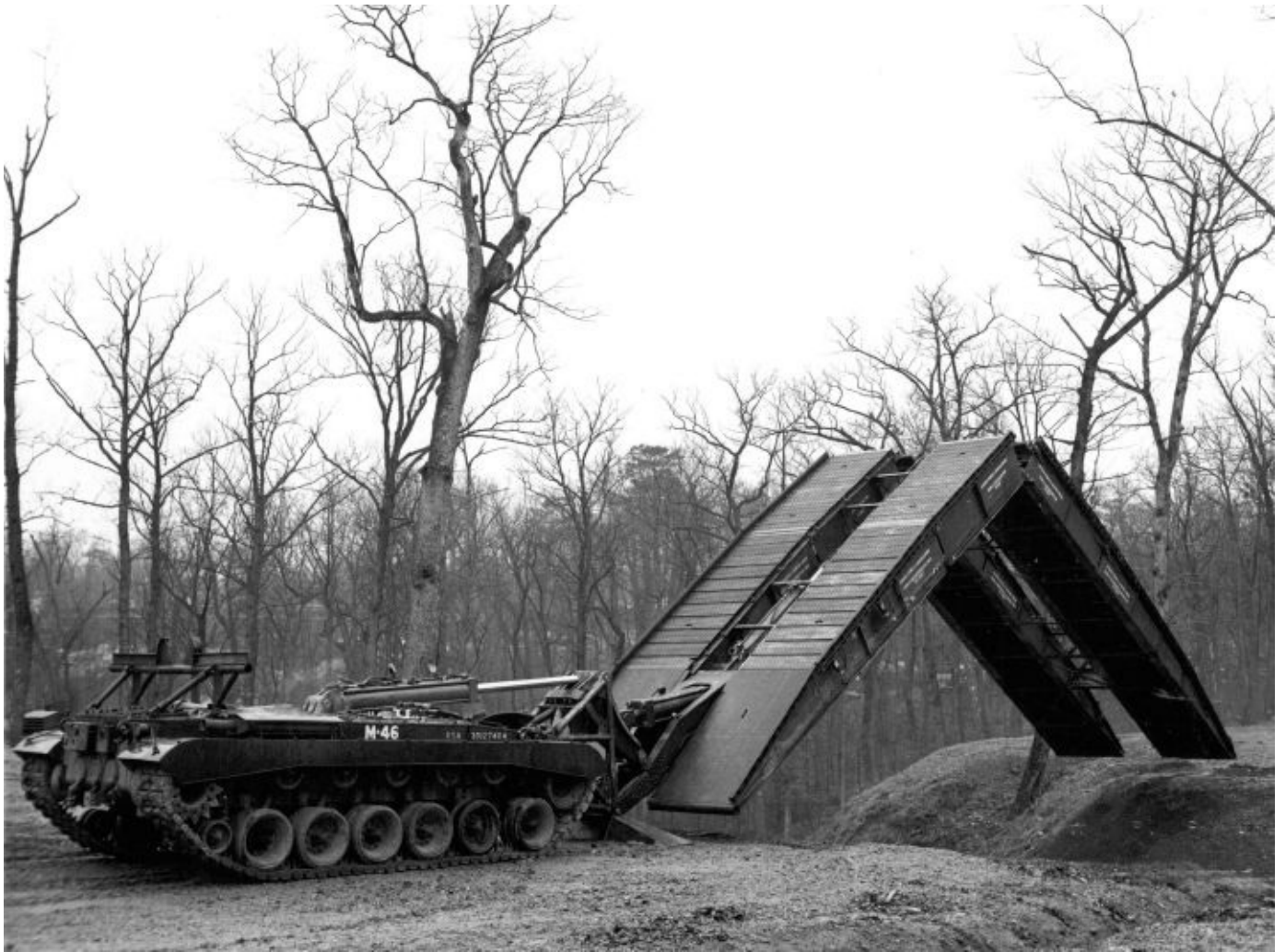
The U.S. Army's first postwar attempt to come with an armored vehicle launched bridge (AVLB) was based on the chassis of the M46 series tank as shown here. The prototype vehicle pictured is emplacing a 63-foot span aluminum (with steel reinforcement) scissoring-type bridge, which was launched and retrieved hydraulically. TACOM
