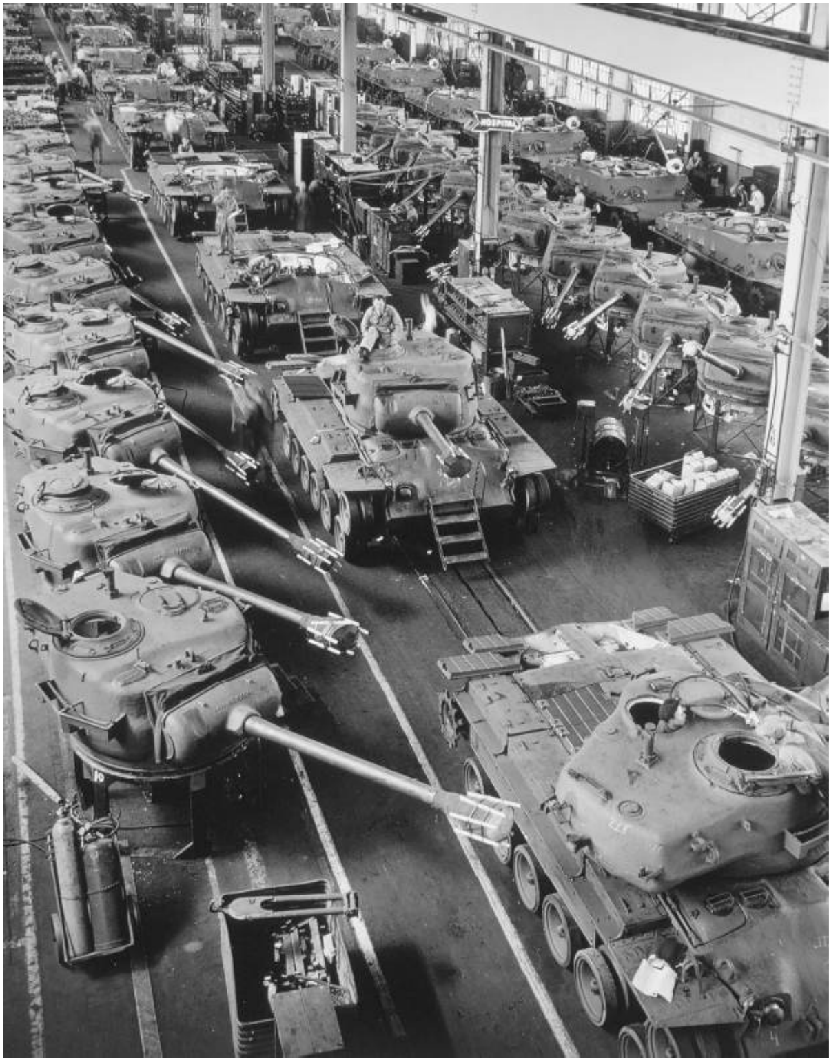
On the production line at the Fisher Tank Arsenal during the Second World War is a long line of M26 tanks. Production of what was then designated the T26E3 tank began at Fisher in November 1944. The initial order called for 250 T26E3 tanks to be built. Patton Museum
