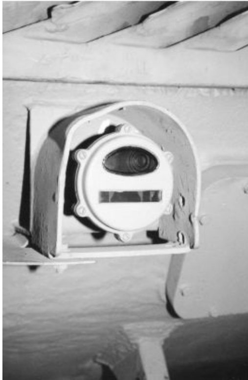
This is the original design for the brush guards around the rear taillights for the M48A2 through early production M48A3 (Mod B) tanks. Michael Green
