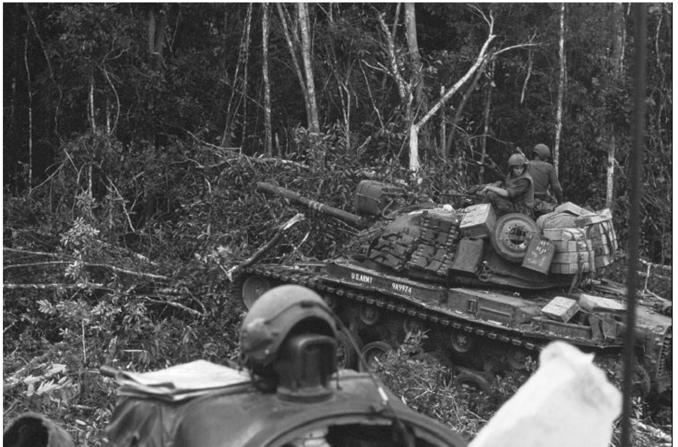
U.S. Army M48A3 tanks are shown jungle-busting in South Vietnam. This process caused a great deal of external damage to the vehicle as is seen with the missing fenders on the left side of the tank in the background. Unseen, is the wear and tear on the vehicle's suspension system and drive train. Kent Hillhouse
