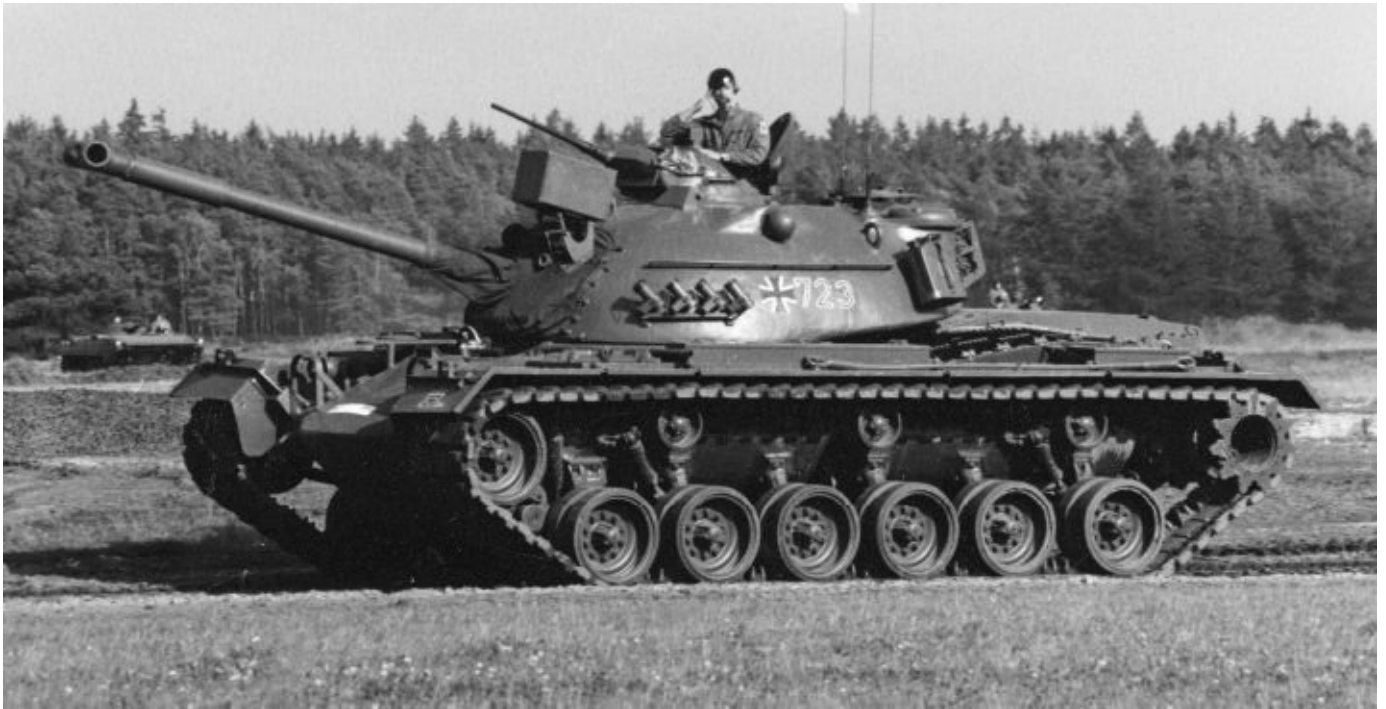
Forming part of the collection of the German Army tank museum located at Munster, Germany, is this operational M48A2C tank. The box-like device mounted on a bracket attached to the tank's turret is an IR/white light searchlight. Thomas Anderson
