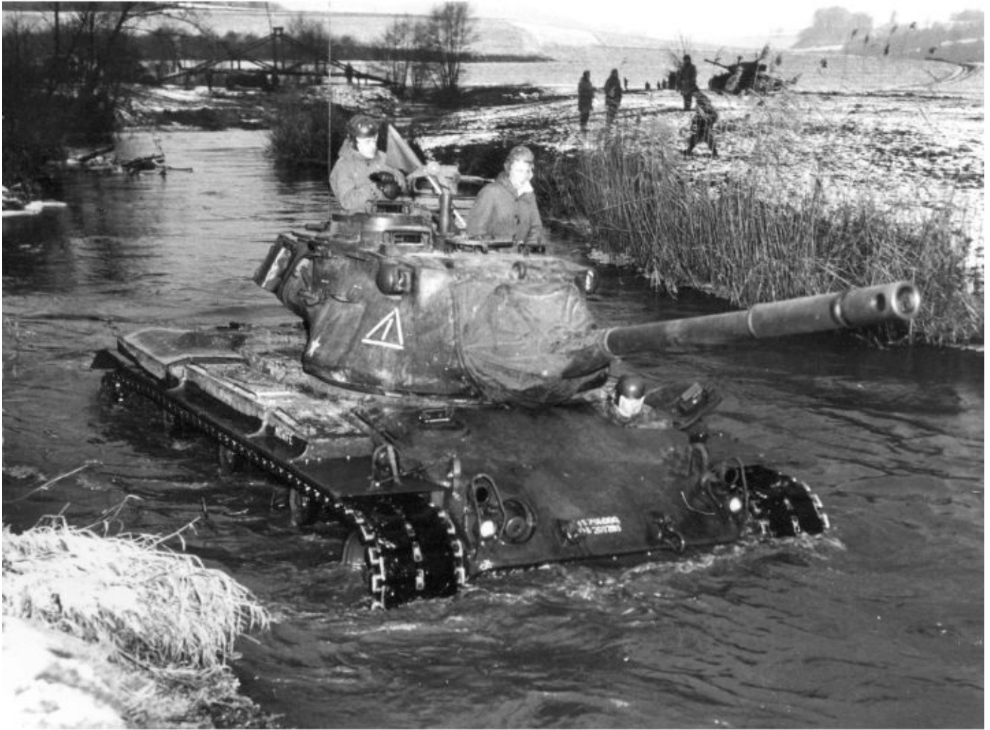
A U.S. Army M47 tank is shown conducting a fording test in the Fulda River near Fulda, Germany on December 11, 1953. All postwar U.S. Army tanks were required to ford, without any prior preparation, a 48 inch deep (1.22m) water obstacle. Patton Museum
