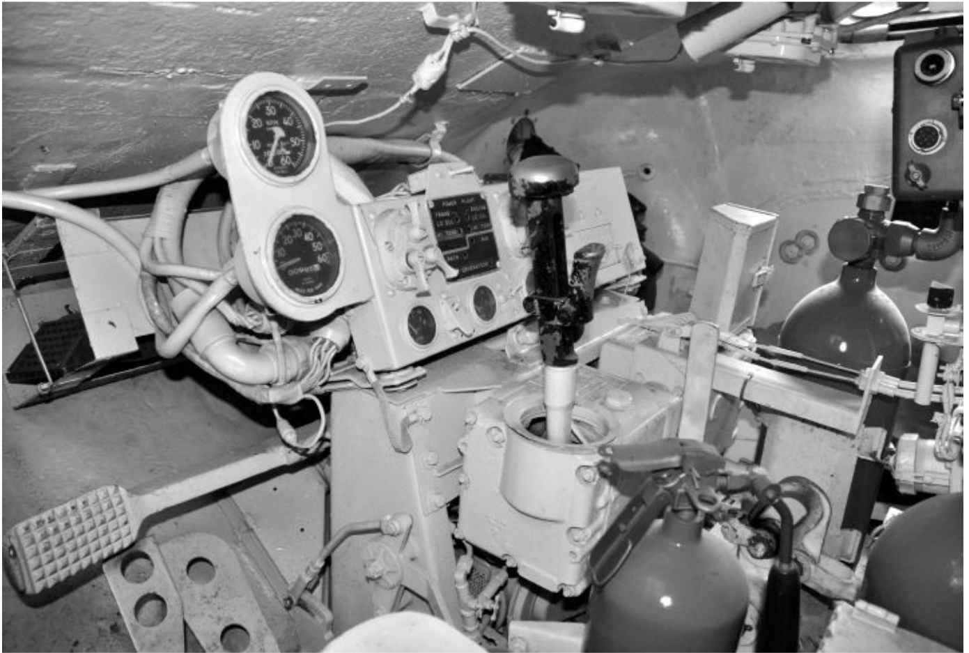
This picture shows a view of the driver's position on a late production M47 tank. Notice the numerous fire extinguishers stored in the front hull of the vehicle. On a level road the driver could sustain a speed of 30 miles per hour (48.3kmh). Chris Hughes
