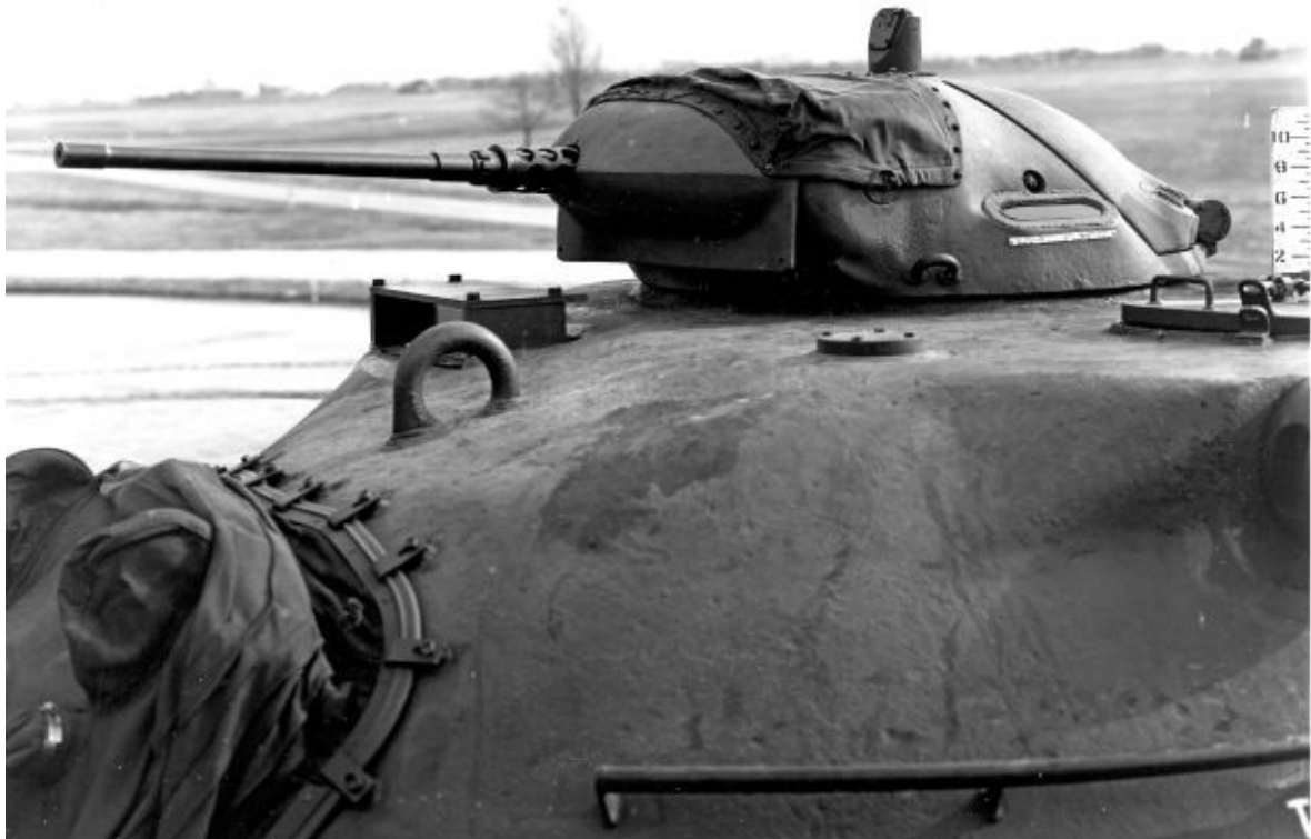
U.S. Army unhappiness with the Chrysler-designed tank commander cupola on the T48 and M48 tanks led to the adoption of a new enclosed tank commander cupola seen here on a T48 tank armed with an internally-mounted .50 caliber (12.7mm) machine gun and eventually designated the M1 cupola. Tanks equipped with the new cupola were designated the M48A1 tank. Patton Museum
