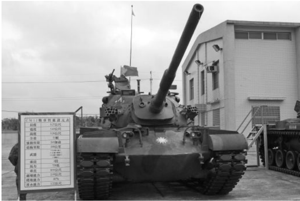
This picture taken during an open house day for the public at a Taiwan Army base shows a CM12 tank, which features the turret from the CM11 Brave Tiger mounted on the upgraded chassis of an M48A1 tank fitted with a diesel engine. Notice the M60 type headlight cluster and brush guards. Mai Sen
