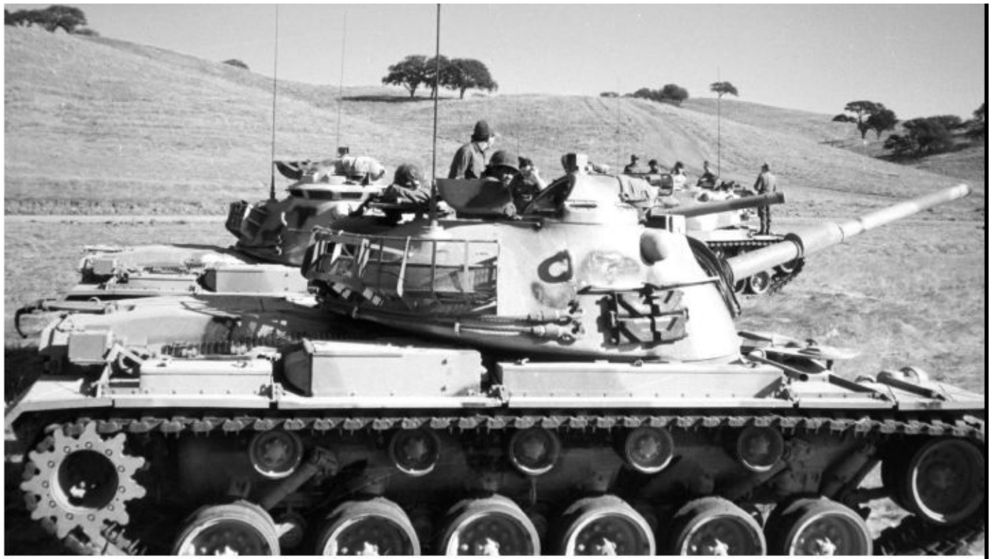
Pictured are California National Guard M48A5 tanks during a training exercise. Notice the vehicle in the foreground has the original M1 cupola but no G305 turret riser, which meant it would have started life as an M48A1 tank before being converted into an M48A5 tank. Michael Green
