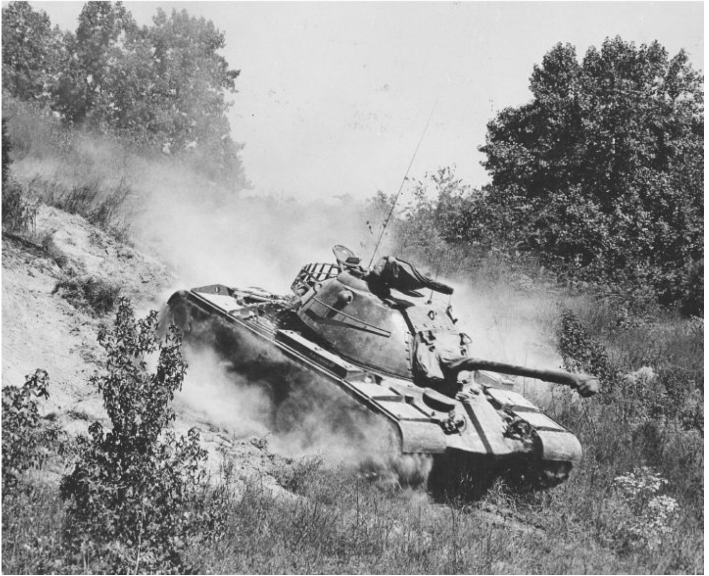
A T48 tank races down a steep hill. Mobility testing of the T48 tank and the constant throwing of tracks led the U.S. Army to decide to add a track tension idler to the later production versions of the vehicle as was seen on the M46, M46A1 and M47 tanks. The T48 rode on a torsion bar suspension system. Patton Museum
