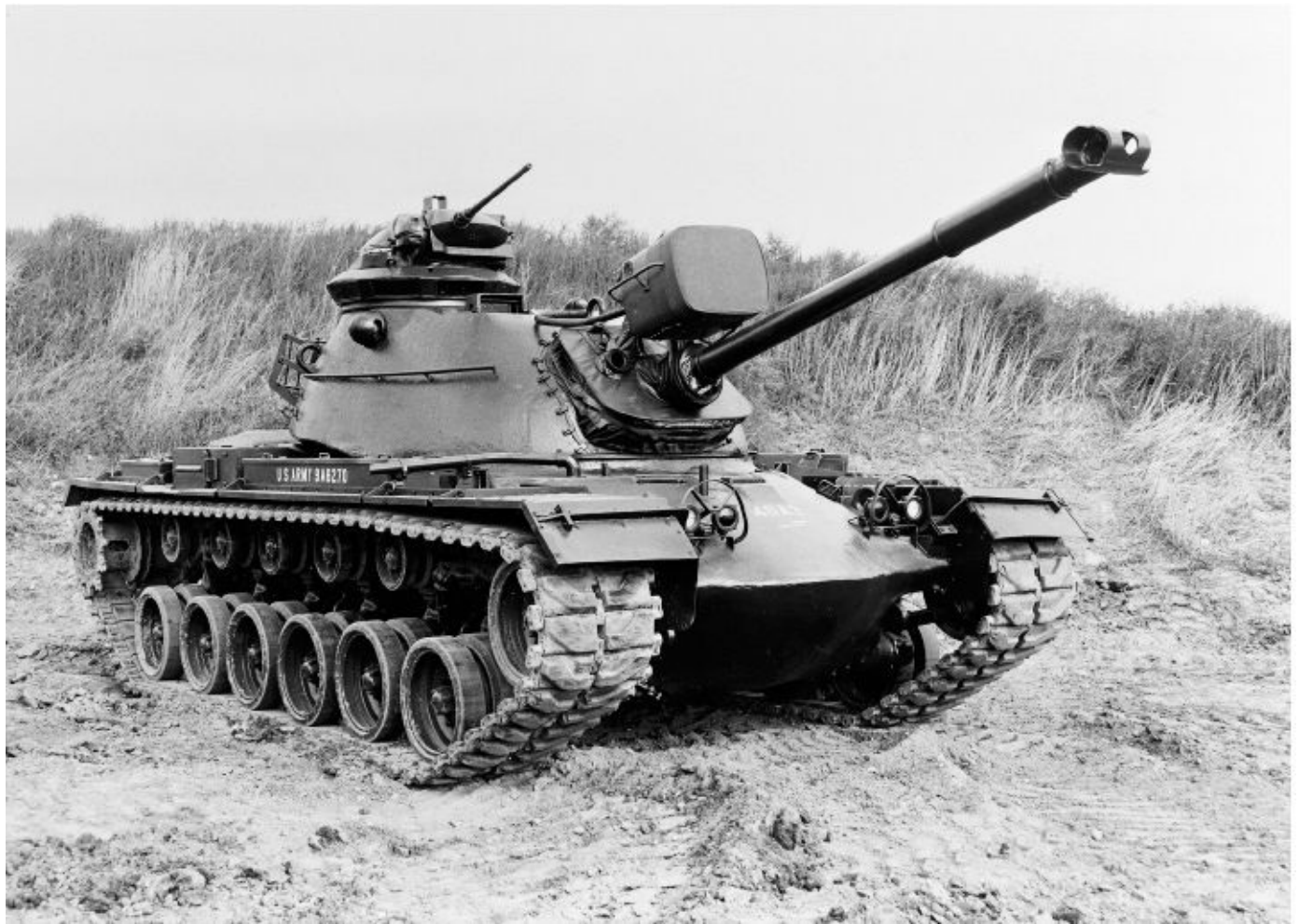
A factory fresh early-production M48A3 (Mod B) poses for the company photographer. Notice the 2.2 kilowatt Xenon white light/infrared searchlight mounted just above the gun shield. The spacer ring under the M1 cupola was designated as the G305 turret riser. Patton Museum
