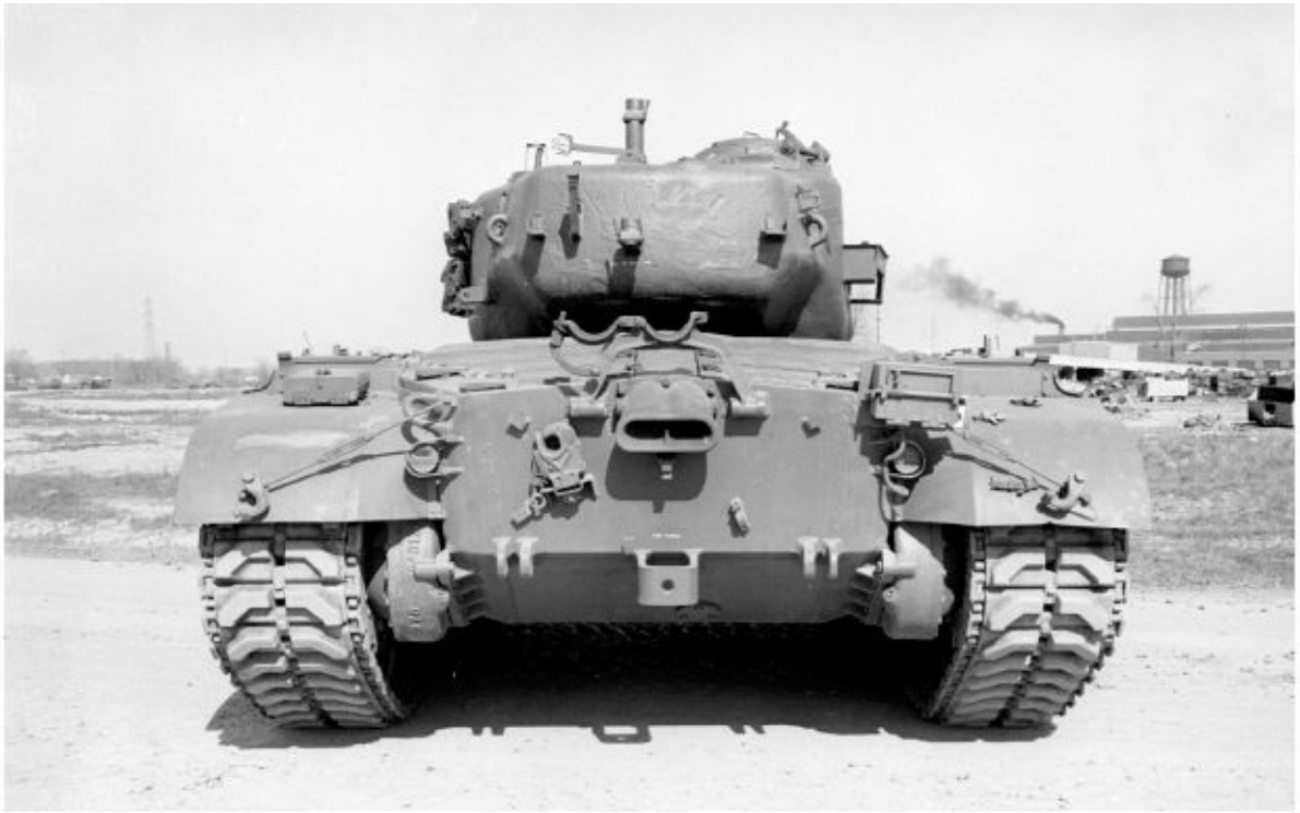
This view of an M26 tank shows the engine exhaust muffler on the upper rear portion of the rear engine compartment plate. Notice the turnbuckles and rods holding up the rounded rear fender extensions on this vehicle, which was a postwar addition to the vehicle. These turnbuckles also appeared on the front of the vehicle. TACOM
