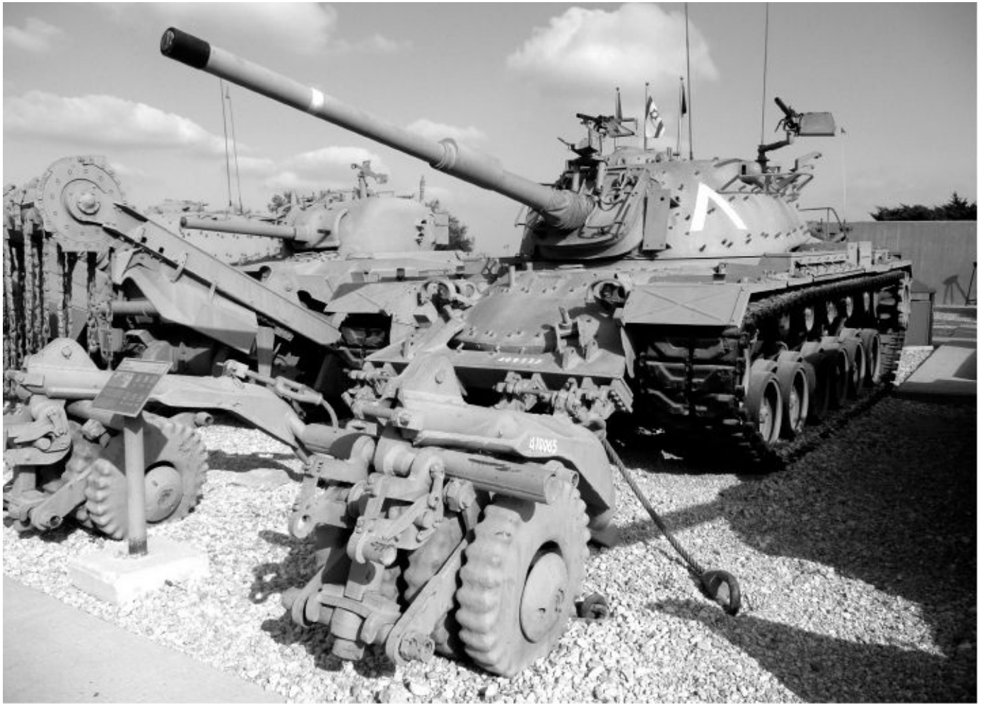
Mounted on the front of this Israeli Magach 3 is an Israeli copy of a Soviet Army tank mounted mine roller, which is on display at the Israeli Armored Corps Memorial Site and Museum. Visible on the vehicle hull and turret are attachment points for Blazer explosive reactive armor tiles. Vladimir Yakubov
