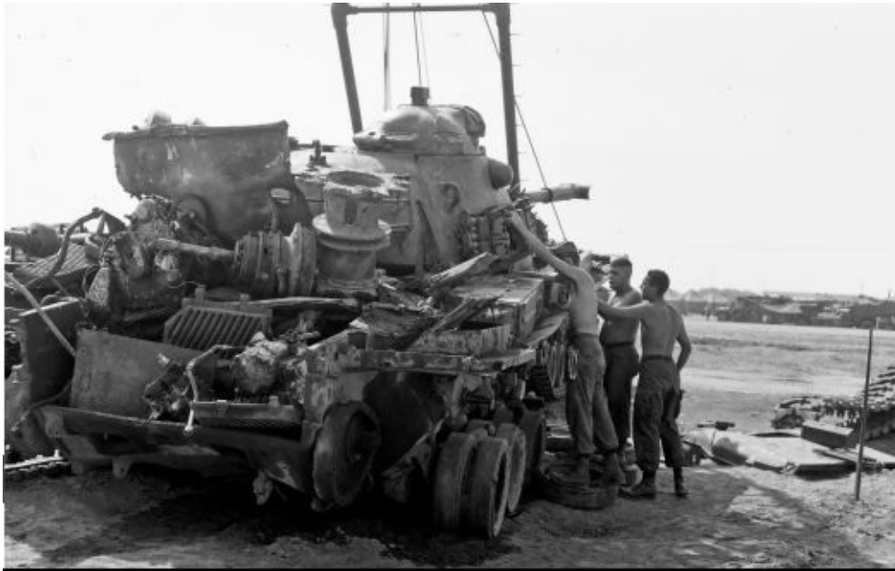
This picture illustrates the damage a large improvised mine could do to an early-production U.S. Army M48A3 tank in South Vietnam. The improvised mines employed by the enemy included recovered dud American artillery shells and aerial-dropped bombs of varying sizes. Patton Museum
