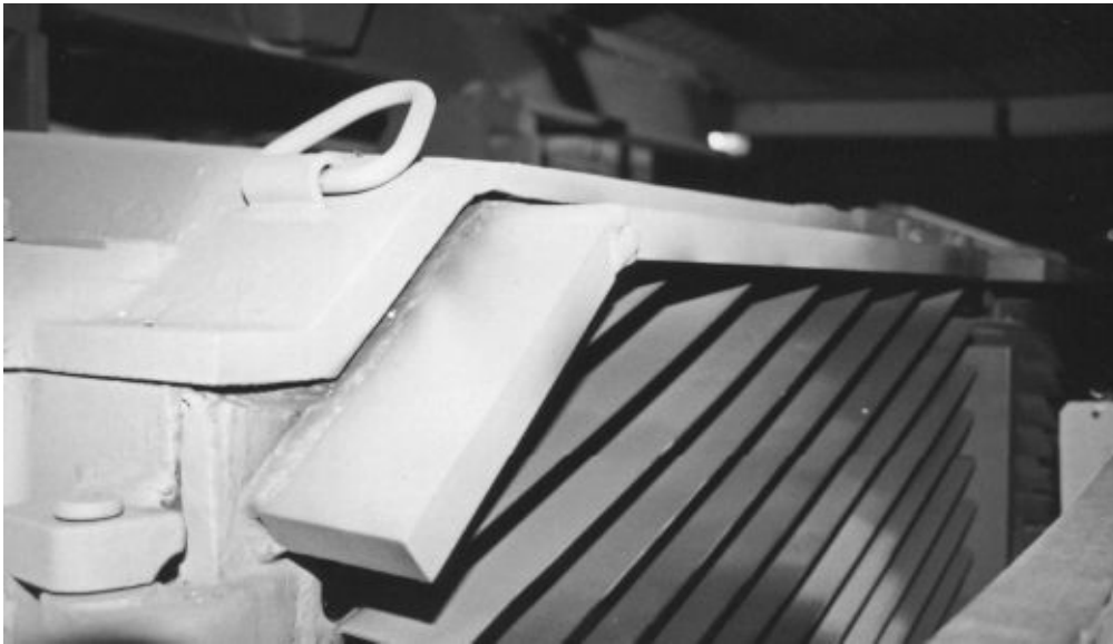
The thick welded-on protruding steel bars that was affixed just above the two large steel louvered doors at the rear hull of late-production M48A3 (Mod B) tank is shown here. Michael Green
