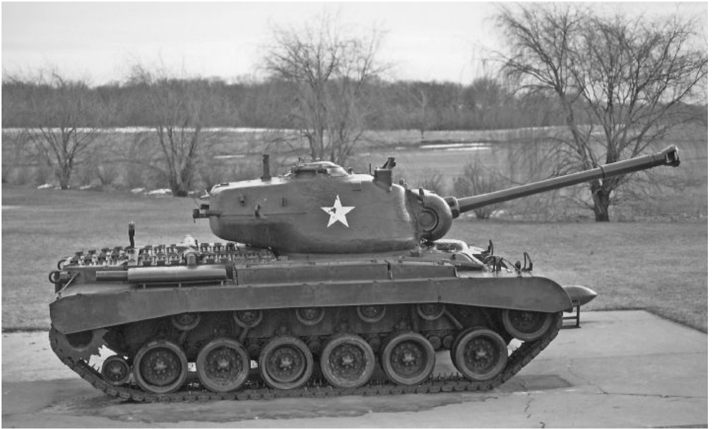
Belonging to the former Patton Museum of Armor and Cavalry is this early-production M46 tank, which is minus the sheet metal muffler shields. The turret of the M46 tank was traversed either manually or with an electric-hydraulic system. With the powered traverse system the turret on the M46 tank could be turned 360 degrees in 15 seconds. Dean and Nancy Kleffman
