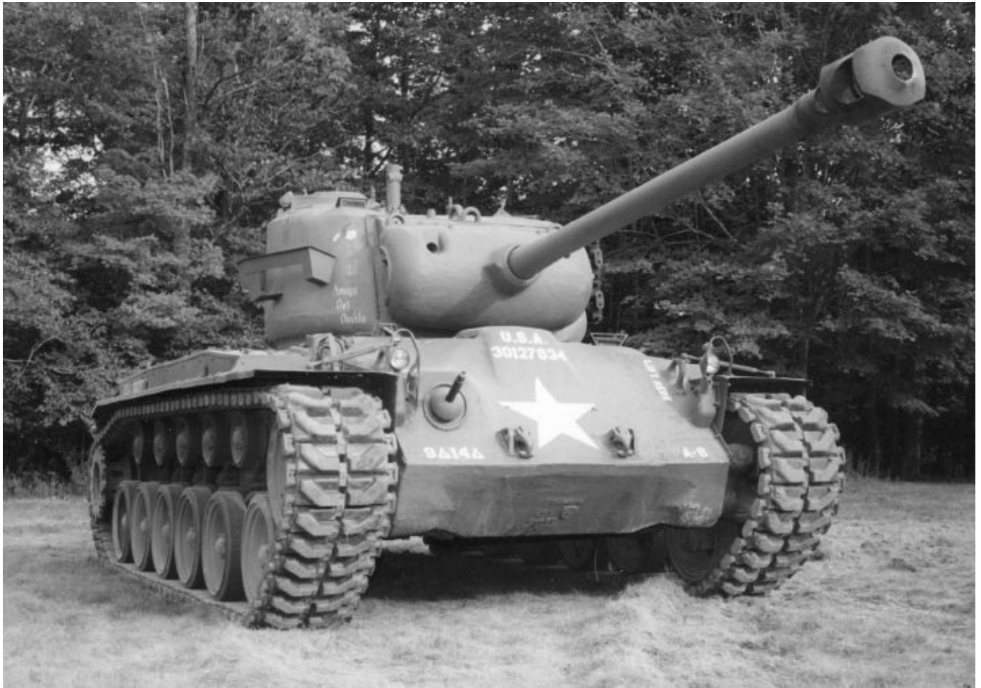
The U.S. Army's answer to late-war German Panther and Tiger tanks was the M26 heavy tank. Unlike the thinly armored and under-gunned M4 series medium tanks, the new tank boasted fairly thick armor and a high-performance, tank-killing M3 90mm main gun. The restored vehicle pictured belongs to a private collector. Bob Fleming
