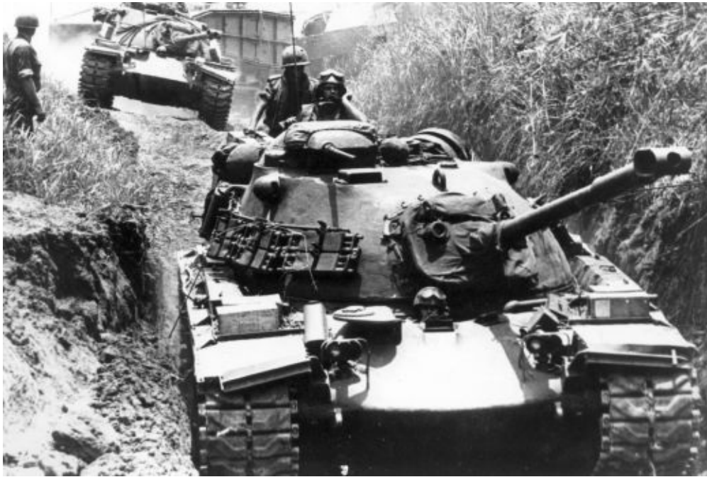
Here we see two U.S. Army M48A3 tanks in South Vietnam without the Mod B turret risers but with late production Mod B front-hull mounted headlight clusters with squared brush guards. Notice that the front hull mounted fender extensions on both tanks have either been cut off or torn off due to dense vegetation. Patton Museum
