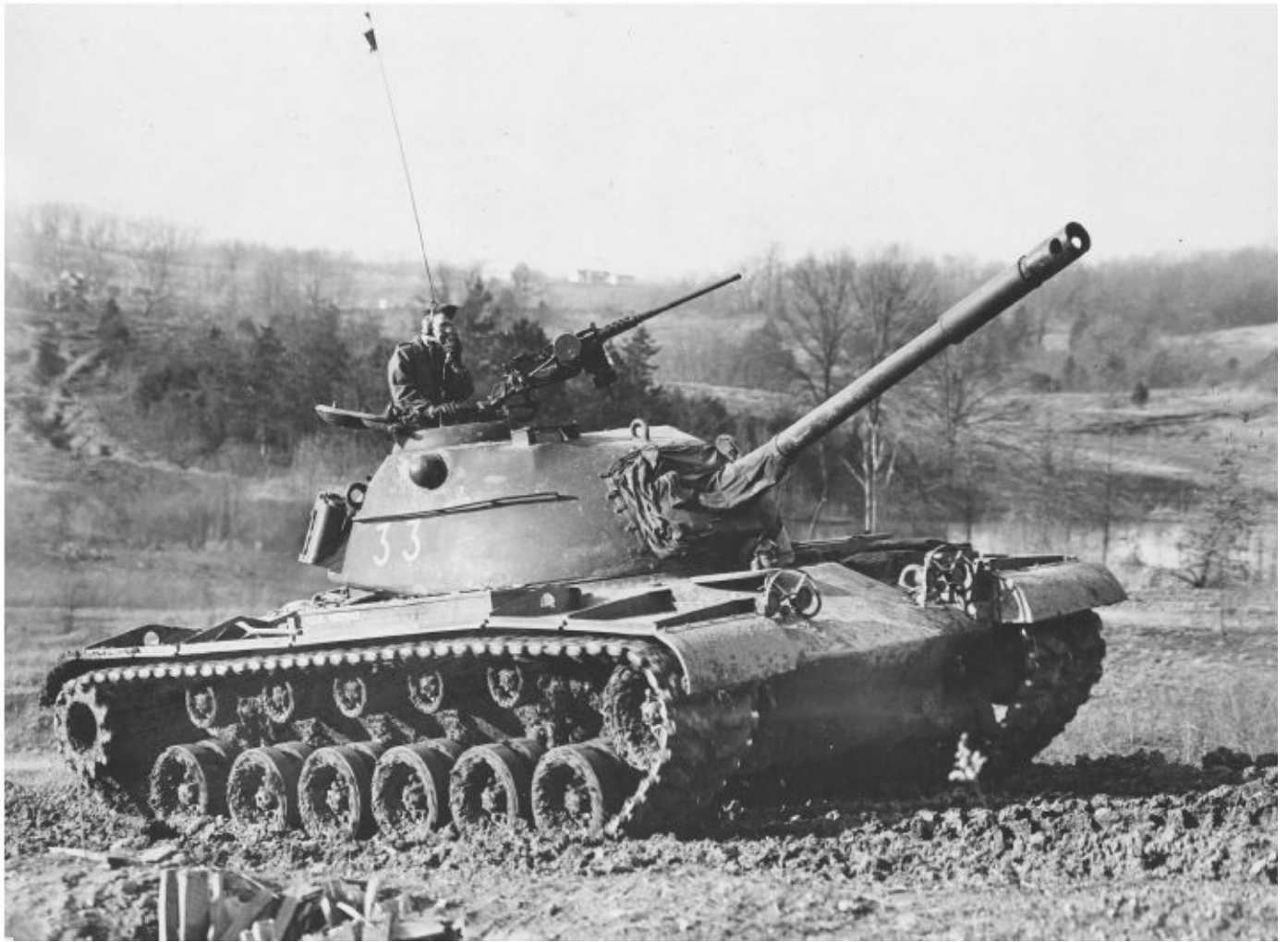
An early model 90mm gun tank T48 is pictured undergoing mobility testing at Fort Knox, Kentucky. Early model T48 tanks can be identified by their cylindrical blast deflector and the lack of track tension idlers located between the last road wheels and the rear-mounted drive sprockets. Patton Museum
