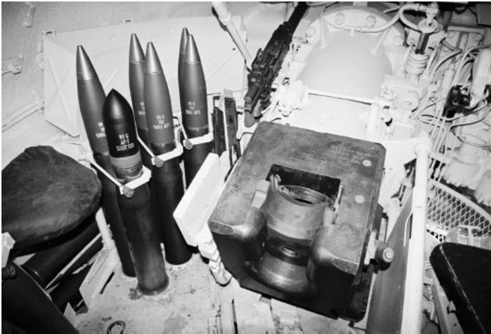
Looking down through the tank commander's cupola on an M26A1 tank, the breech of the M3A1 90mm main gun as well as the loader's ready rounds are visible. The M3A1 90mm main gun in the M26A1 tank was an improved version of the M3 90mm main gun mounted in the M26 tank. Michael Green
