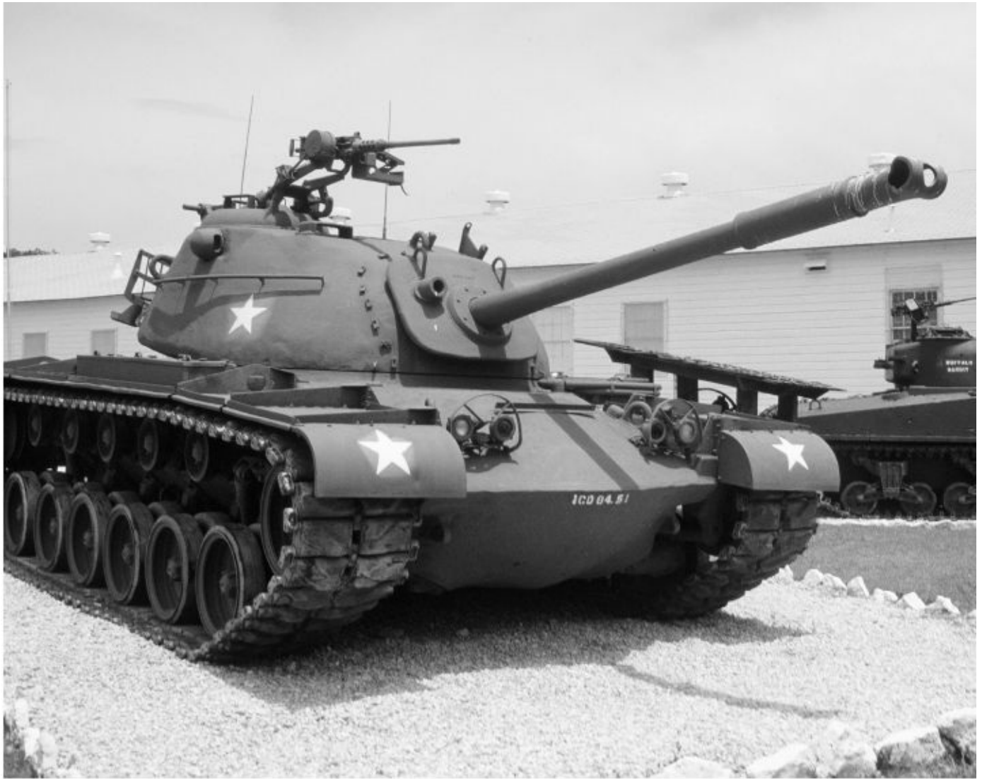
The T48 tank became the 90mm gun tank M48 in April 1953. Pictured at Fort Hood, Texas is an M48 tank. The original cylindrical blast deflector was eventually replaced with the T-shaped blast deflector seen here. This vehicle also has the Chrysler-designed low profile tank commander cupola seen on all the T48 and M48 tanks. Michael Green
