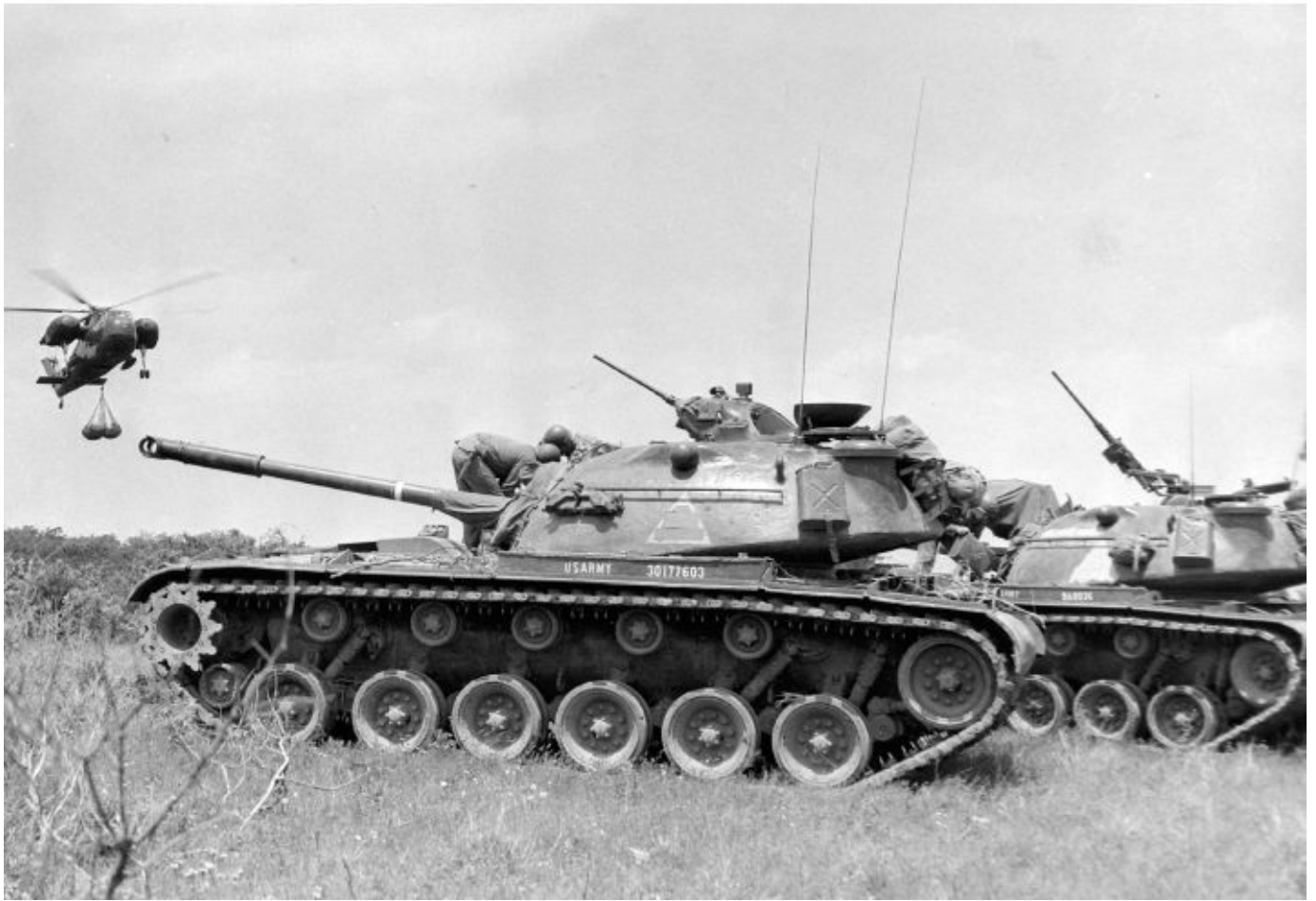
This picture taken during a field exercise shows an M48A1 tank in the foreground and an M48 tank in the background. The M48A1 tank was provided with an opened-topped enclosed turret bustle rack, which normally contained items like the crew's sleeping bags and spare uniforms. Patton Museum
