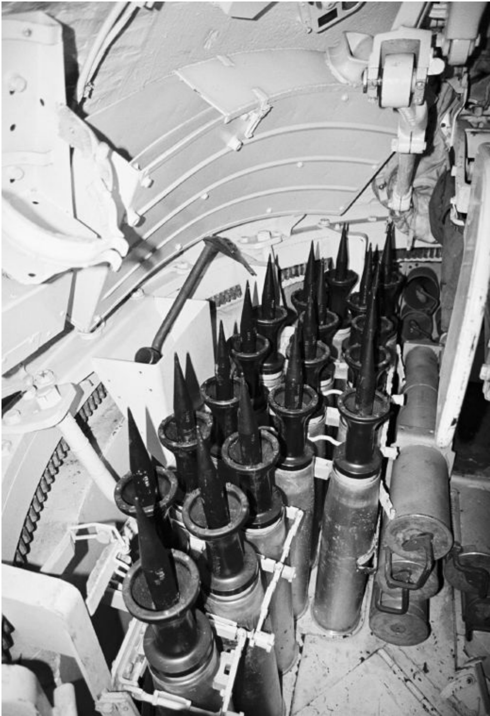
Looking forward from the loader's seat on an IDF Magach 3 is part of the main gun ammunition storage arrangement, in this case loaded with armor piercing rounds. On the interior turret wall just above the stored main gun rounds is a large white-painted metal bin that contains the ammunition supply for the tank's 7.62mm coaxial machine gun. Michael Green
