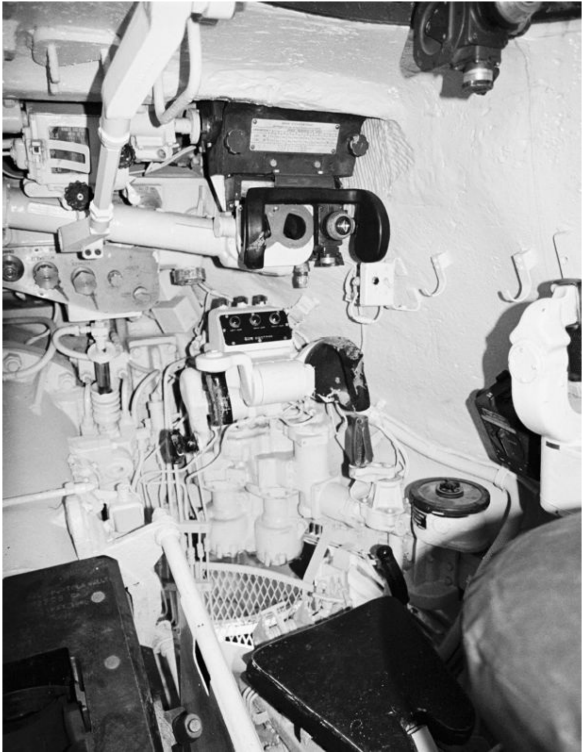
From just behind the M3A1 90mm main gun in a M26A1 tank can be seen the gunner's position. A portion of the tank commander's seat can be seen in the right foreground of the picture. Michael Green
