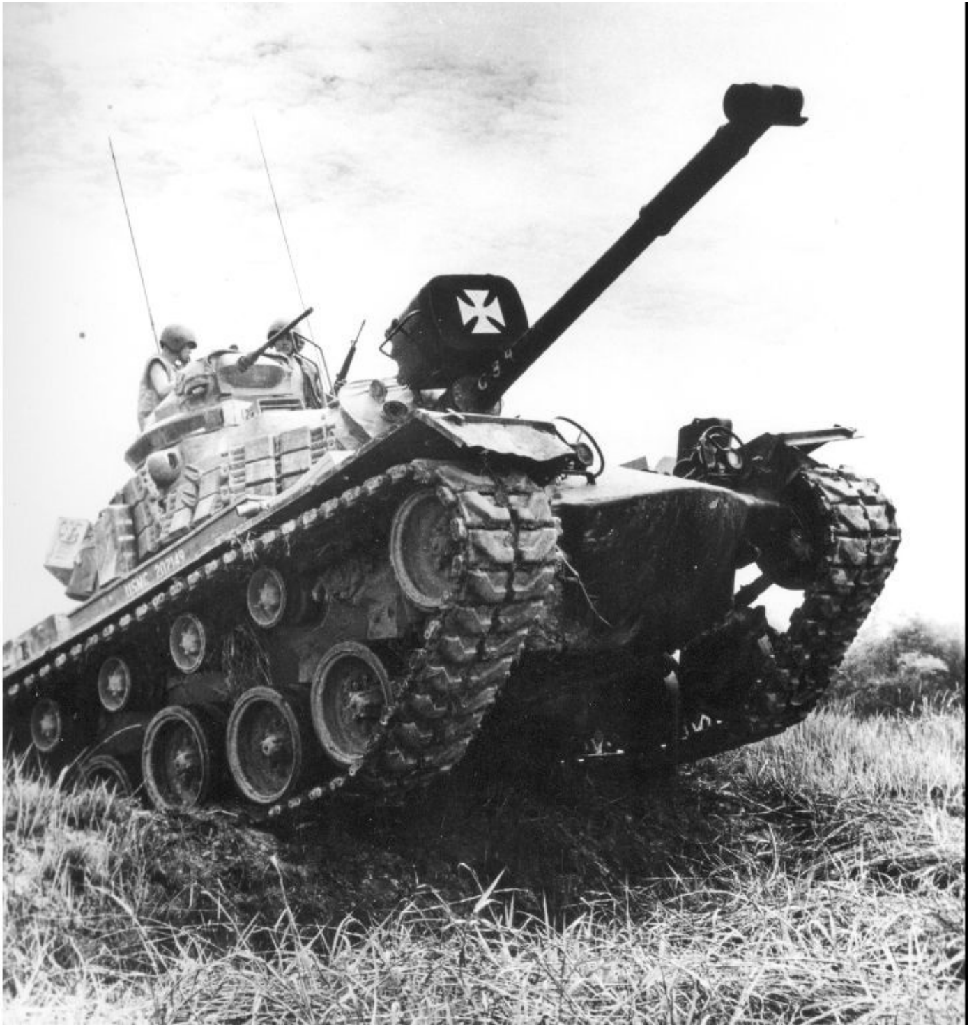
A U.S. Marine Corps early-production M48A3 (Mod B) tank crosses over a rice paddy dike somewhere in South Vietnam. The large wheel at the front of the tank's suspension system is one of two front hull compensating idlers that helped to eliminate slack in the vehicle's two sets of tracks under dynamic conditions. Slack is the stretching of a tank's tracks, which can then disengage themselves from the vehicle's suspension system if not corrected for. Patton Museum
