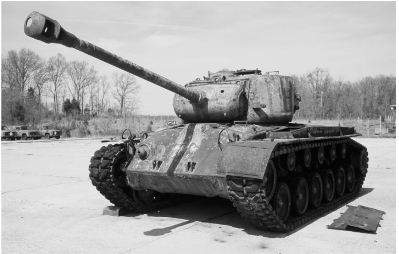
Belonging to the former Patton Museum of Armor and Cavalry is this unrestored M26 tank that came off a U.S. Air Force firing range. A distinguishing external feature of the M26 was the large and squat CHA turret that set well forward on the hull as seen in this photograph. Michael Green
