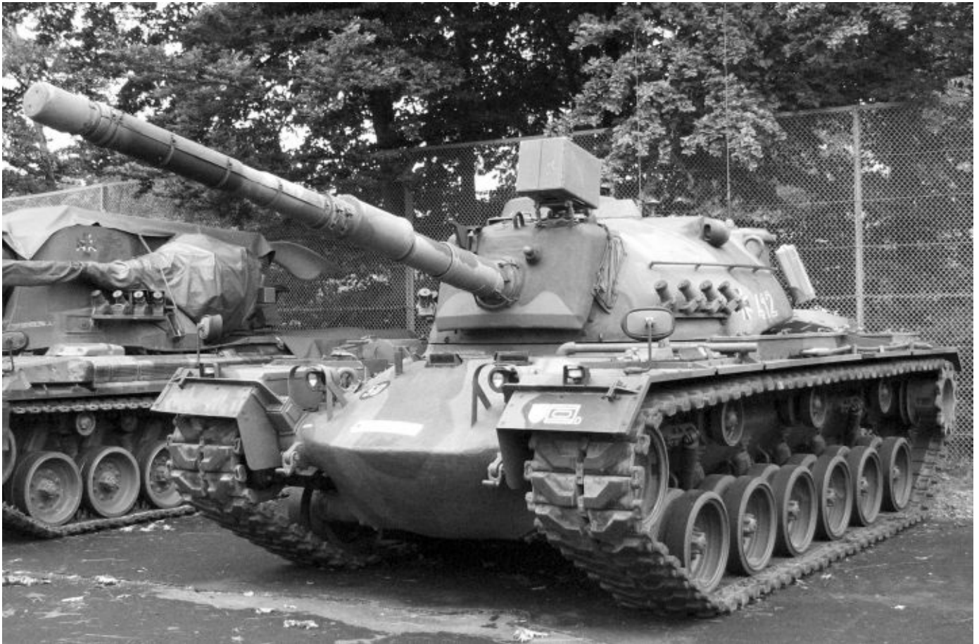
On display at the German Army tank museum is what the West German Army referred to as the M48A2GA2, which was an upgraded M48A2C tank armed with a 105mm gun. It also featured a new square gun shield, as well as a new vehicle commander's cupola. Frank Schulz
