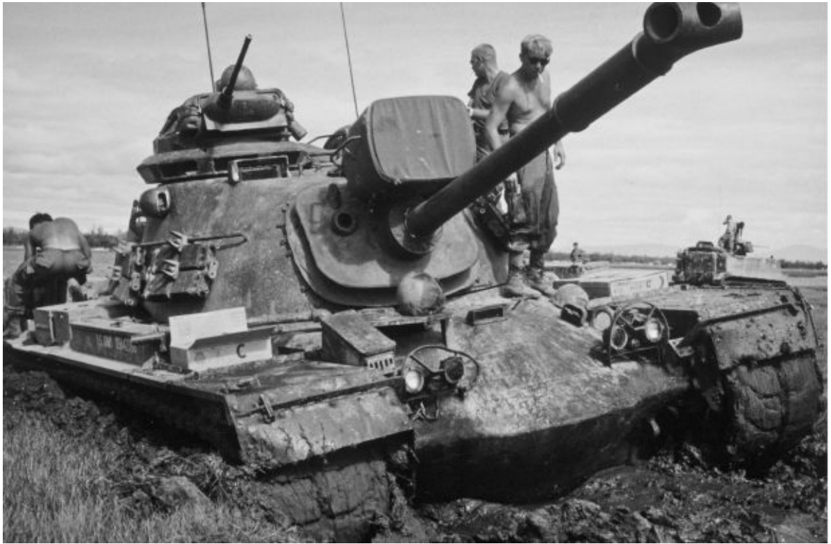
Here we see an early production U.S. Army M48A3 (Mod) B tank with the G305 turret riser. This particular vehicle has become immobilized in a South Vietnamese rice field. Tank drivers are taught when confronted with a marshy area to keep their momentum up, follow a straight line, and avoid spinning the tracks. Patton Museum
