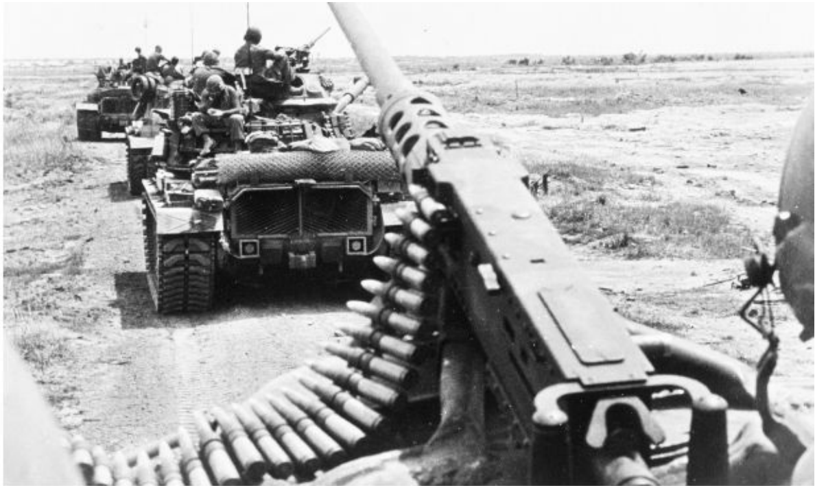
This picture was taken from the top of an U.S. Army M48A3 (Mod B) tank in South Vietnam. The tank in the foreground carries a large bundle of cyclone fencing material wrapped around a number of engineering stakes. The box-like brush guard around the rear tail lights of the tank in the foreground mark it as a late-production M48A3 (Mod B) tank. Patton Museum
