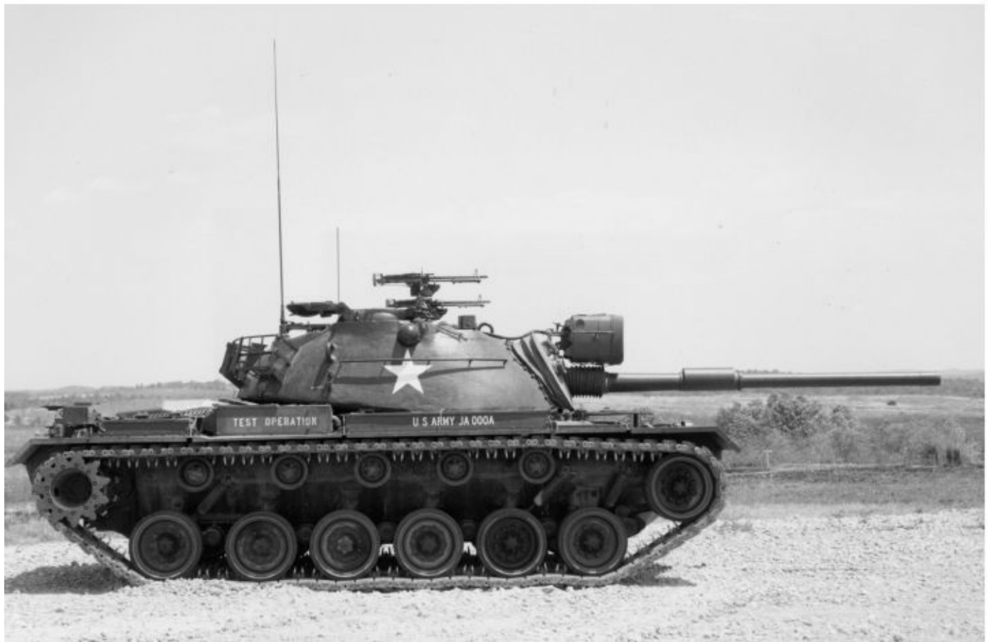
A side view of an M48A5PI tank. An important spotting feature of the M48A5PI tank is the M68 105mm main gun with a bore evacuator located roughly midway on the barrel. The M68 105mm gun on the M48A5-series tank is a modified license-built copy of the Royal Ordnance L7 series 105mm tank gun. Patton Museum
