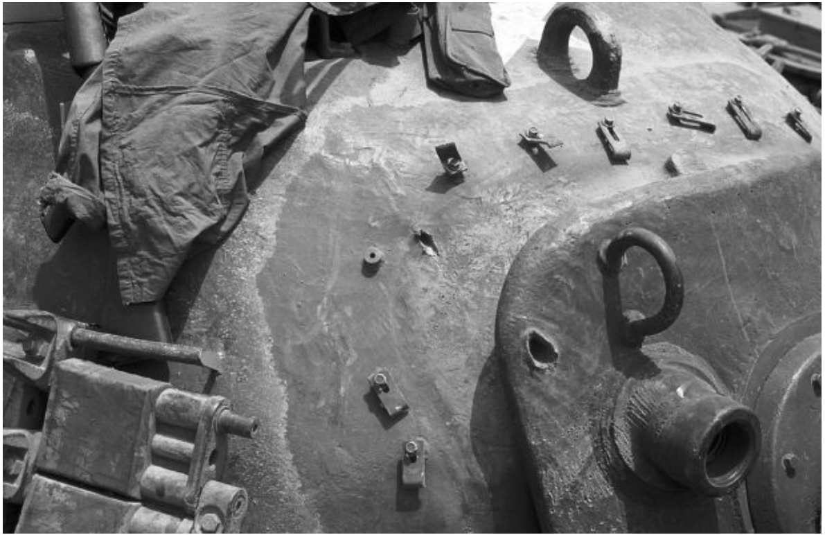
Pictured is an RPG-7 penetration of the thick armor of the gun-shield on an M48A3 tank in South Vietnam, which injured everybody in the vehicle. Despite having a maximum effective range of several hundred yards, the VC and NVA felt the closer the better and typically fired them at ranges of 55 yards (50m) and under to improve accuracy. Kent Hillhouse
