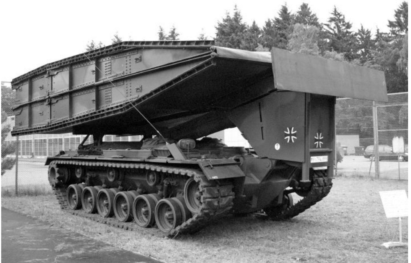
On display at the German Army Tank Museum is this AVLB based on the chassis of an M48A2 tank. The large flat metal plate just above the front of the tank's hull provides the base upon which the portable bridge rests as it is deployed into position Frank Schulz
