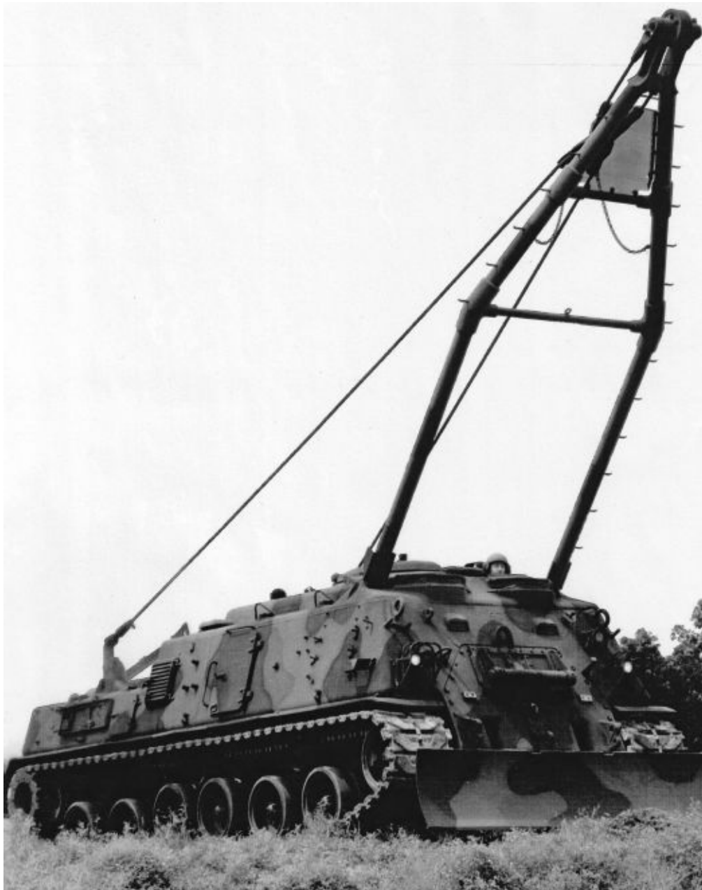
The erected "A" frame type hoisting boom of an M88 ARV appears in this picture. The boom was attached to the vehicle by a trunnion lever mounted on each side of the forward armored crew cab roof. The trunnion levers extended downward and connected to the hydraulic boom cylinders anchored to the vehicle's hull in the crew compartment. TACOM
