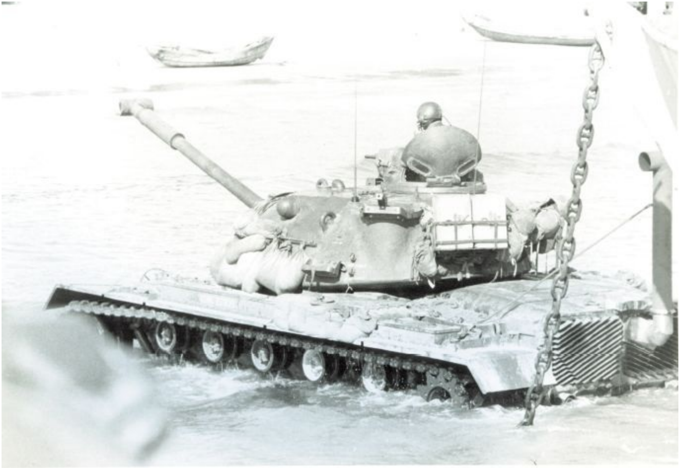
Coming off a U.S. Navy landing craft during the Vietnam War is a U.S. Marine Corps M48A3 tank. The vehicle is fitted with the deep water fording kit. Clearly visible at the rear of the engine compartment is the tall vertical fording exhaust stack. Patton Museum
