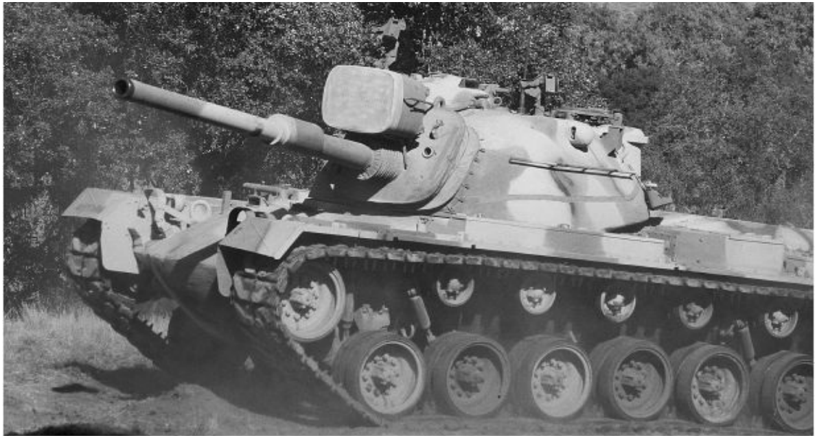
A California Army National Guard M48A5PI tank is shown. The 7.62mm M60D machine guns are not fitted on this vehicle. The thickest armor was on the front of the vehicle's turret and was 178mm, while the front upper hull armor was 110mm thick, sloped at 60 degrees. Michael Green
