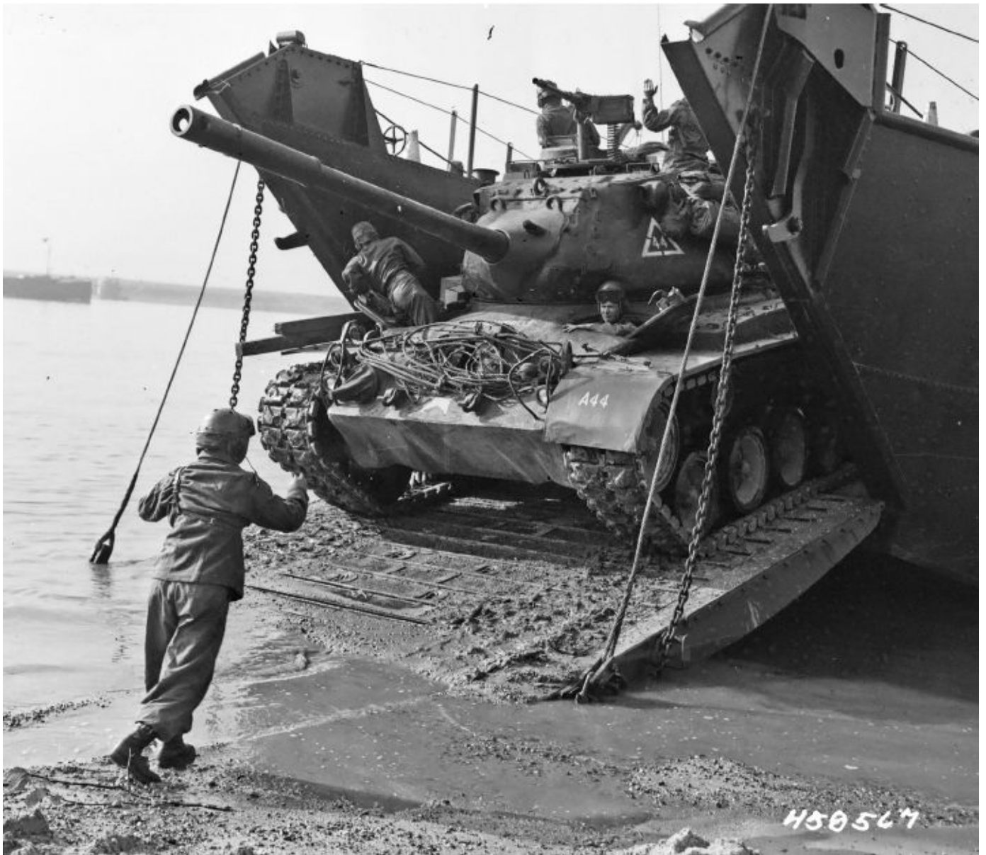
The crew of a U.S. Army M47 tank is shown carefully backing up their vehicle into a U.S. Navy landing craft. The M47 tank was 27 feet 11 inches (8.5m) long and had a width of 11 feet 6.3 inches (3.5m). The vehicle was 10 feet 11 inches (3.3m) tall and had a combat weight of 101,800 pounds (46,175.5kg). Patton Museum
