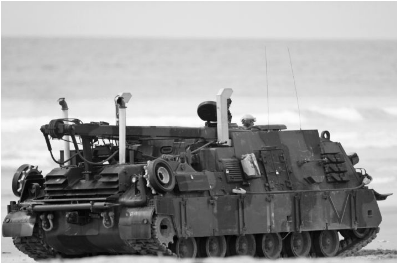
Taking part in a beach training exercise is a U.S. Marine Corps M88A2 ARV. Notice the fording equipment mounted on the rear of the vehicle's engine compartment. The M88A2 ARV is equipped with a Nuclear, Biological, and Chemical (NBC) protection system as well as a smoke screen generator. U.S. Marine Corps
