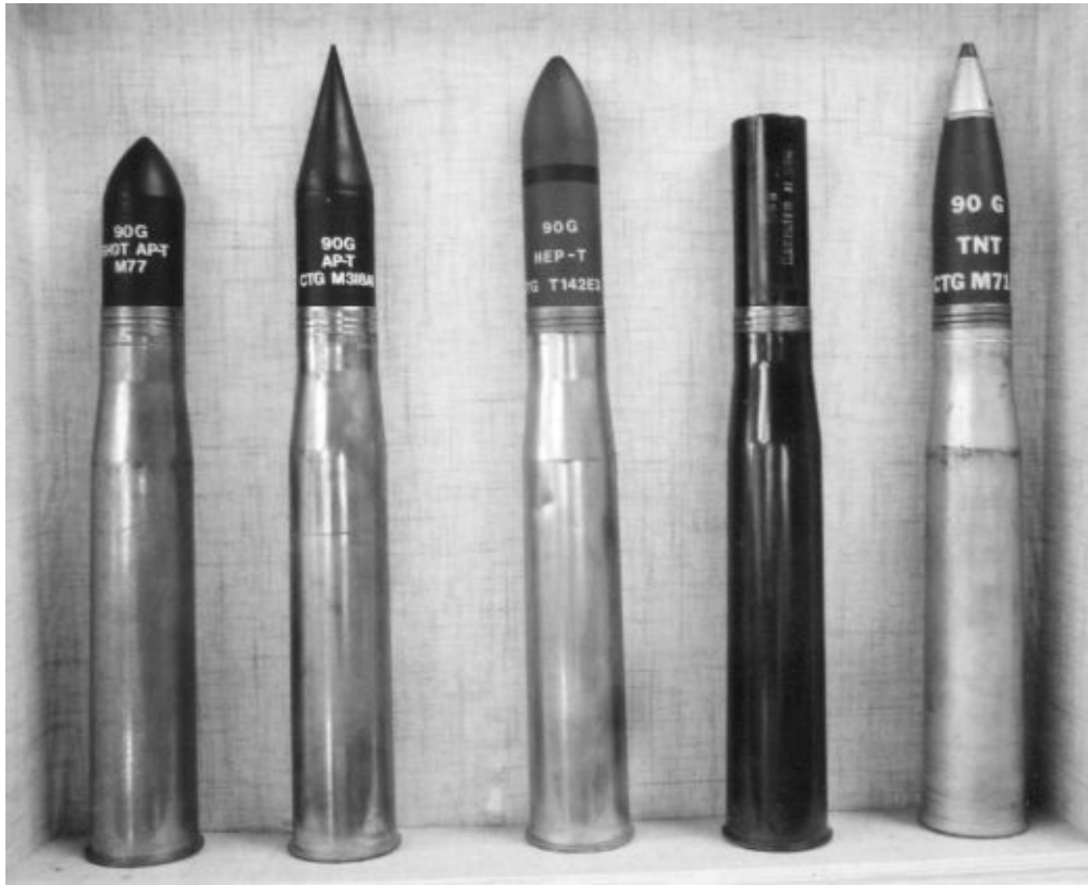
This photograph shows some of the main gun rounds fired from the M41 90mm main gun on the M48 series tanks. On the left are two kinetic energy rounds. In the middle is a high explosive plastic (HEP) round. To the right of the HEP round is an anti-personal canister round. On the far right is a high-explosive (HE) round with a fuze that can be set to detonate on contact or as a result of a delay action. Michael Green
