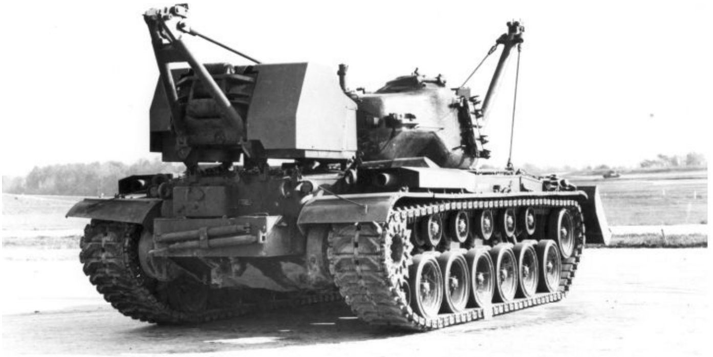
A rear view of the engineer armored vehicle T39 based on the chassis of the M46 series tanks. Visible on the rear engine deck of the vehicle is the housing for a 20-ton winch. There was storage space inside the vehicle for 26 main gun rounds. Patton Museum
