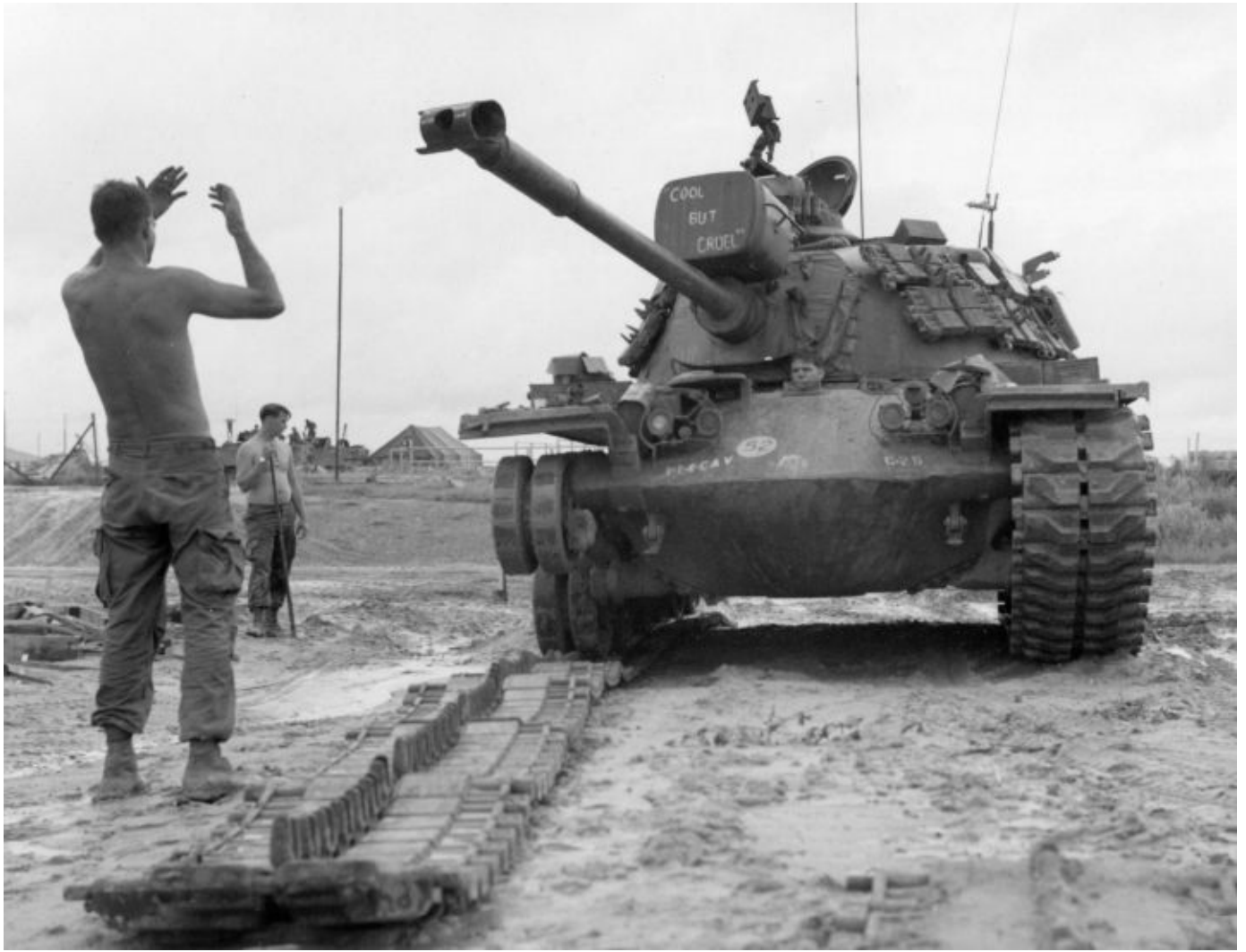
A dismounted U.S. Army tankerman is guiding the driver of his early-production M48A3 (Mod B) tank over a new track so it can be connected and the vehicle placed back in service. Convoy protection duties by tanks took a heavy toll of their tracks. Patton Museum
