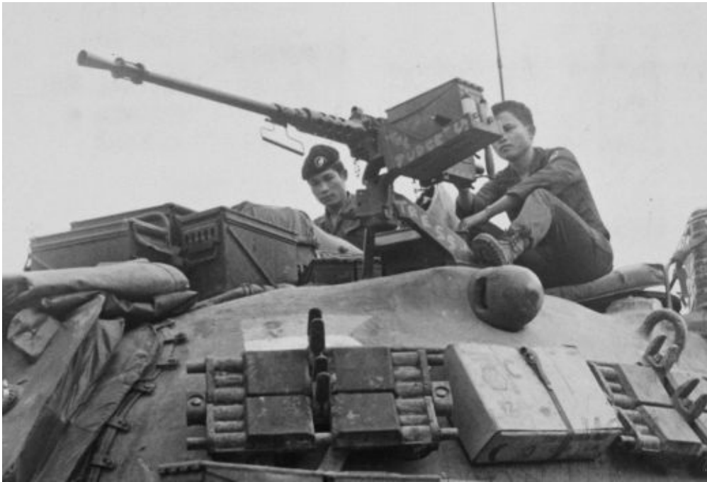
Here we see an M48A3 (Mod B) tank in the service of the Army of the Republic of Vietnam (ARVN) that has been modified to have the vehicle's .50 caliber (12.7mm) machine gun operated from the loader's position. Patton Museum
