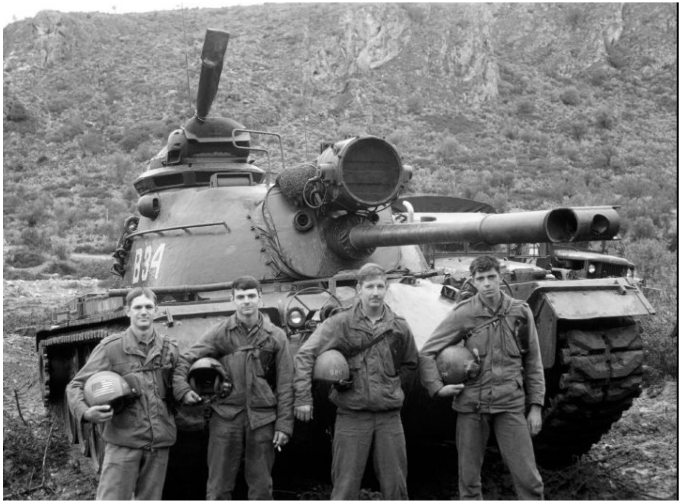
The four-man crew of a U.S. Marine Corps M48A3 tank nicknamed “The Grim Reaper” pose for the photographer in 1971. This tank had the G305 turret riser but had not yet gone through the Mod B upgrade program. The vehicle also retains the white light only 18-inch Crouse-Hinds searchlight that first appeared in use during the Korean War. Ken Estes
