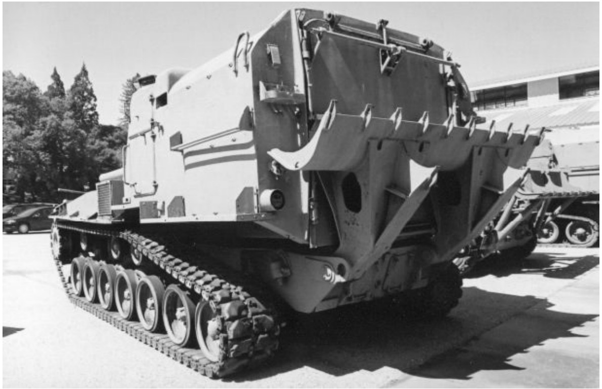
Clearly visible in this picture is the large rear hull spade of a 155mm self-propelled gun M53. The spade was lowered prior to action and helped to stabilize the gun when firing and absorbed some of the weapon's recoil. Michael Green
