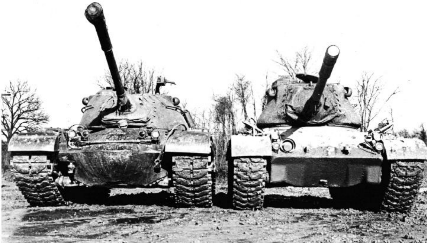
The large CHA hemispherical shaped turret of the T48 tank is clearly evident in this picture showing it parked next to an M47 tank. The rounded shape of the T48 tank turret was made possible by the adoption of the 85 inch (2.16m) diameter turret ring of the T43 tank. The turret ring diameter of the M47 tank was only 73 inches (1.85m). Patton Museum
