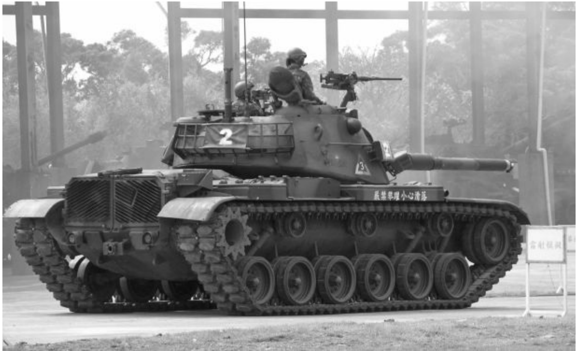
A Taiwan Army CM11 tank drives past a reviewing stand during a public demonstration. It retains the rear turret bustle rack that first appeared on the M48A1 tank. Notice the wind sensor stalk on the rear of the vehicle's turret. Chun-Lun Hsu
