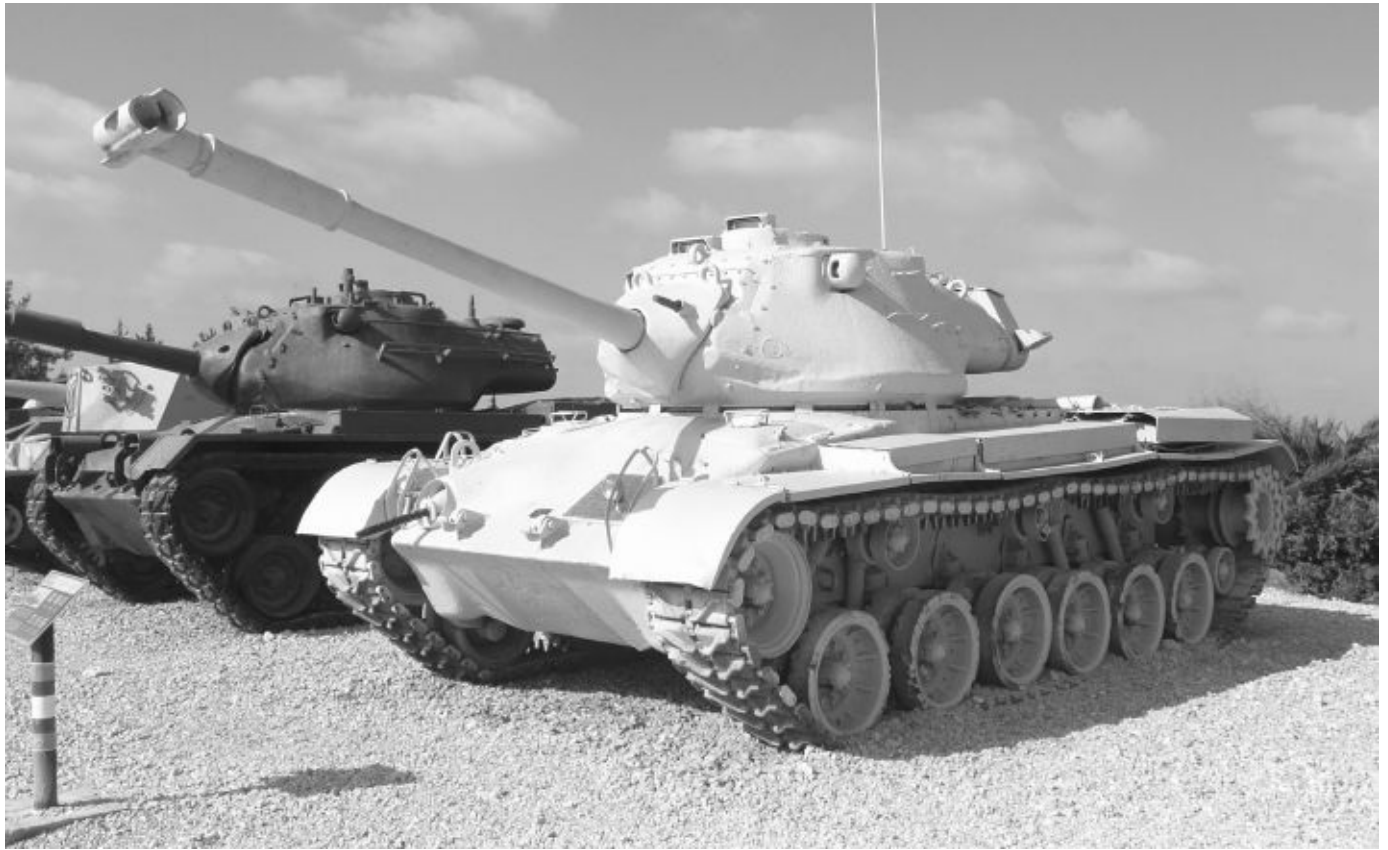
Belonging to the Israeli Armored Corps Memorial Site and Museum in Latrun, Israel, is this M47 tank captured from the Royal Jordanian Army Corps during the 1967 Six-Day War. The vehicle is no longer in its original paint scheme. It has the late production T-shaped blast deflector. Vladimir Yakubov
