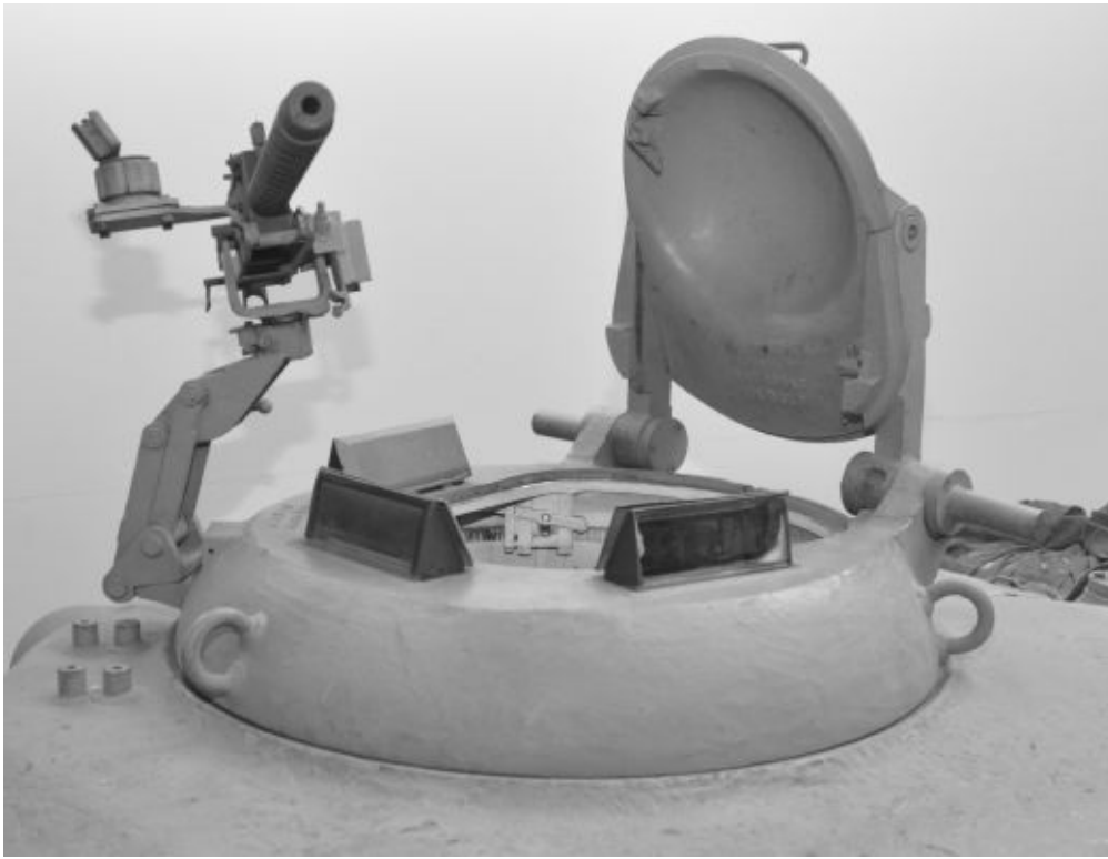
Following the 1967 Six Day War, the IDF set about replacing the American-designed M1 cupola on its M48 tank series with a new low-profile cupola named the “ Urdan ” after the Israeli company that designed and built it. Pictured is an Urdan cupola on an IDF Magach 3 tank. Chris Hughes
