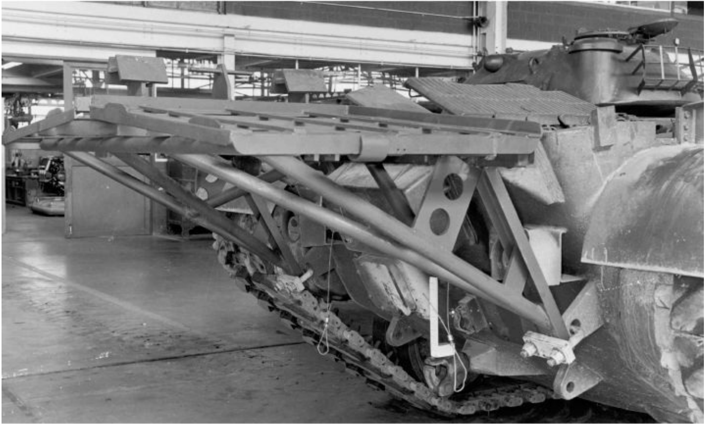
Shown without the four unarmored 55 gallon fuel drums fitted is the metal rack that attached to the rear of the M48A1 tank. If the need arose, the metal rack could be jettisoned from within the vehicle. Patton Museum
