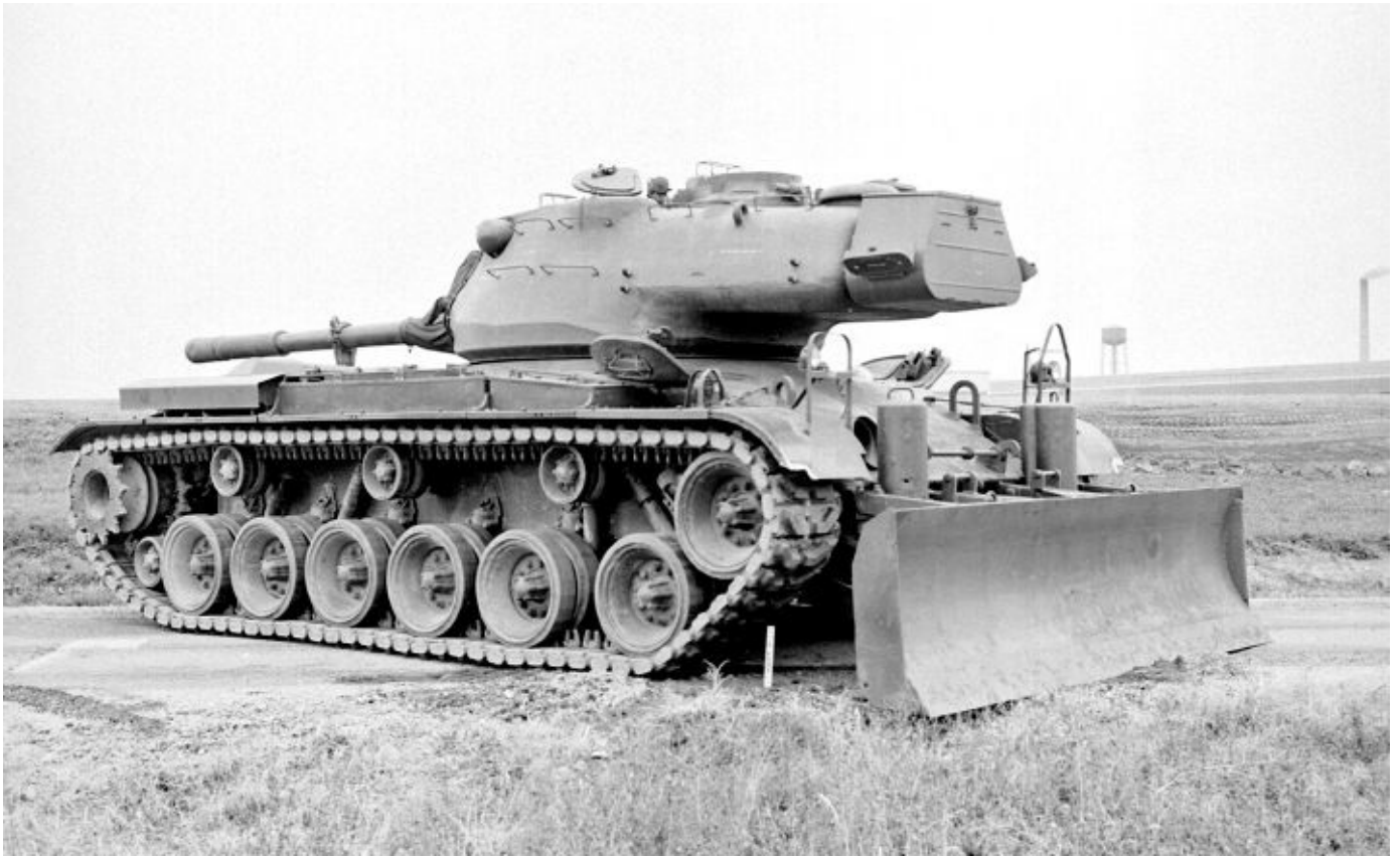
Mounted on the front of this M47 tank is the tank mounted, bulldozer M3. This was the replacement for the M1 and M2 series bulldozer employed on the M4 series tanks during the Second World War. Patton Museum
