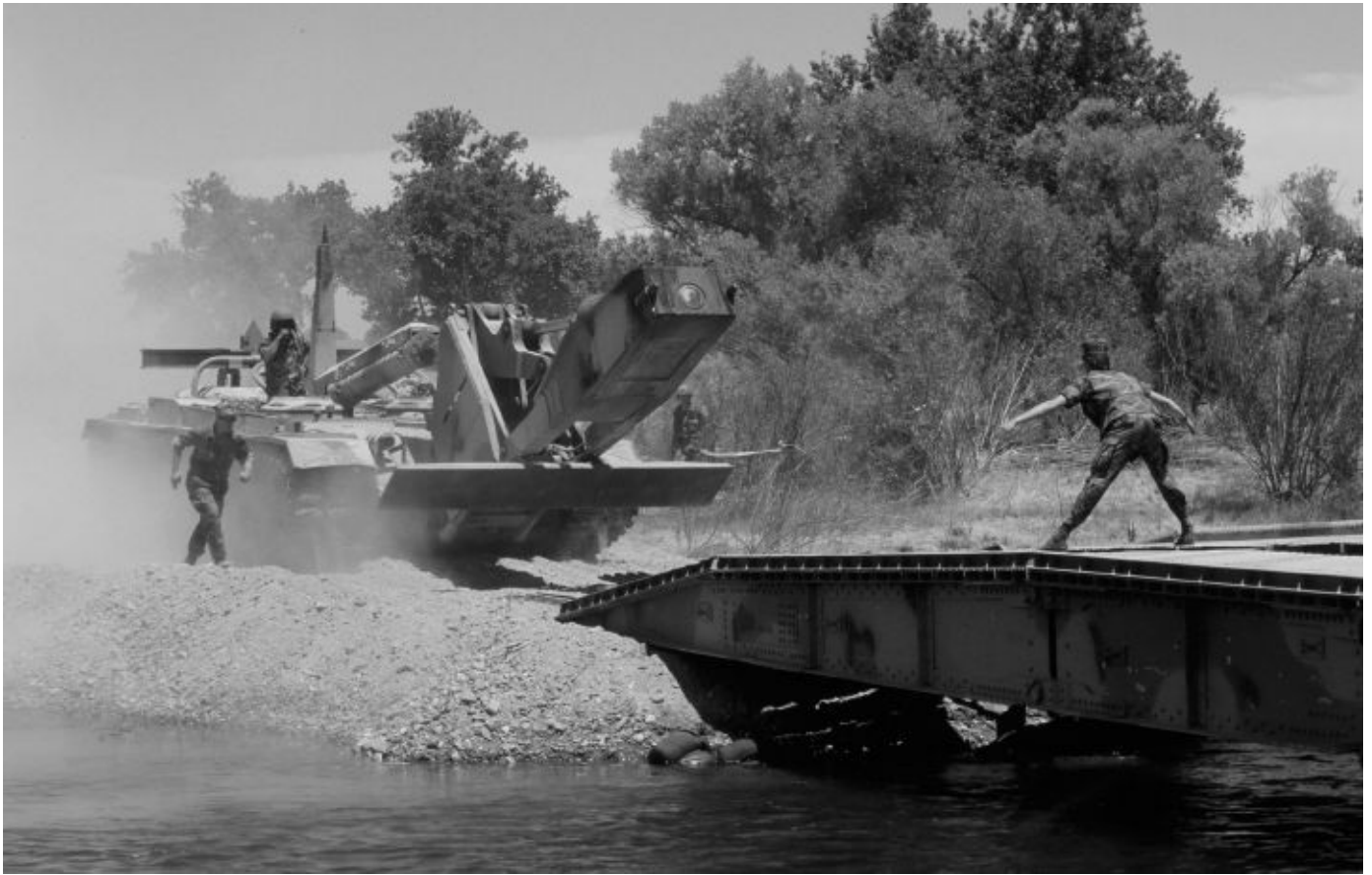
A California Army National Guard AVLB based on the chassis of an M48A5 tank is shown in the process of recovering its 63-foot span aluminum scissoring type-bridge. The controls for launching and retrieving the bridge were located in front of the driver's seat. Michael Green
