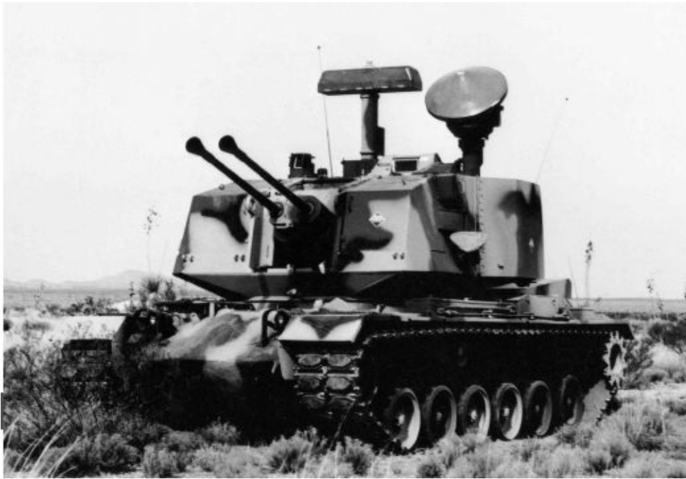
A Ford Aerospace Division Air Defense (DIVAD) gun system, also known as the M247 Sergeant York, is shown posed for a publicity picture. The two 40mm guns in the 360 degree rotating turret had a rate of fire per gun of 600 rounds per minute and could reach out and strike targets at about seven miles (12.5km). TACOM
