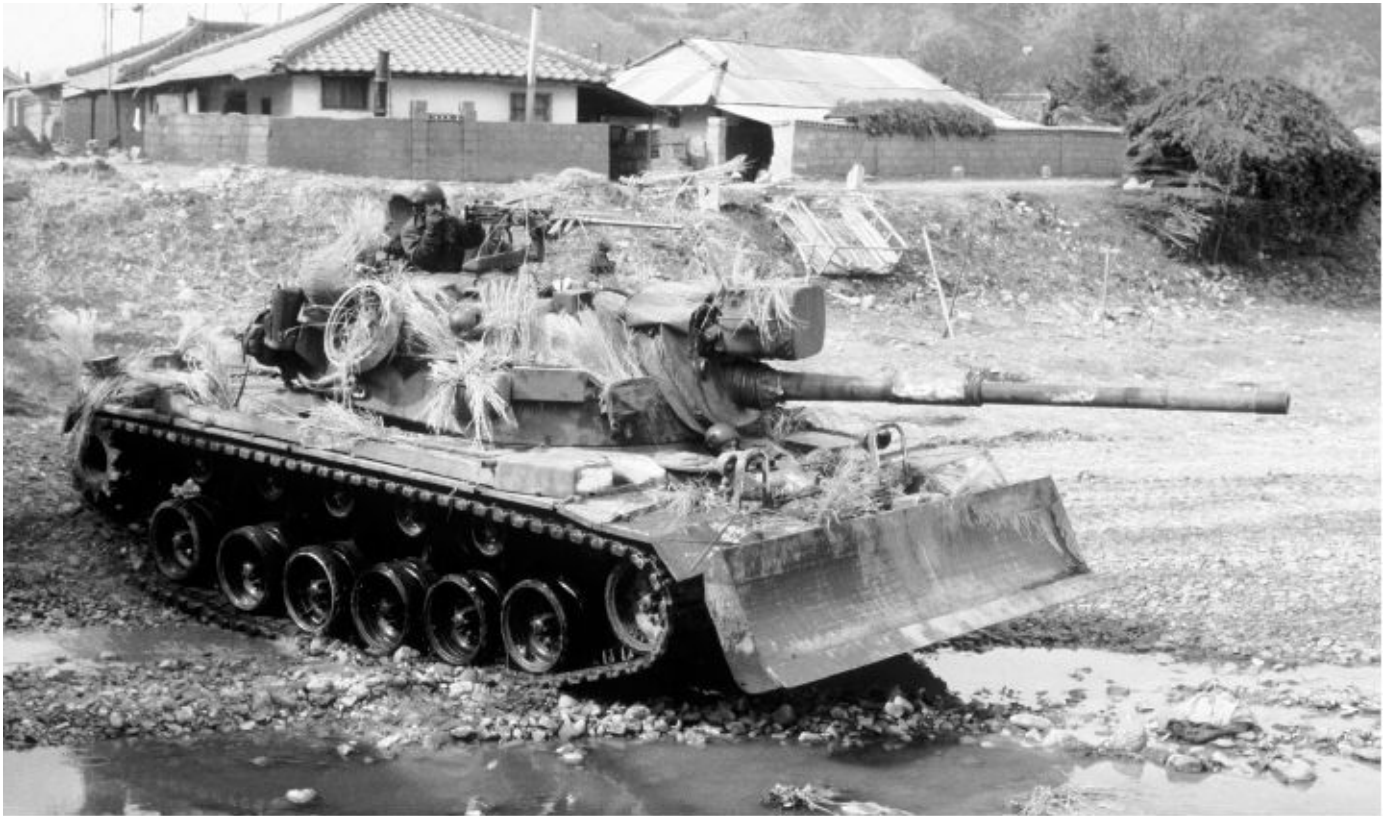
This picture taken during a large-scale training exercise in South Korea shows a South Korean Army M48A5PI equipped with a tank mounted bulldozer M8A3. The bulldozer blade is shown in its raised travel position. Notice the raised headlight arrays on this tank. TACOM
