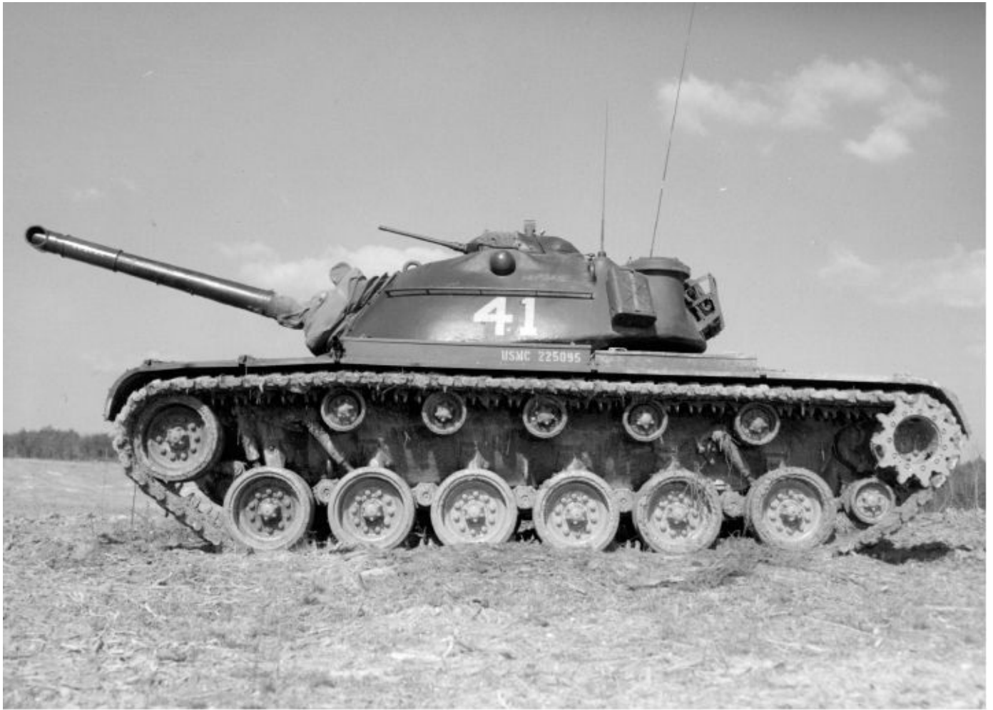
A side view of a U.S. Marine Corps flame thrower tank M67 that was based on a modified M48A1 tank. Since the vehicle had no cannon, the loader's position was done away with and replaced with a large container of napalm, bringing the crew down to three men. The M6 flame gun was housed in a metal shroud intended to mimic the appearance of the standard 90mm main gun. Patton Museum
