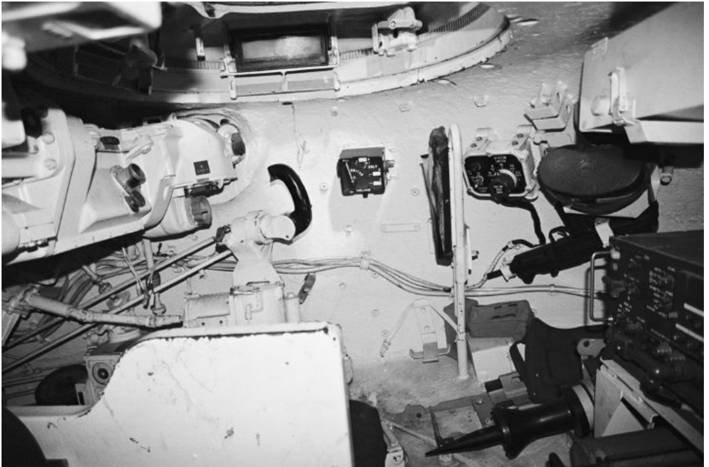
This picture was taken from the loader's side of an IDF Magach 3 looking towards the tank commander's position. In the lower left foreground of the photograph is the recoil guard. Above the recoil guard is the rangefinder. The black handgrip is the tank commander's power control assembly, which affords him a capability identical to that of the gunner. Michael Green
