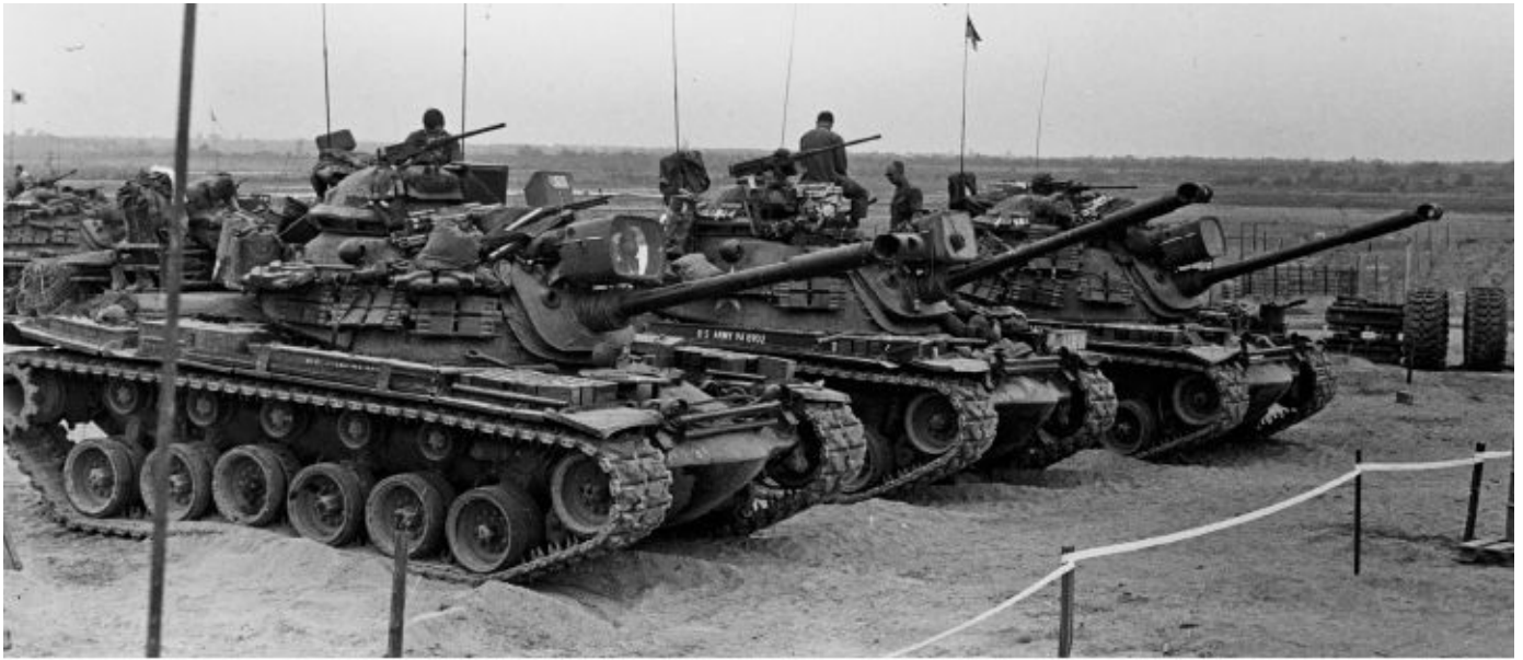
Pictured is a formation of late production U.S. Army M48A3 (Mod B) tanks in South Vietnam. The tank crews have affixed engineer stakes horizontally over the lower portion of the vehicle's glacis to prevent vegetation riding up and injuring the driver when jungle busting. Patton Museum
