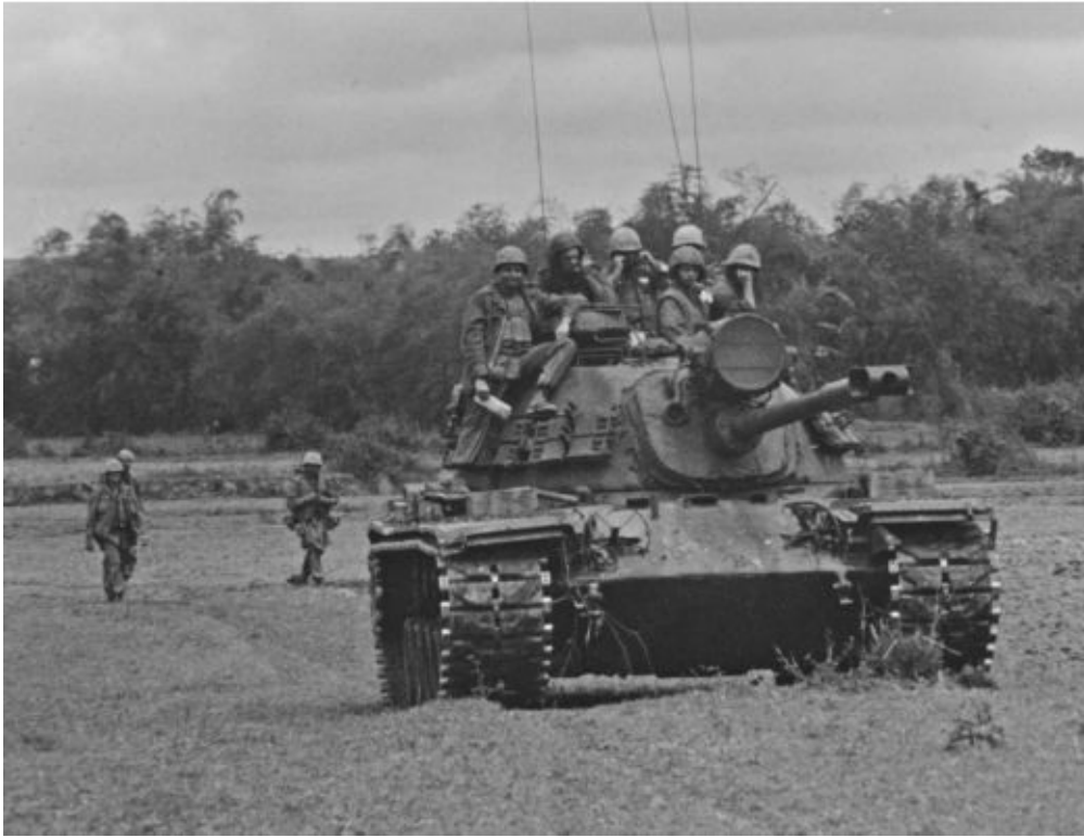
A U.S. Marine Corps M48A3 tank is seen carrying a group of Marine infantrymen. The vehicle is equipped with a Korean War vintage 18-inch Crouse-Hinds searchlight. Notice the infantrymen behind the tank are walking in the track impressions to avoid enemy antipersonnel mines or booby traps. Patton Museum
