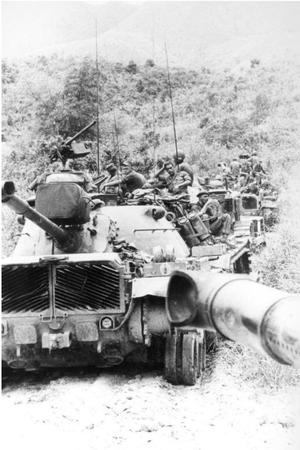
Not all M48A3 tank commanders favored mounting their .50 caliber (12.7mm) machine guns on the roof of the M1 cupolas. The early production M48A3 (Mod B) tank being towed has a .30 caliber (7.62mm) machine gun mounted on the roof of the M1 cupola. Notice the early-type taillight brush guards on this vehicle. Patton Museum
