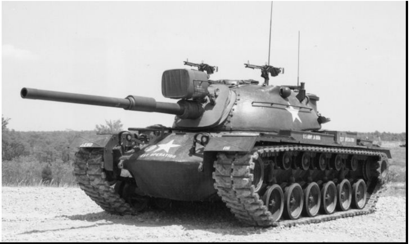
Pictured is an M48A5PI with various Israeli-inspired upgrades, including the new low-profile cupola and the addition of two 7.62mm M60D machine guns located at both the tank commander and loader stations. Patton Museum
