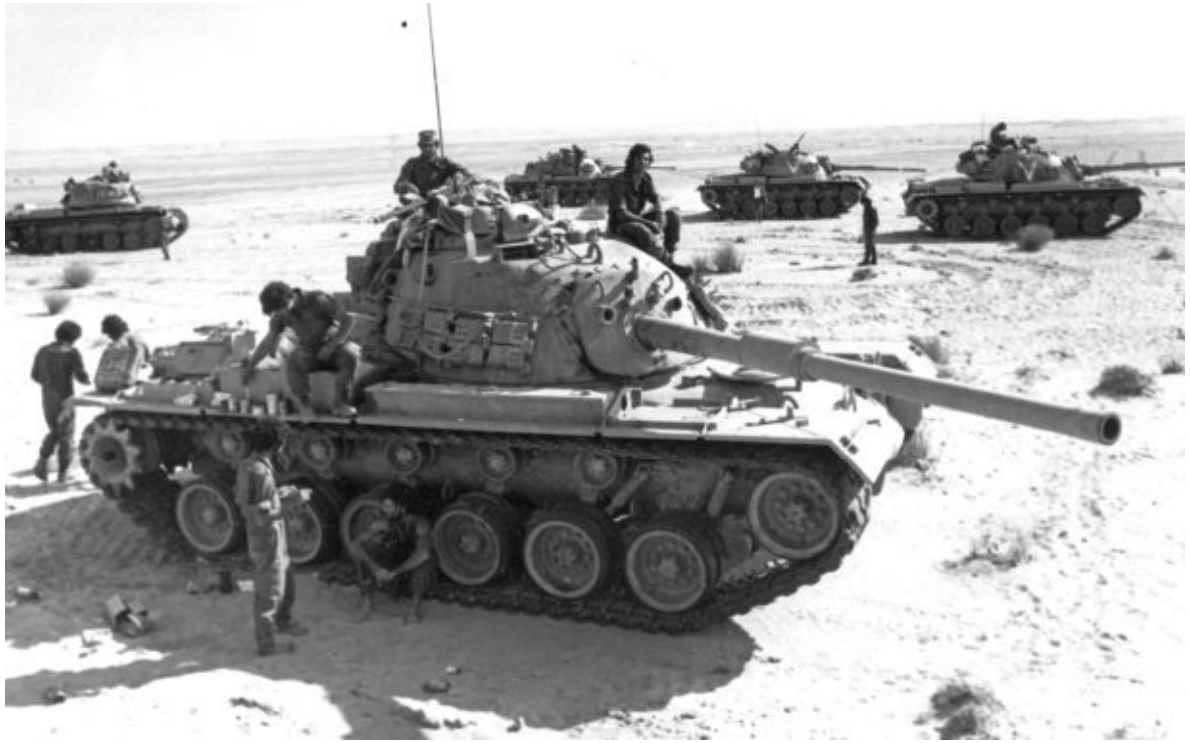
This picture shows a formation of IDF Magach 3 tanks on patrol in the Sinai Peninsula sometime before the 1973 Yom Kippur War. Despite having been upgraded with a 105mm main gun and a diesel engine, the vehicles shown still have the unsatisfactory original American-designed and built M1 cupola. IDF
