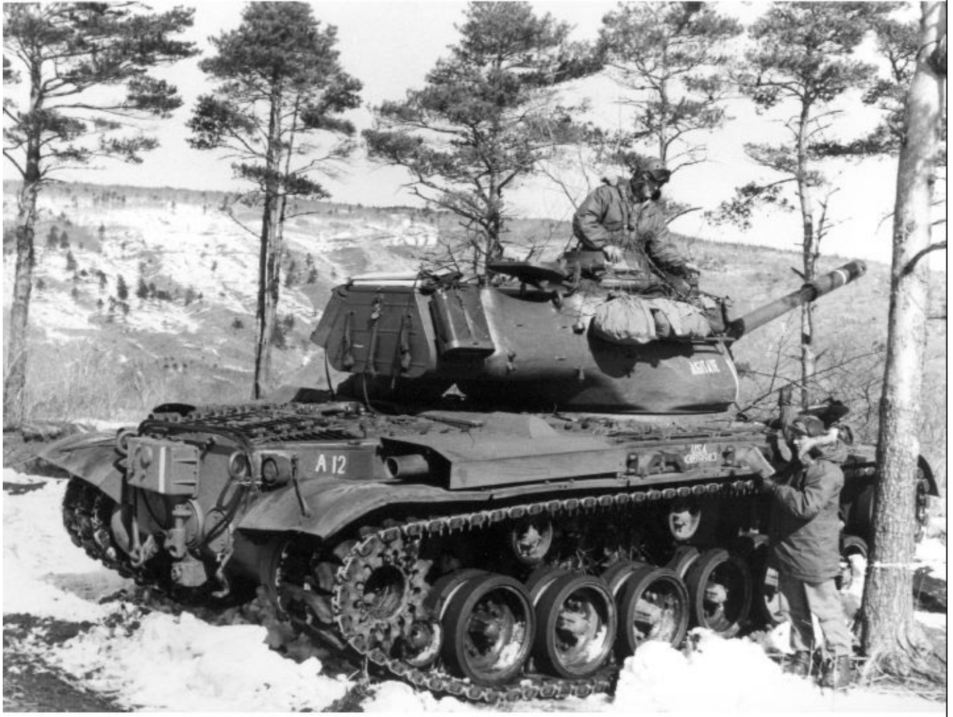
Pictured is a U.S. Army M47 tank that is taking part in a field training exercise near Mount Fuji, Japan in February 1956. Unlike the suspension system on the M46 series tanks that had five track return rollers, the M47 tank only had three. Patton Museum
