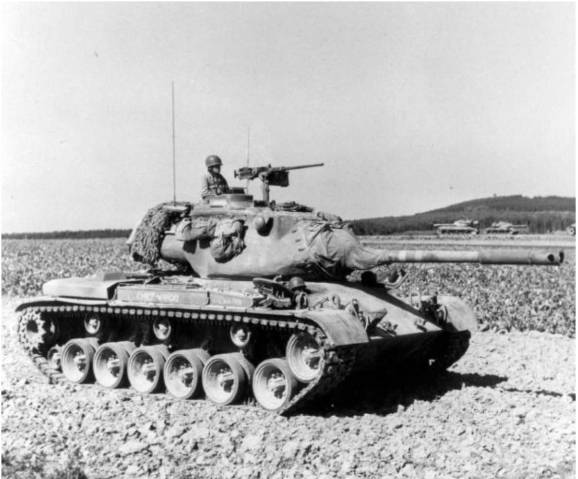
Taking part in a Western European training exercise is a platoon of U.S. Army M47 tanks. The vehicle rode on a torsion bar suspension system with 12 individually sprung dual road wheels (six per side) and six dual track return rollers (three per track). Patton Museum
