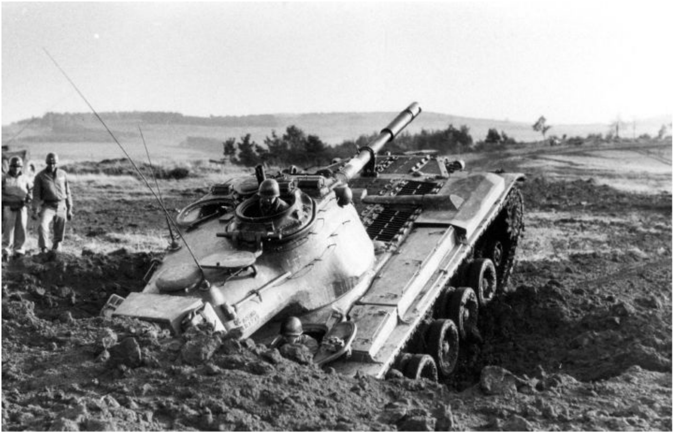
The crew of a U.S. Army M47 tank is trying to cross a field obstacle. The vehicle could handle a grade of 60 percent and cross over a trench 8.5 feet (2.6m) wide. Like all American postwar tanks, it had the ability to climb a vertical wall 36 inches (91.4cm) tall. Patton Museum
