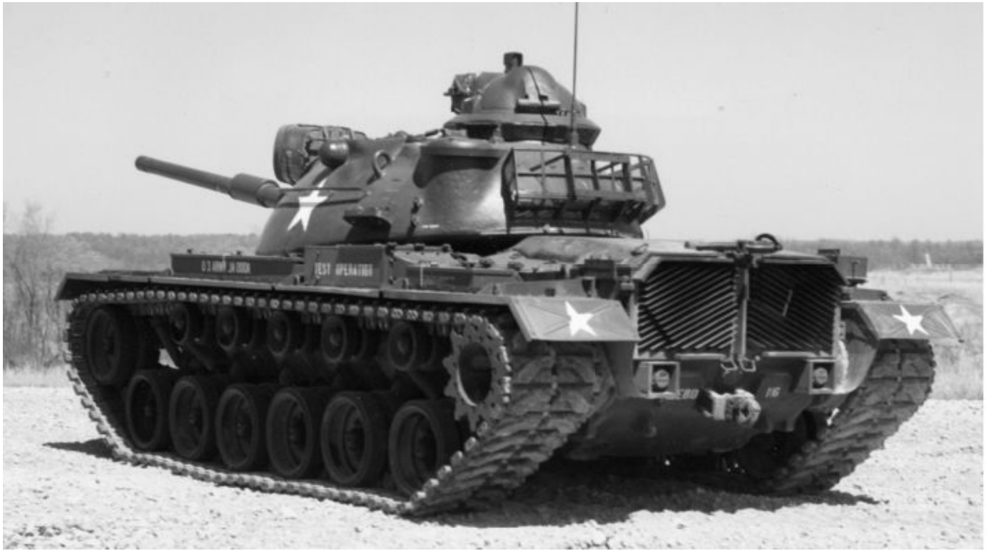
This picture shows a rear view of an early production M48A5 tank with the M48A3 (Mod B) tank configuration features, which included the bulged tank commander's overhead hatch. Notice the late production M48A3 (Mod B) tank configuration strengthened rear fender extensions with the embossed X-pattern. TACOM
