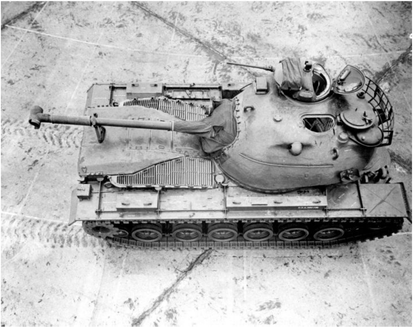
A big problem with the M48 and M48A1 tanks was their large infrared signature. The solution shown on the M48A2 tank pictured was a redesigned and enlarged rear engine compartment that significantly cut down on the vehicle's infrared signature. Also visible are the horizontal air intake grills along each side of the solid center section. Patton Museum
