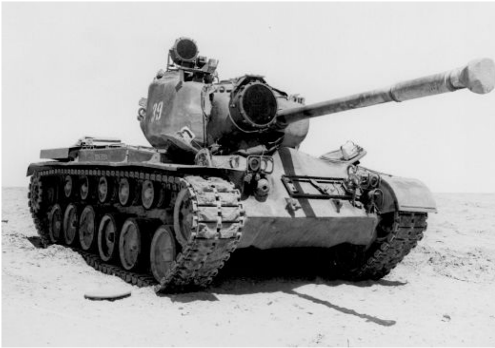
Shown is a U.S. Army M46 series tank fitted with a large infrared searchlight mounted on the right side of the gun shield. The infrared viewer is mounted on the front of the tank commander's cupola. The codename for the installation shown was Leaflet II. Patton Museum
