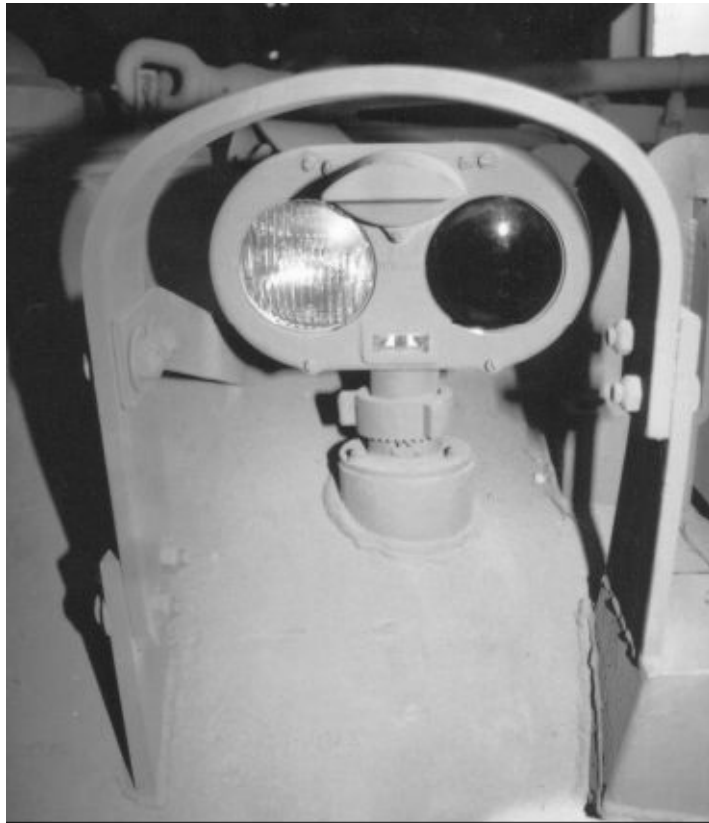
A close-up photograph of one of the two identical headlight clusters that first appeared on the front hulls of M48A2 tanks. This same headlight cluster arrangement and brush guard would remain on all the follow-on vehicles of the M48 tank series. Michael Green
