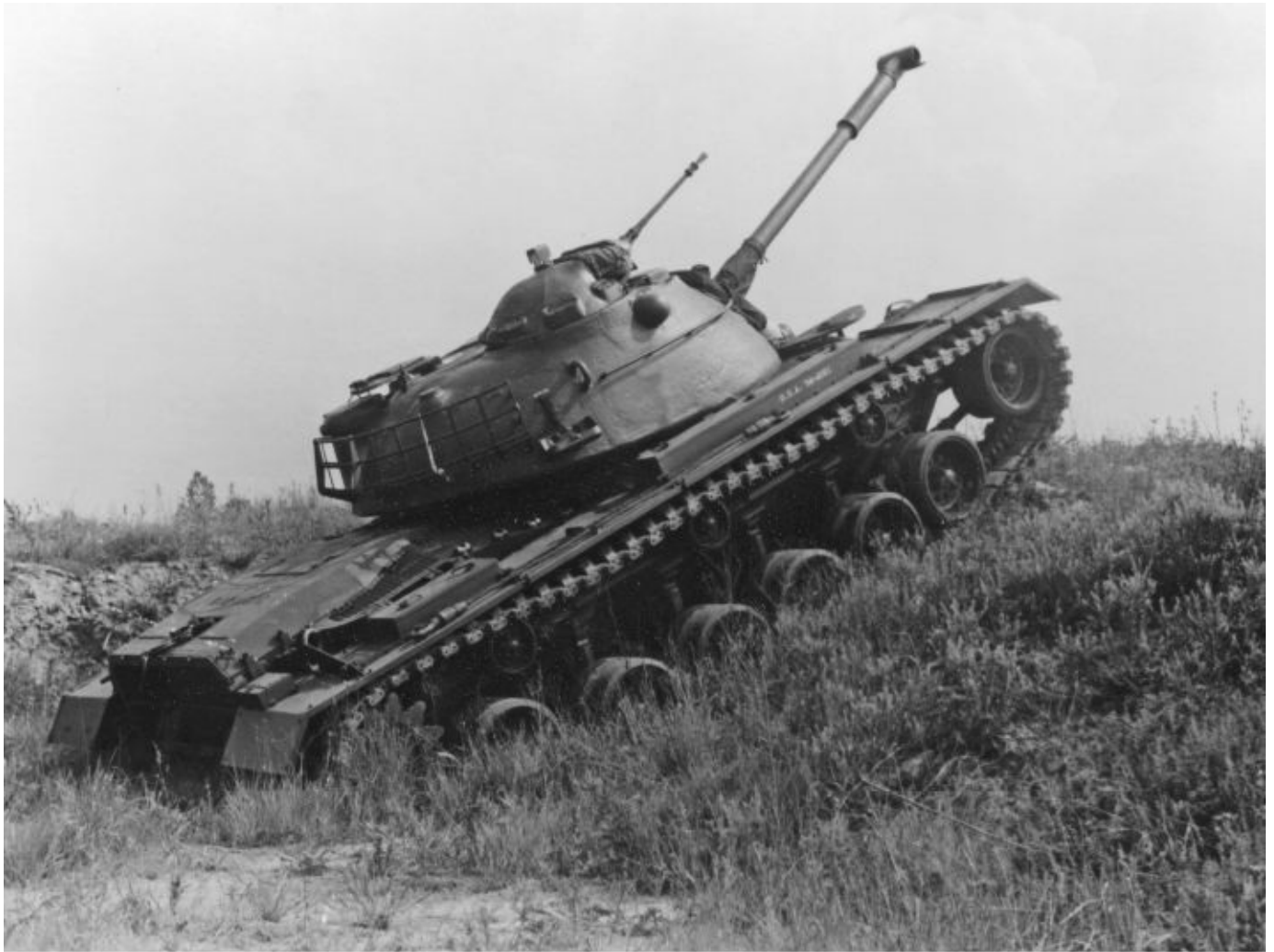
This picture shows the redesigned and enlarged rear engine compartment of an M48A2 tank. The solid center section of the rear hull roof compartment covered an insulated exhaust tunnel that discharged the engine's exhaust gases out the rear of the tank's hull. Notice the semi-enclosed turret bustle rack that first appeared on the M48A1 tank. Patton Museum
