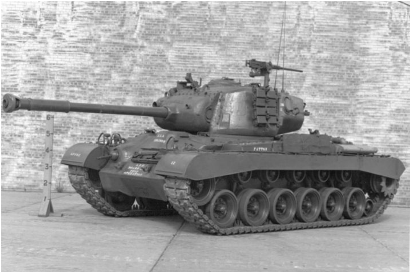
The financial constraints that forced the US to modernise rather than replace its M26 stocks led to the construction of ten vehicles designated T40, one of which is shown here. Patton Museum
