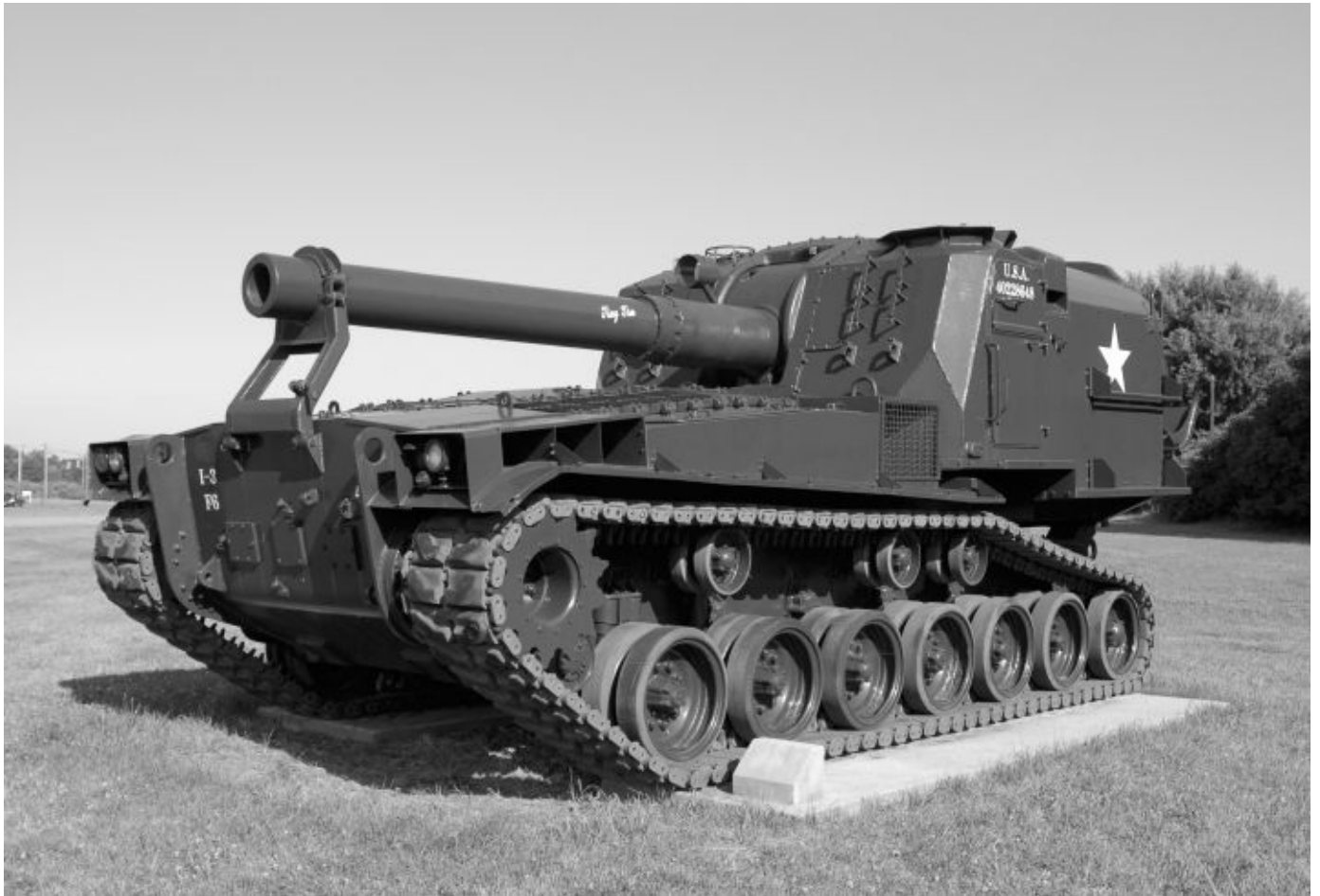
The 8-inch self-propelled howitzer M55 pictured belongs to the U.S. Army Ordnance Museum collection. Armor protection on the M55 was limited to 13mm, except for the vehicle's front hull plate that was 25mm thick. The M55 had storage space for 10 rounds of 8-inch ammunition onboard. Christopher Vallier
