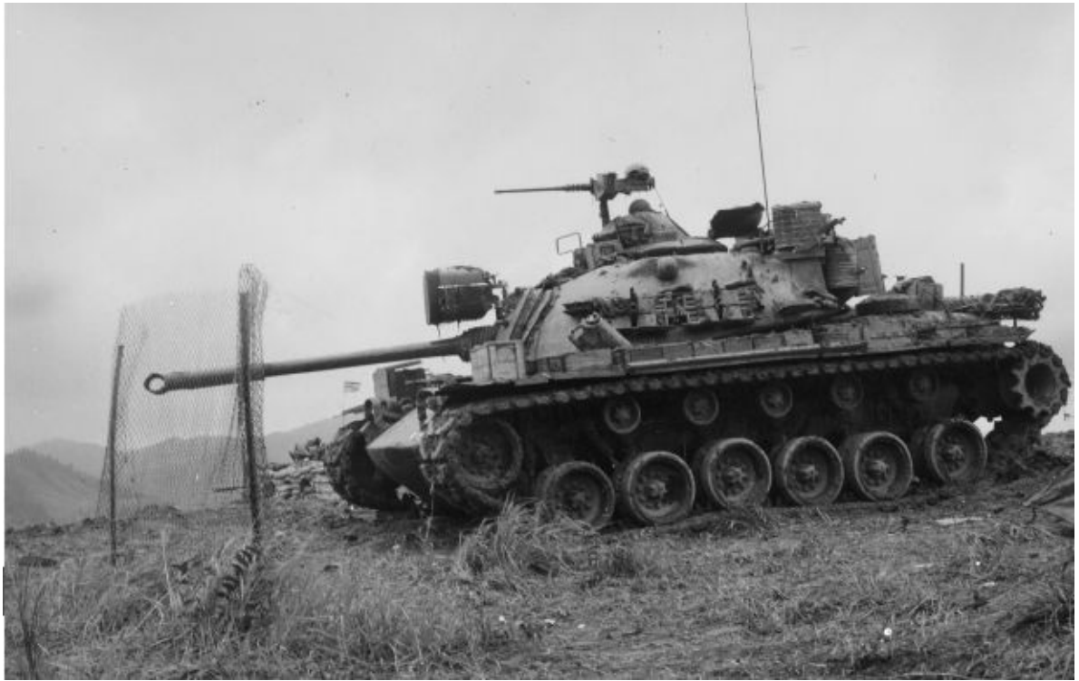
The VC and NVA favored attacking American military ground forces at night to offset their firepower advantage. It was a common practice to install cyclone fencing (attached to engineer stakes) in front and around M48A3 tanks when halted at night to pre-detonate incoming RPG-7 projectiles. Pictured is an example of that practice. Patton Museum
