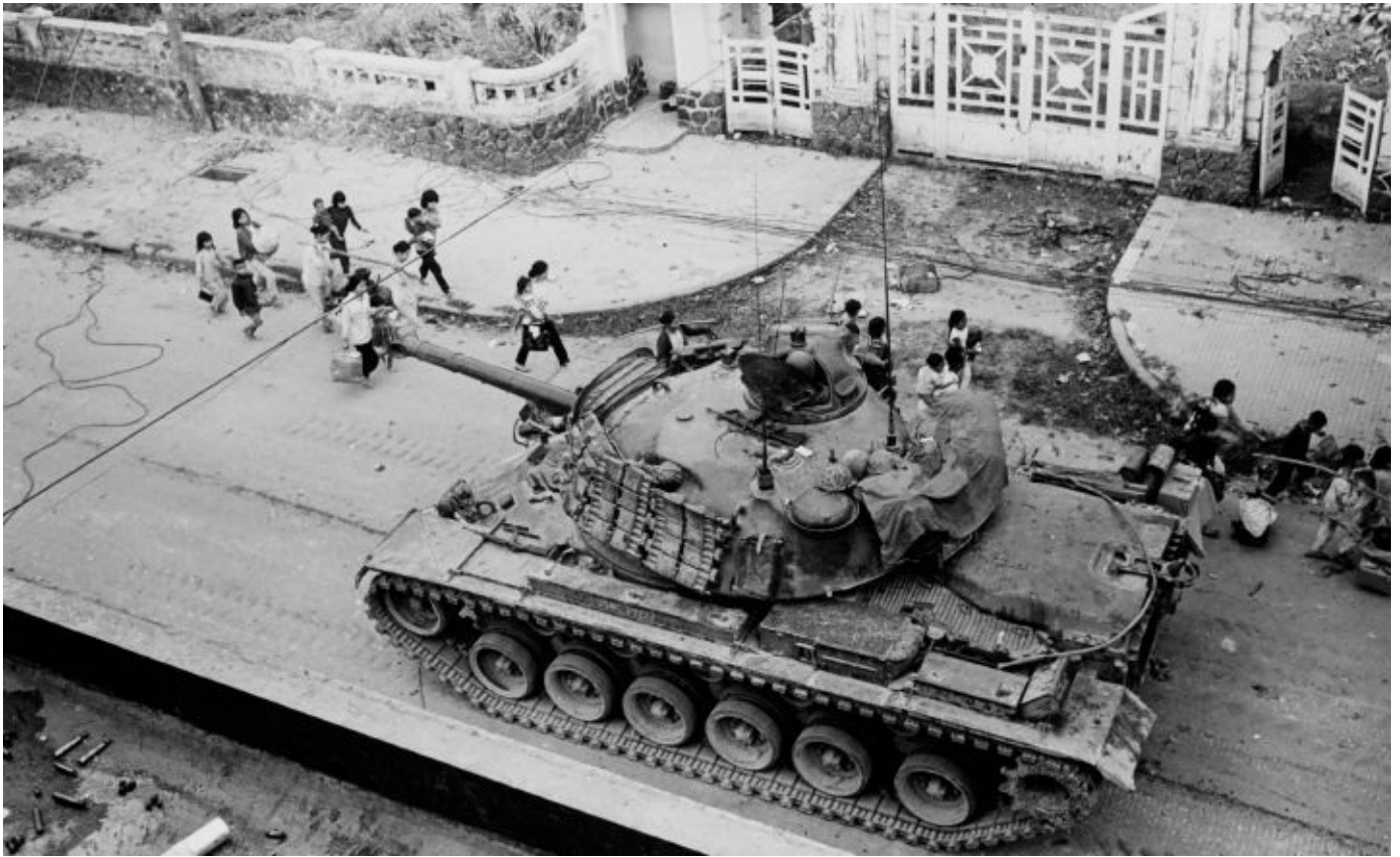
A U.S. Marine Corps full-tracked combat tank, flame thrower M67A2 is pictured in South Vietnam as refugees from the fighting stream past. Very evident in this picture is the shorter and stubbier appearance of the metal shroud for the M6 flame gun that identifies it as an M67A2 and not a standard M48A3 tank. Patton Museum
