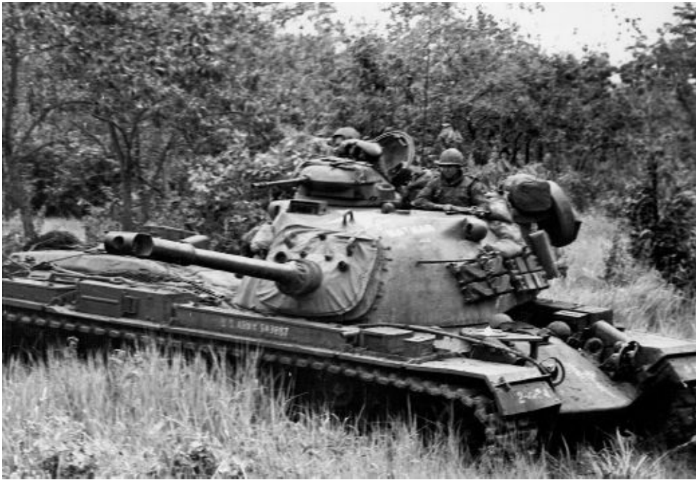
Pictured is a U.S. Army M48A3 tank somewhere in South Vietnam. The loader is armed with a Second World War-era M3 or M3A1 submachine gun, popularly known as the “Grease Gun.” Notice the spare road-wheel attached to the rear turret bustle rack. Patton Museum
