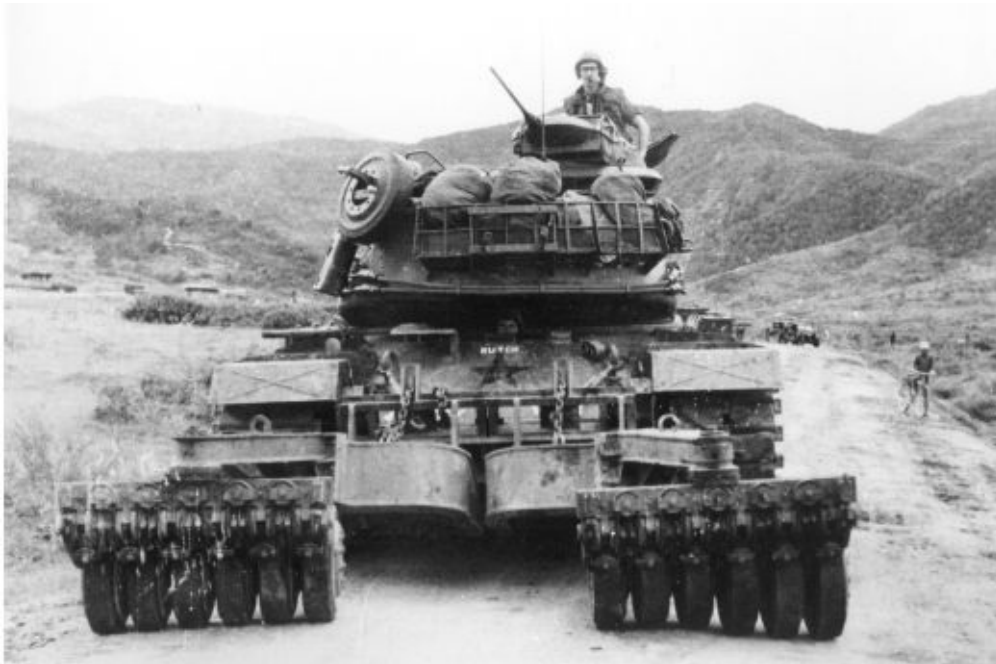
Pictured mounted to the front of a U.S. Army M48A3 tank during the Vietnam War is the ENSURE 202 expandable mine clearing roller. The 10,000 pound device was made up of 12 modified tank road wheels divided into two separate six-wheel roller assemblies that were each 47 ½ inches wide. TACOM
