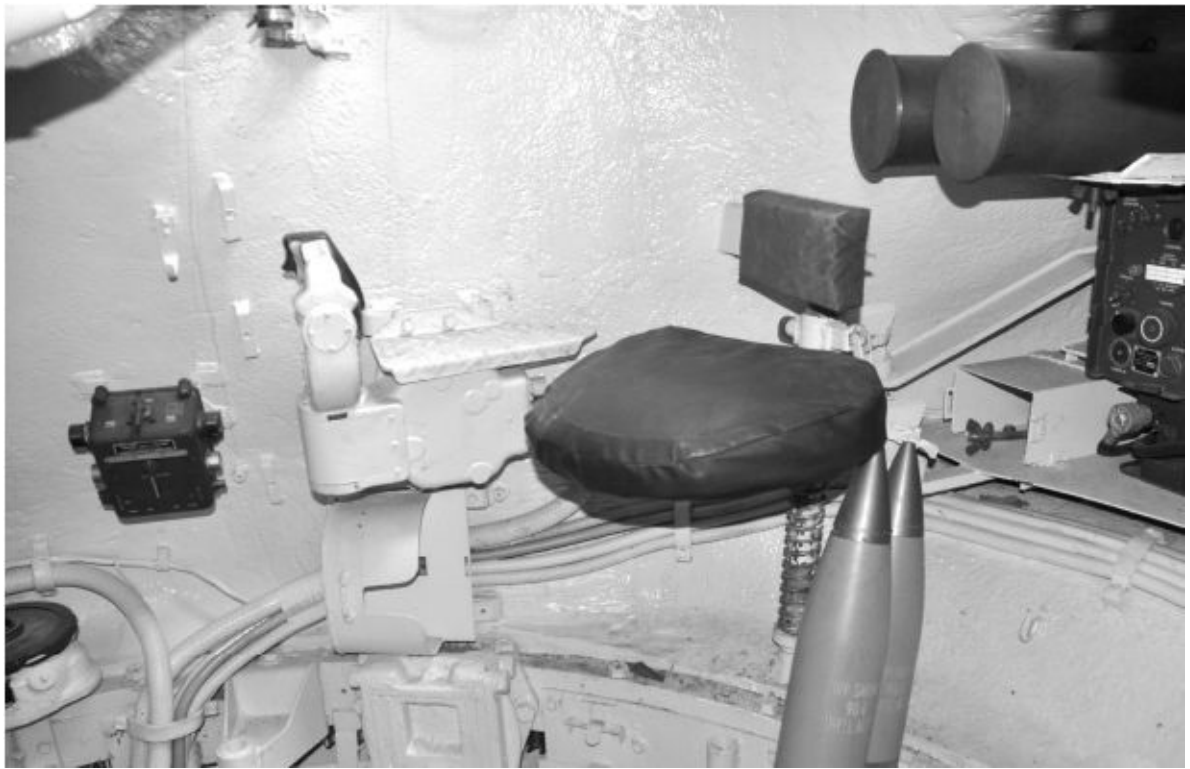
A picture taken from the loader's position on an M47 tank shows the vehicle commander's seat, which is located behind and just above the gunner's seat that is visible in the lower left portion of the picture. The tank commander stood on his seat when looking out over the top of his cupola. Chris Hughes
