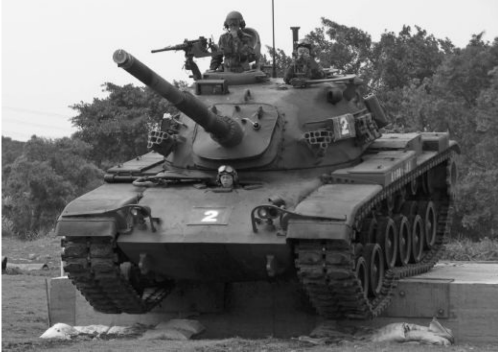
This picture shows a Taiwanese Army CM11 tank, officially nicknamed the “Brave Tiger,” which consists of an M48A2 turret equipped with a 105mm main gun and an advanced fire-control system. The upgraded turret, which has an Urdan cupola, is mounted on the chassis of an M60A3 tank. Chun-Lun Hsu
