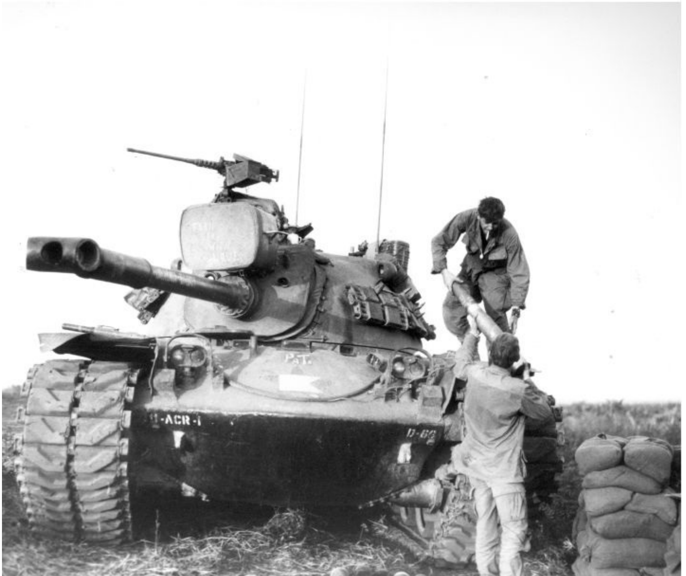
Late-production M48A3 (Mod B) tanks can normally be identified by the new squared brush guards around the front hull-mounted headlight clusters. Those squared brush guards can be seen in this picture showing a couple of tankers loading up their vehicle with main gun rounds in South Vietnam. Patton Museum
