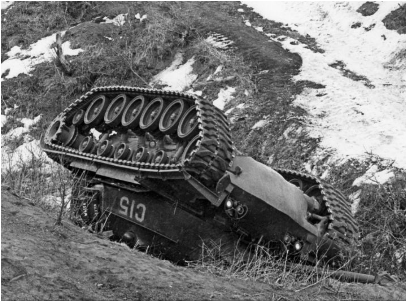
Pictured is an overturned U.S. Marine Corps M48A1 tank. Driving any large tracked vehicle on side slopes can be extremely difficult as they have a tendency to drift downhill. It is up to the driver to perform constant corrections to keep the vehicle straight. RC McInteer collection
