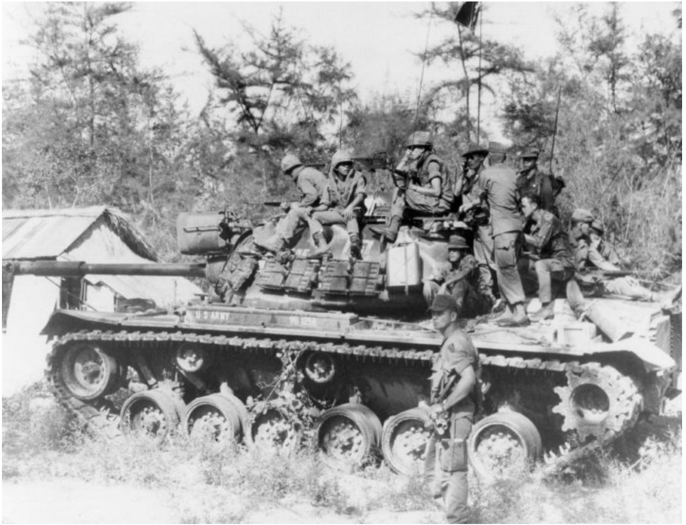
Army of the Republic of South Vietnam (ARVN) troops ride into action on a U.S. Army M48A2C tank. The most noticeable features that identifies the vehicle pictured as an M48A2C tank is the lack of a large box-like dry type cleaner box as seen on M48A3 tanks and the lack of track tension idler between the last set of road wheels and the rear hull-mounted drive sprocket. A U.S. Army combat cameraman is standing next to the vehicle. Patton Museum
