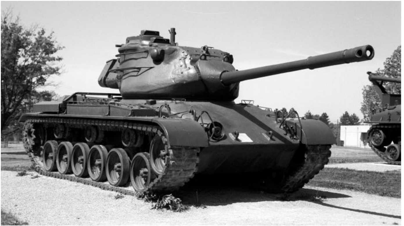
This M47 tank is pictured on display at the former Patton Museum of Armor and Cavalry. Notice the cylindrical blast deflector. The tank carried 71 main gun rounds for its M36 90mm cannon and 11,150 rounds of ammunition for its two .30 caliber (7.62mm) machine guns. Richard Hunnicutt
