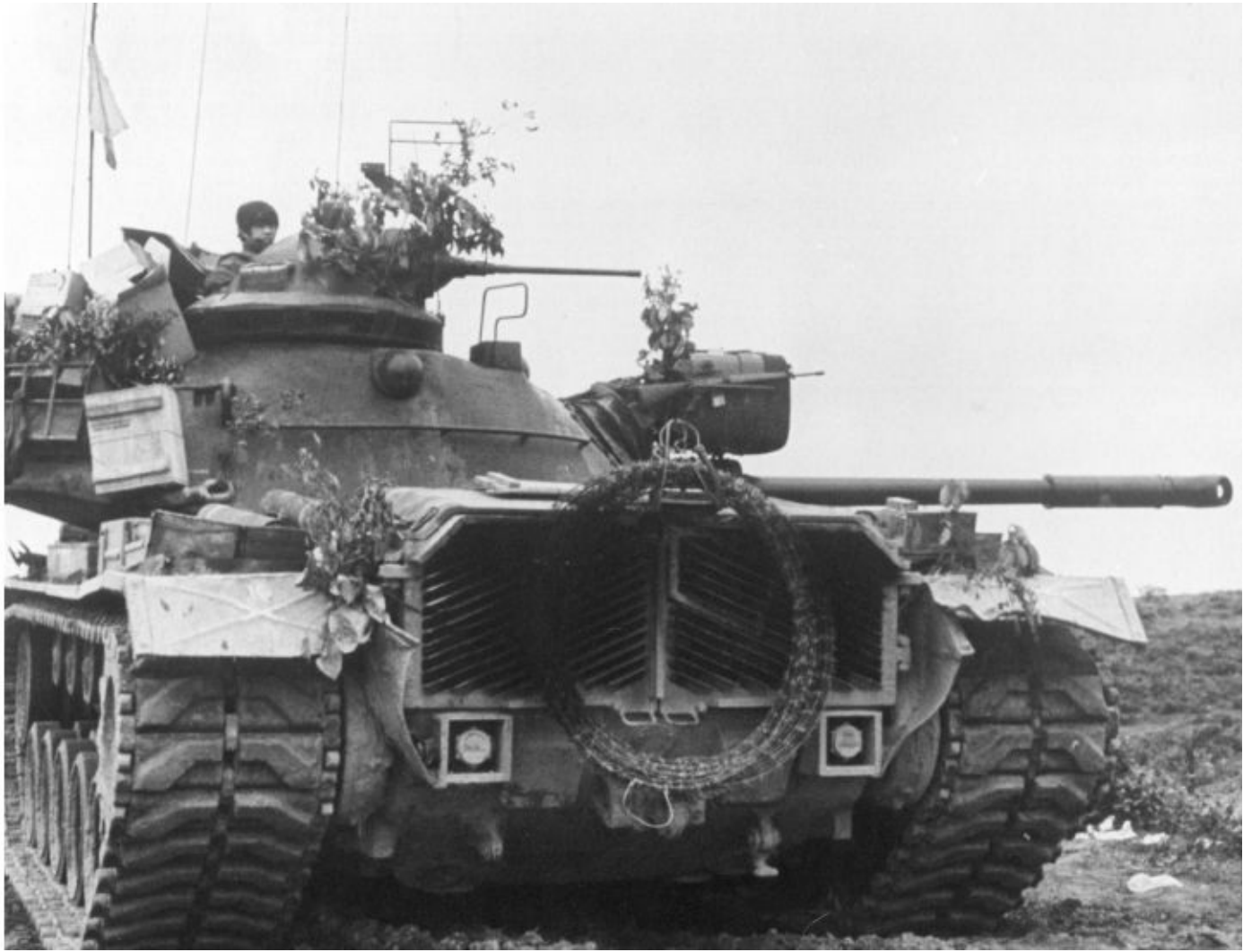
Here we see a late-production Army of the Republic of South Vietnam (ARVN) M48A3 (Mod B) tank. Besides the identifying feature of the squared brush guards around the rear taillights, the vehicle pictured also has the embossed “X” pattern on the rear fenders not seen on early-production M48A3 (Mod) B tanks. Patton Museum
