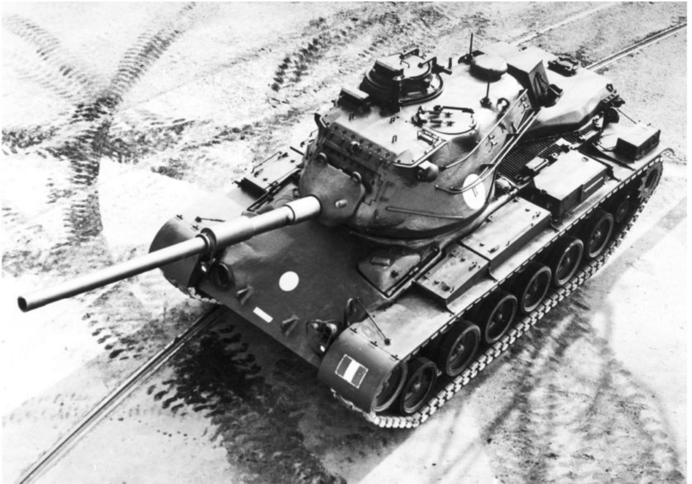
An overhead picture of an M47 tank upgraded with an M68 105mm main gun and a diesel engine by an Italian firm interested in drumming up business with countries that might wish to modernize their tank inventories. Patton Museum
