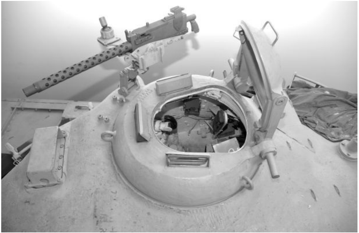
An overhead view of the Israeli-designed and built Urdan cupola on a Magach 3 tank. Directly in front of the cupola is the armored cover for the gunner's sighting periscope. The Urdan cupola is very similar to the Chrysler-designed low profile cupola that appeared on the original M48 tank. Chris Hughes
