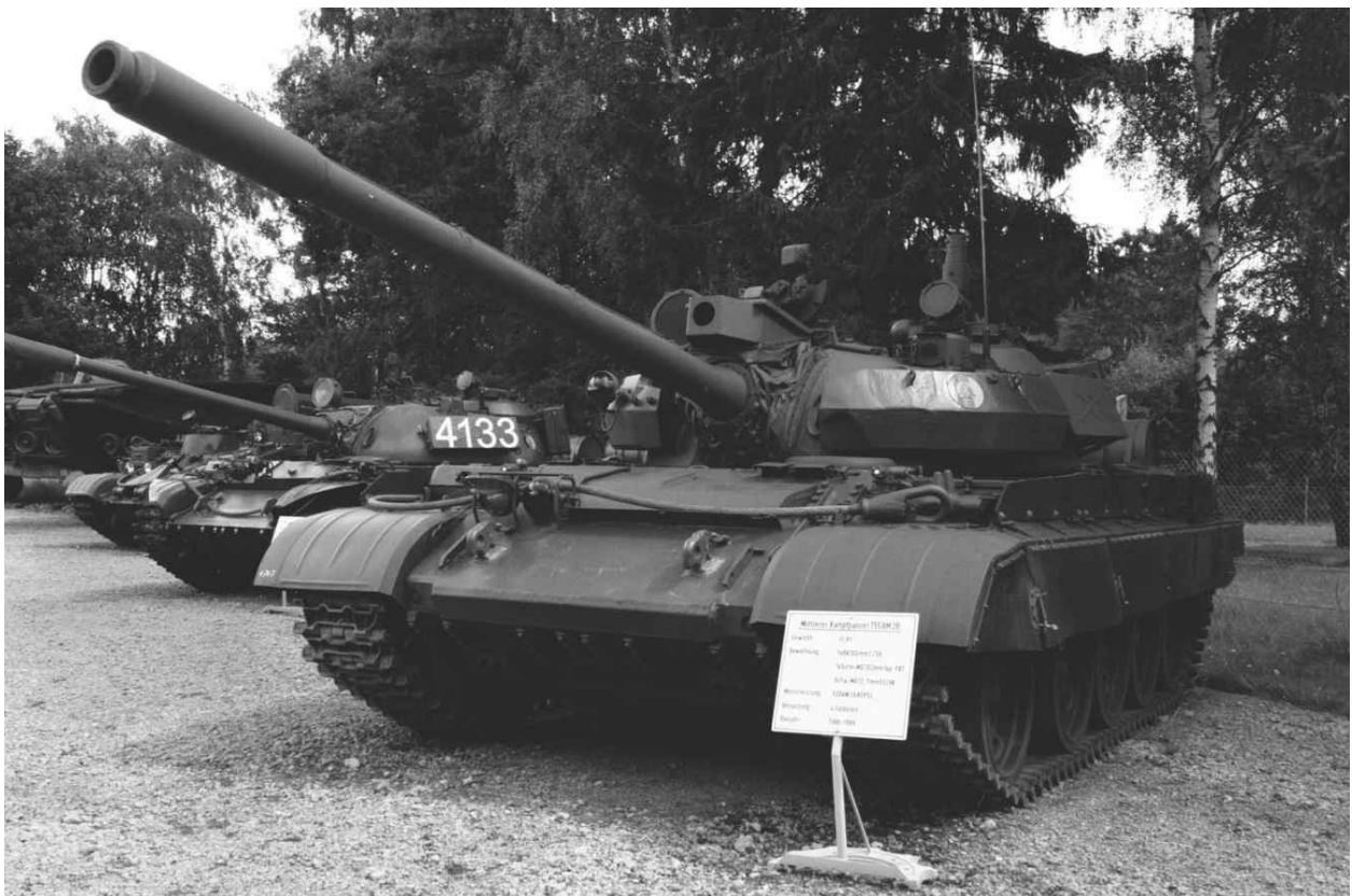
Polish-built East German T-55AM2B with reinforced glacis armour, turret brow armour and laser
