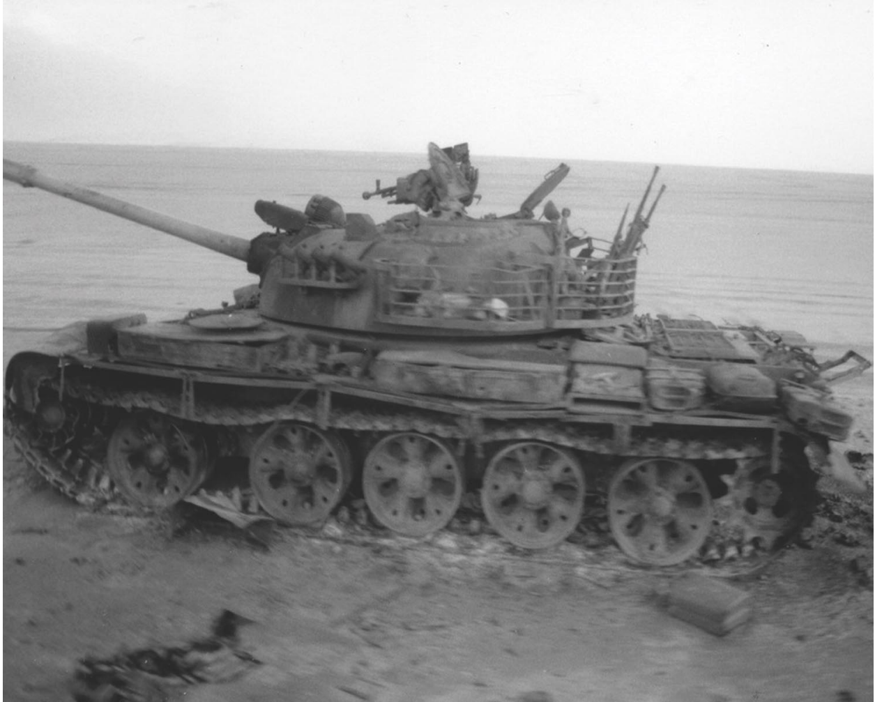
Remains of an abandoned Iraqi Type 69-II. It retains its turret 'boom shields' but not the side skirts.
