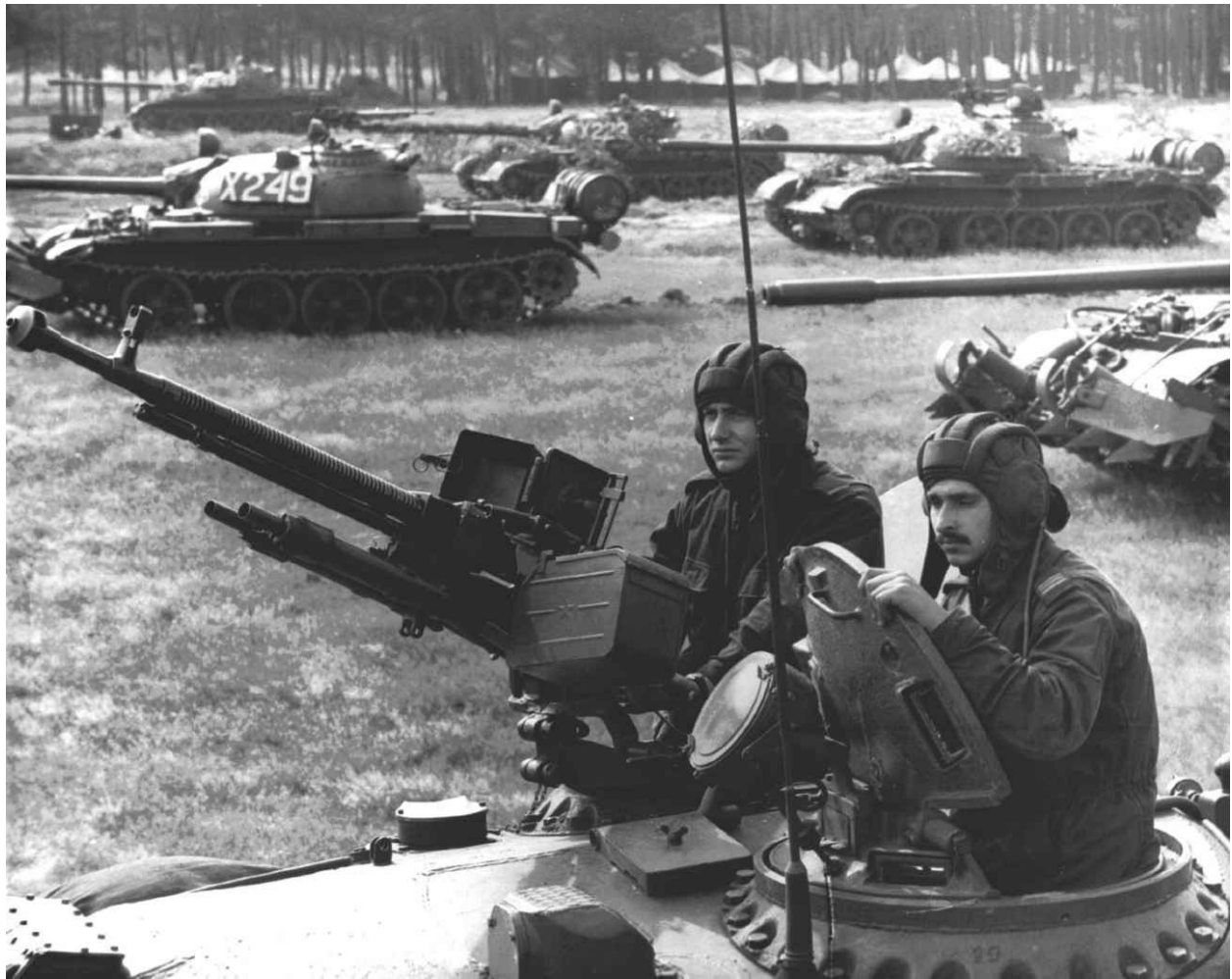
Polish T-55s. The loader is manning the 12.7mm DShKM anti-aircraft machine gun. Note the tank fitted with the mine plough just to the right.
