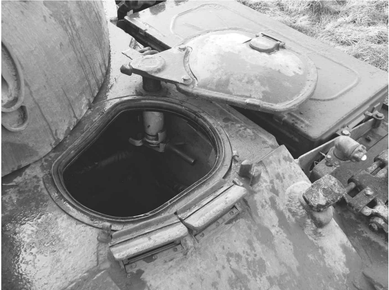
Driver's single-piece access hatch and twin periscopes.
