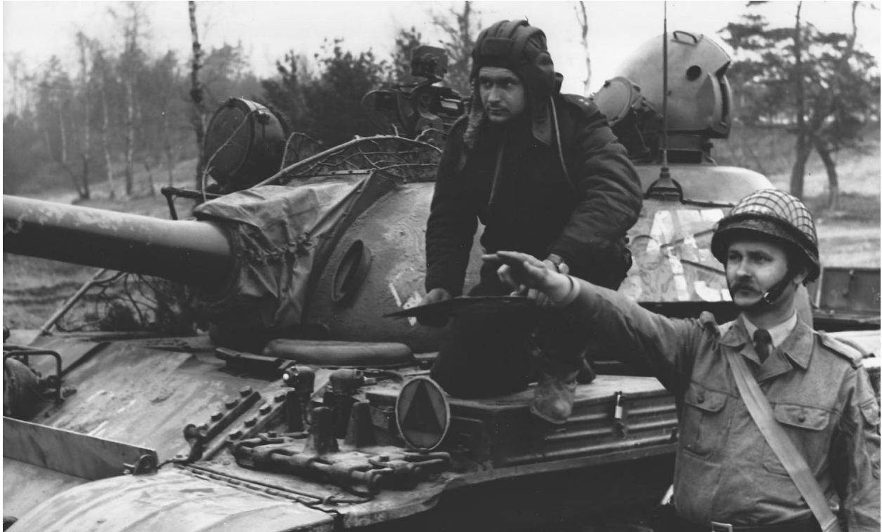
The gunner's sight opening on the turret of Polish and Czech-built tanks is much more oval than on its Soviet counterparts, as can be seen on this Polish T-55.
