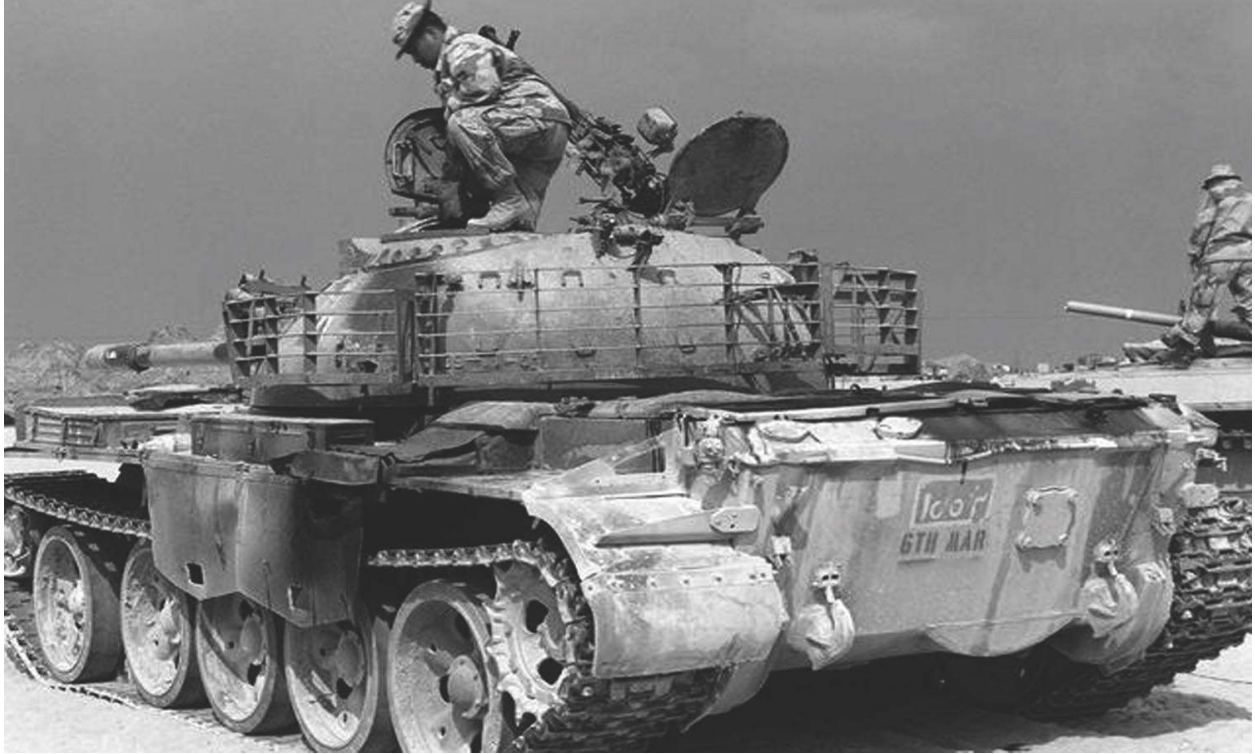
The rear of the same Iraqi Type 69-II. It has the distinctive semicircular edge on the bottom of the rear hull plate. This allowed for the new fan which was copied from the Soviet T-62. The basket frame around the turret was designed to thwart hollow charge weapons.
