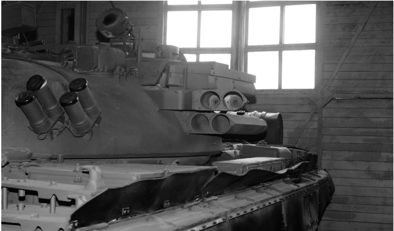
A T-55AD with the Drozd anti-missile system. This was the very first active protection system for a tank. The launcher fires a fragmentation warhead to destroy any incoming threat.
