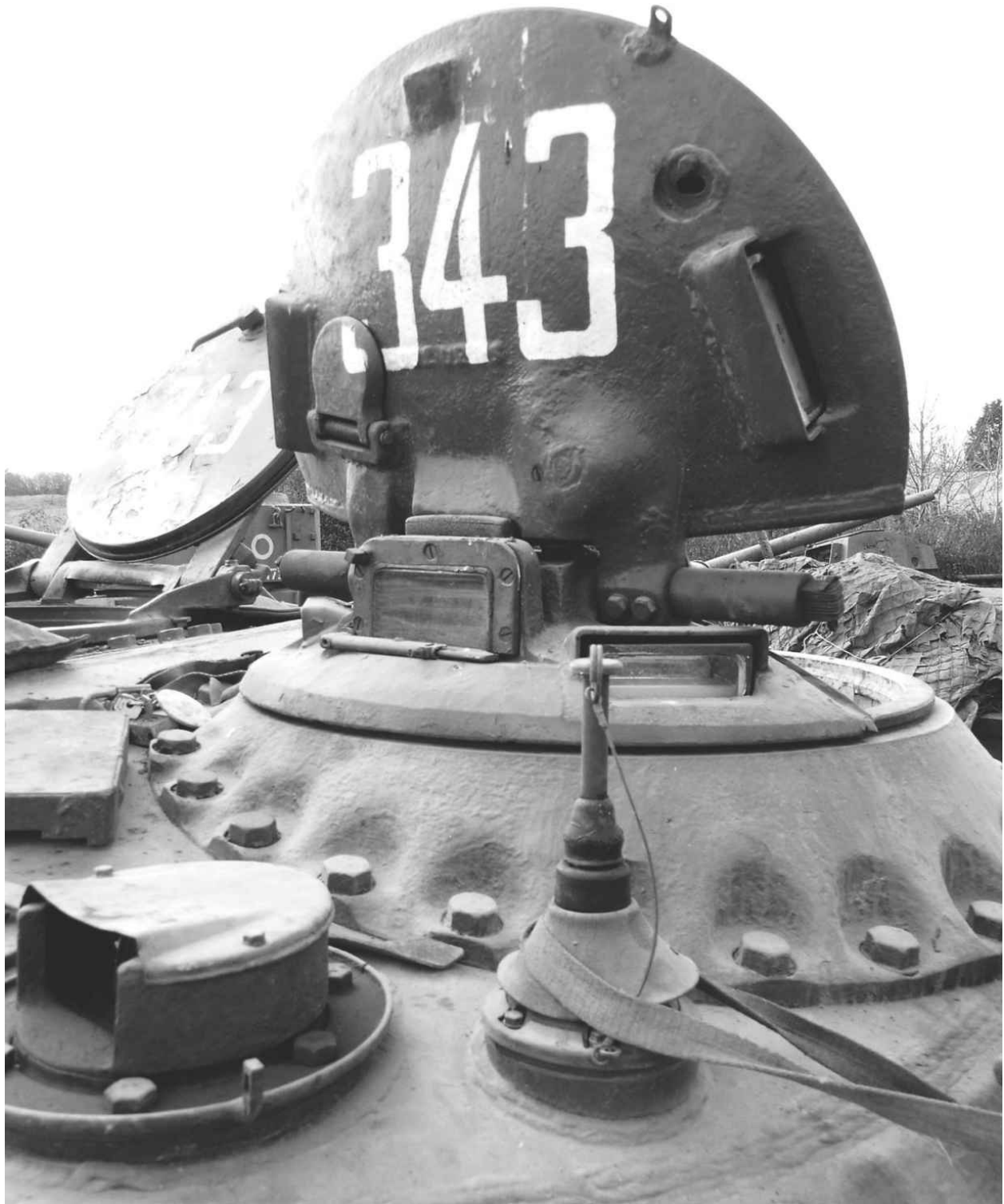
Bolted-on mounting for the commander's cupola and gunner's left-hand turret periscope. From the T-54B onwards the tank was equipped with the Luna night-fighting system. As part of this the gunner's MK-4 periscope was replaced with the TPN-1 night observation device.
