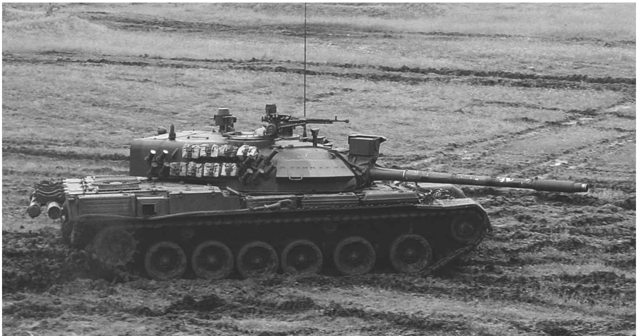
The modernized version of the TR-85, known as the M1, with redesigned turret and twin return rollers. It retained the 100mm gun. Very few of these upgrades were carried out.
