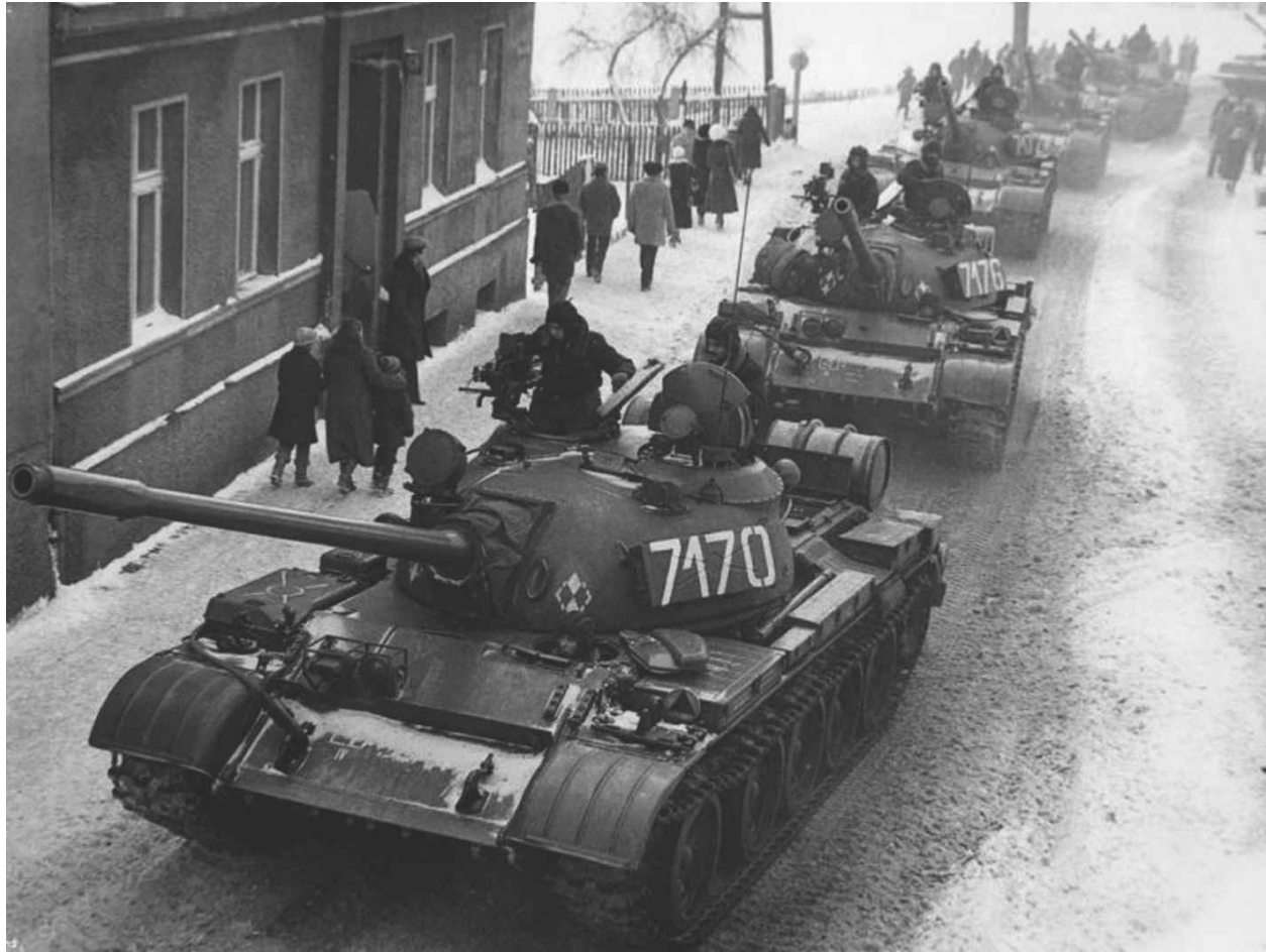
Polish T-55s. Note the very large storage box on the left side of the turret, this was a particular Polish feature. Another distinctive feature on the Polish T-55 is the prominent combing around the turret hatches which housed anti-radiation lining.
