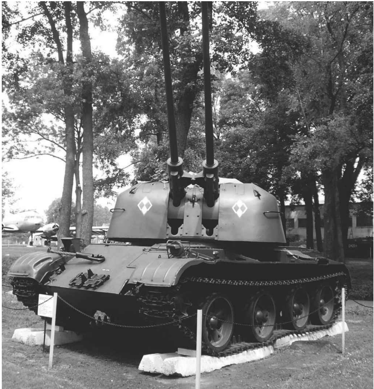
The ZSU-57-2 self-propelled anti-aircraft gun utilized a shorted T-54 chassis armed with twin 57mm guns. This only had four road wheels rather than the standard five.
