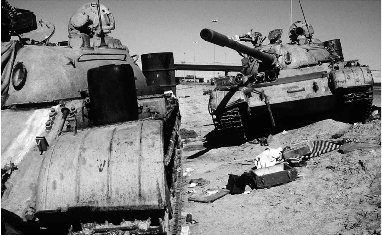
The same but not. Two Iraqi T-55s on the Basra-Kuwait Highway during the Gulf War. The one to the right is a Soviet Model 1970 with the anti-aircraft gun mount over the loader's hatch, while the one to the left is of Polish origin as it has the different-style gunner's aperture. The glacis marking on the second tank is a unit vehicle registration.
