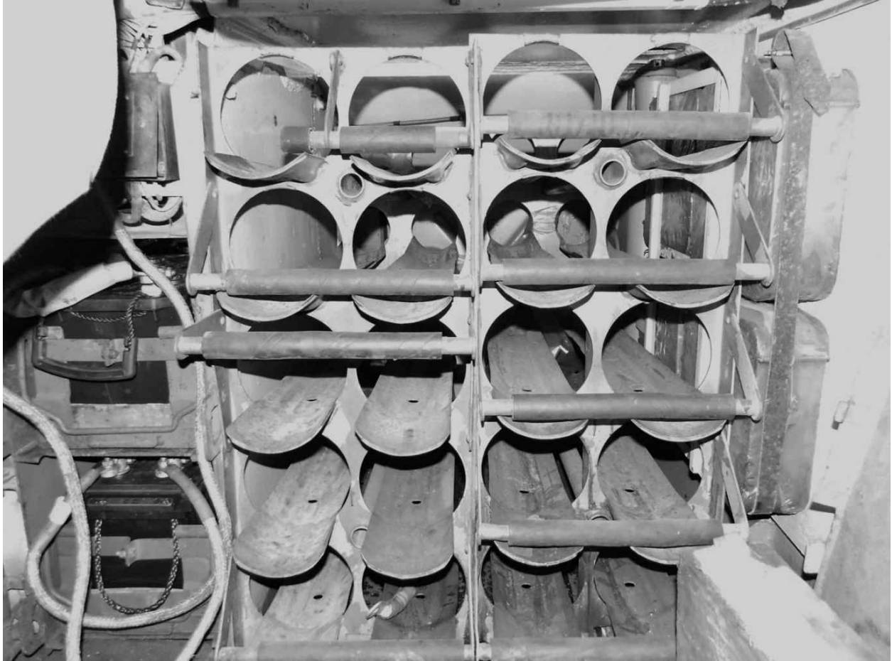
Close-up of one of the ammunition racks – the T-54 can carry a total of thirty-four 100mm rounds and the T-55 some forty-three rounds.
