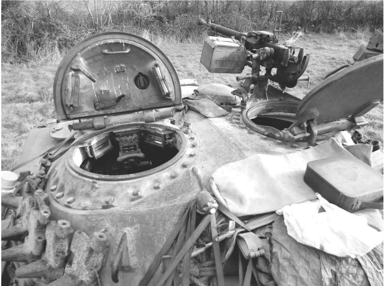
The commander's and the loader's hatches open in opposite directions. The commander's hatch on the left shows the cupola optics as well as the commander's sight.
