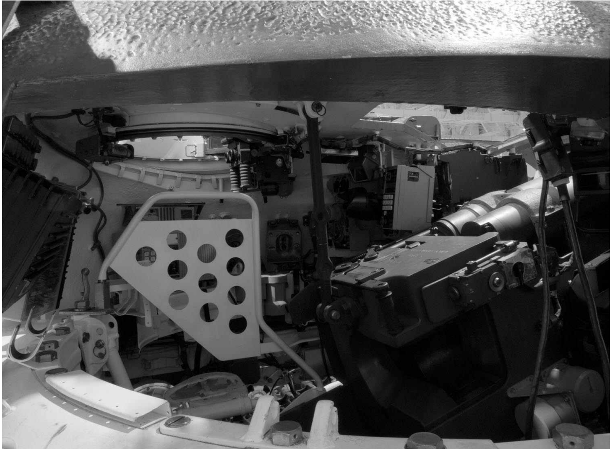
This training cutaway of a T-55 turret shows just how cramped the fighting compartment is. The commander, gunner, and loader all have to operate in this confined space.
