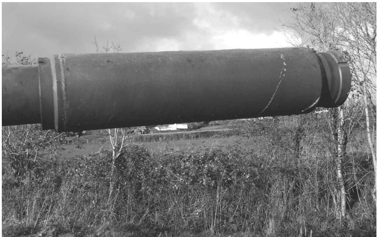
The 100mm D-10T gun fume extractor which is set back from the muzzle.
