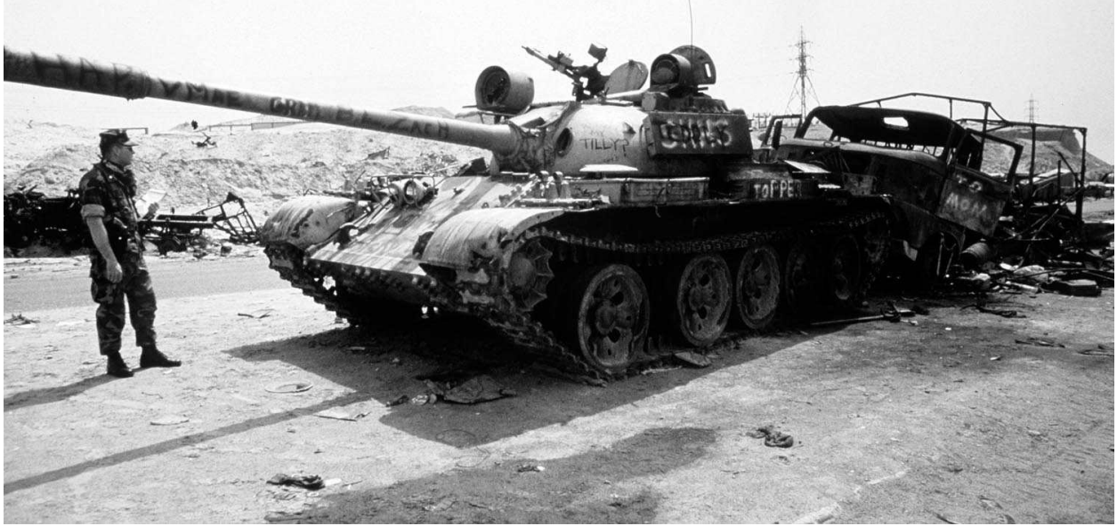
Polish-built T-55 belonging to the Iraqi Army lost on the Kuwait-Basra Highway in 1991. The loader's hatch is fitted with the anti-aircraft MG mounting. Its captors have daubed the whole tank in graffiti.
