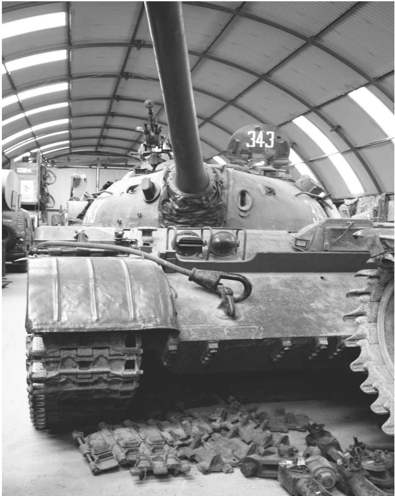
The narrow vertical plate running horizontally across the glacis is designed to stop water rushing up the front when fording shallow rivers and inundating the driver. The tiny hole just below it is the opening for the bow machine gun. The prominent mounting lugs welded to the lower nose plate are for attaching a dozer blade.
