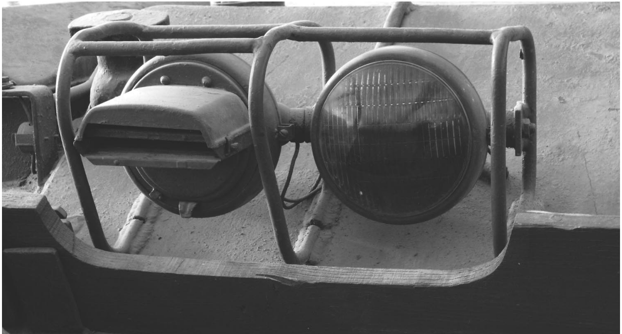
Headlights mounted in a protective frame on the right side of the glacis: one is restricted white light, the other infra-red.
