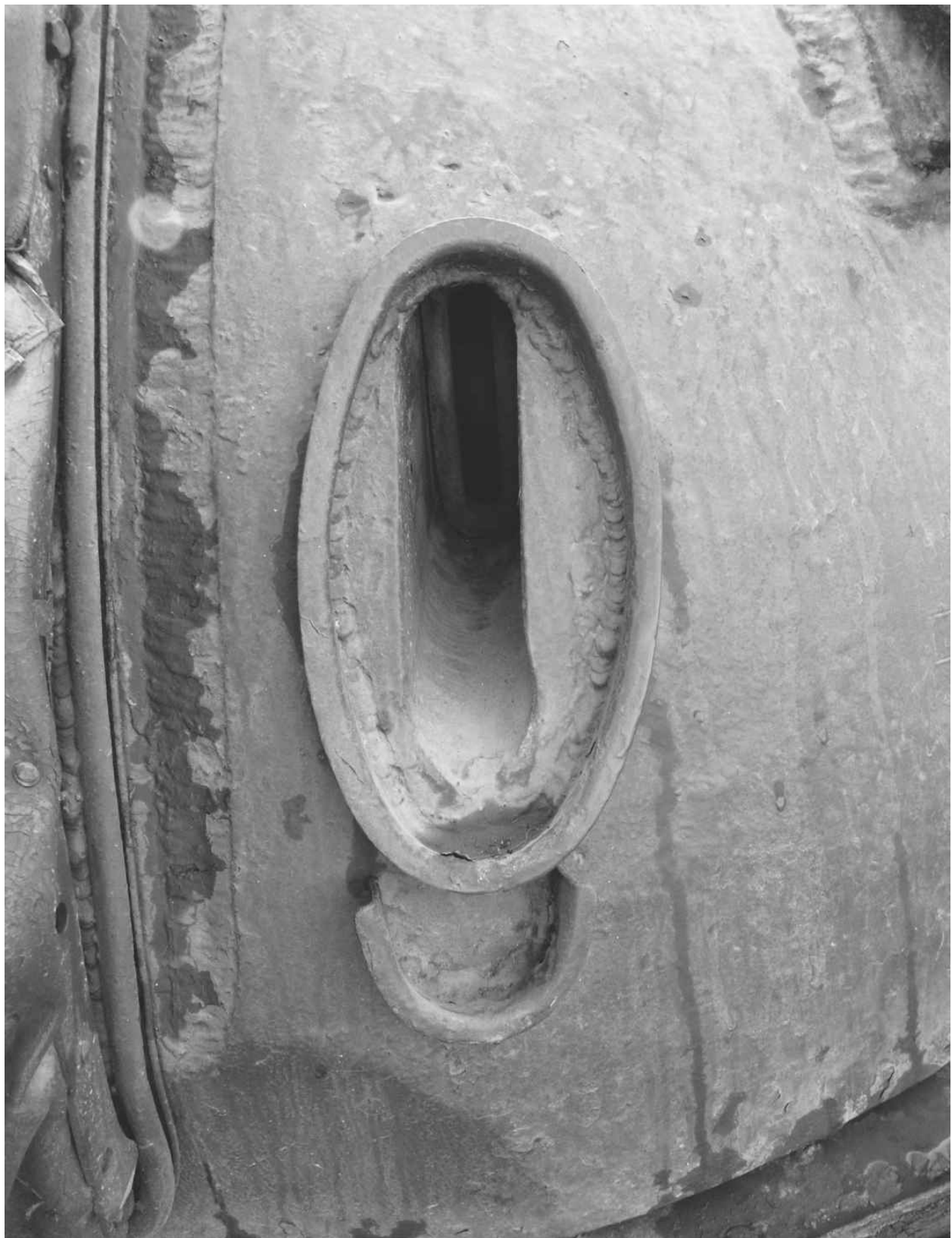
The oval cover fitting and lower bracket are welded to the turret. The latter does not appear on Polish-built T-54/55s.
