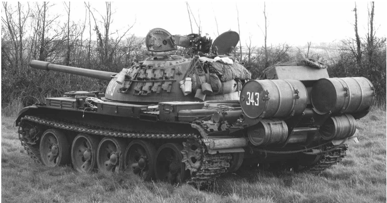
This Czech-built T-54 has its full complement of spare fuel tanks and smoke canisters. Limited internal space meant that when in the field equipment had to be stored on the outside of the tank as well. The narrow black oblong shape on the track guard just behind the long stowage bin is the exhaust outlet.
