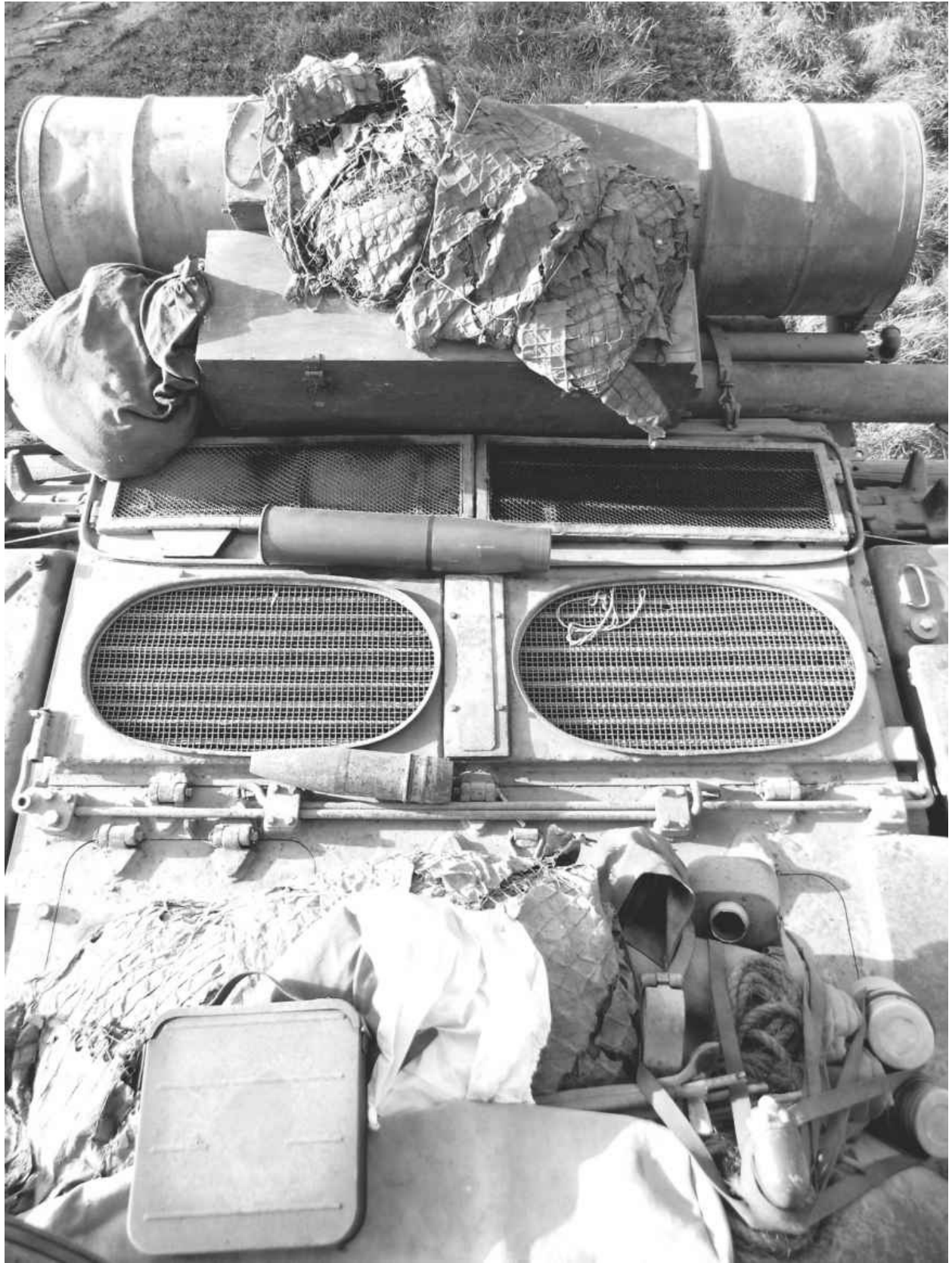
Rear engine deck showing the rectangular fan and rounded engine grills.
