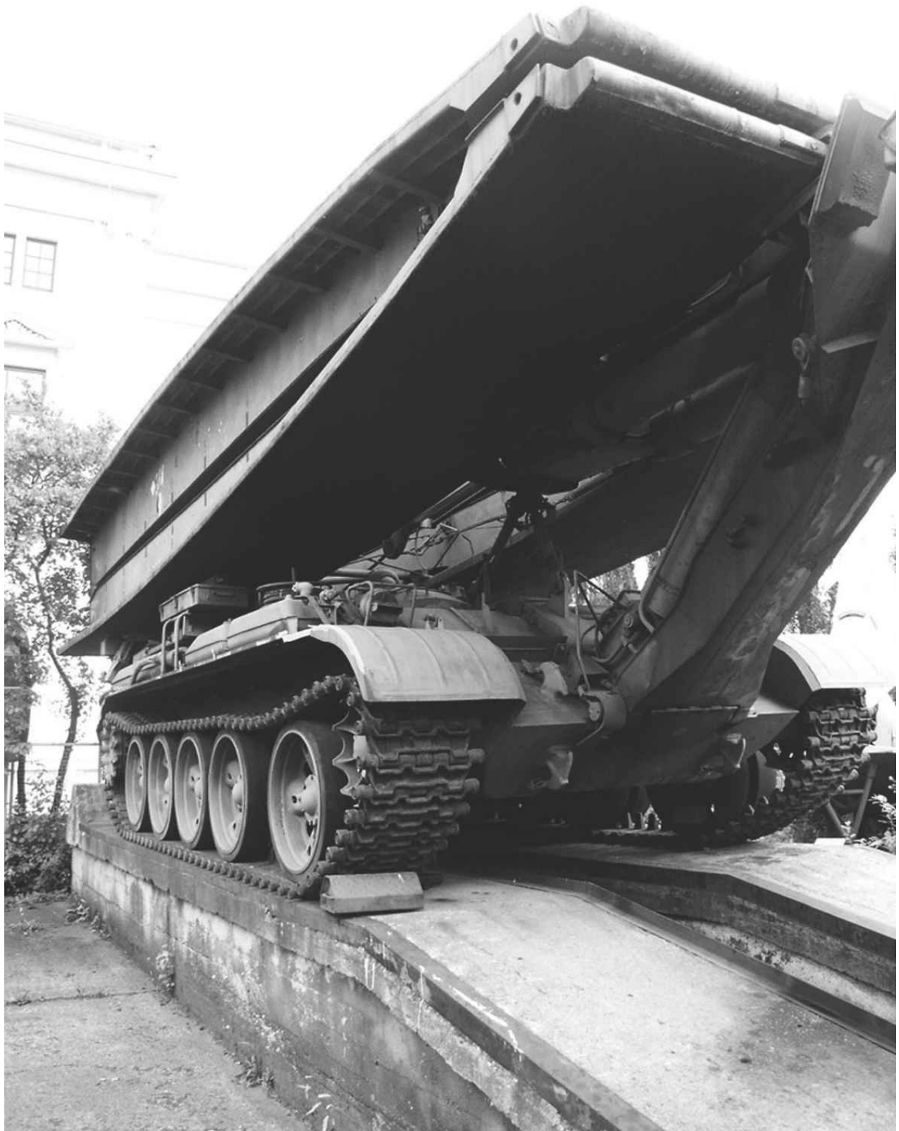
Front view of the MT-55 showing the electrohydraulic system used for launching the bridge into position.
