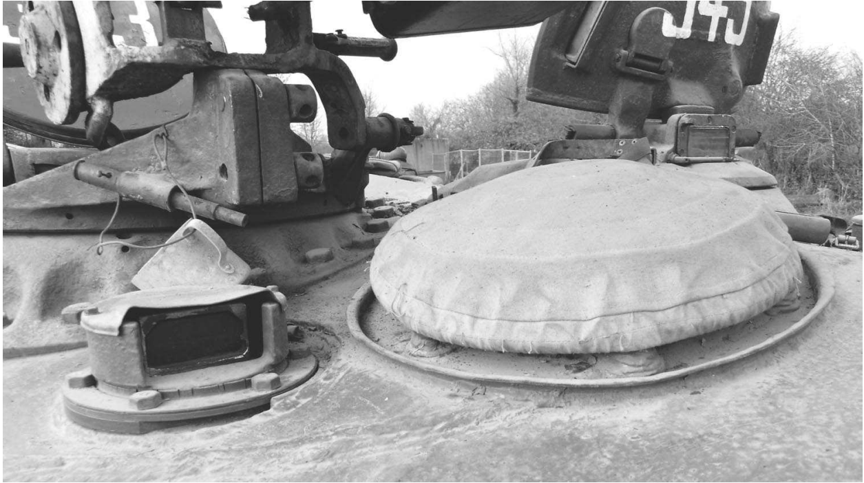
T-54 turret ventilator dome with rain cover, forward and to the left of the loader's hatch, and the loader's right-hand MK-4 turret periscope. The dome was omitted on the T-55 and is the easiest way to tell the two apart.
