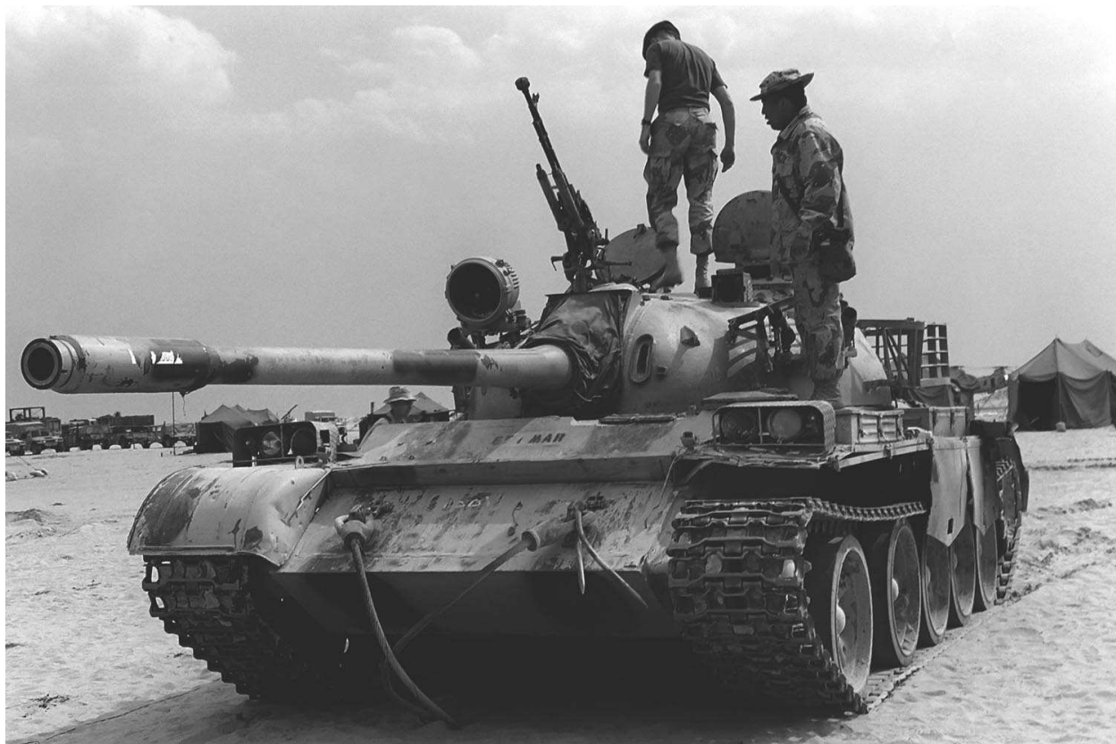
This Iraqi Type 69-II was captured during Desert Storm in 1991 by the US 6th Marines. It lacks its laser rangefinder over the main armament and the side skirts are damaged.
