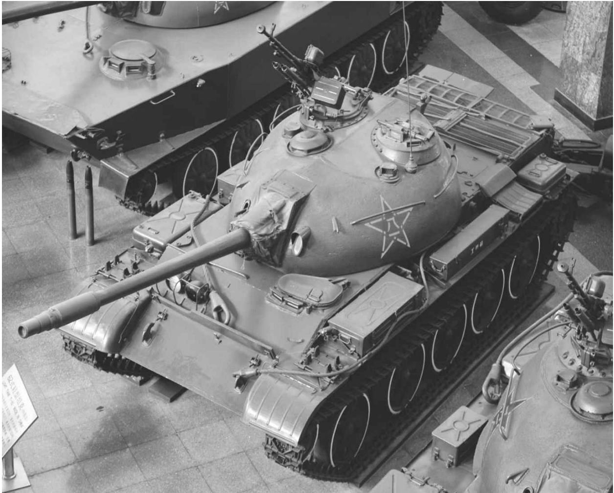
Like the Type 59, the Type 62 retained the T-54's turret ventilator dome and general layout.
