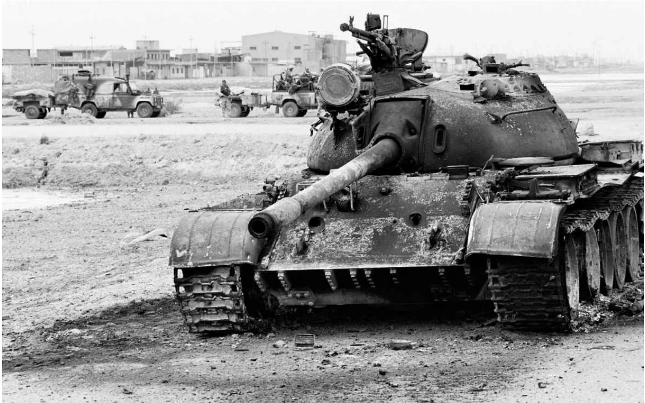
Completely burnt-out T-55 belonging to the Iraqi Army destroyed in 2003. The glacis plate has been pierced.
