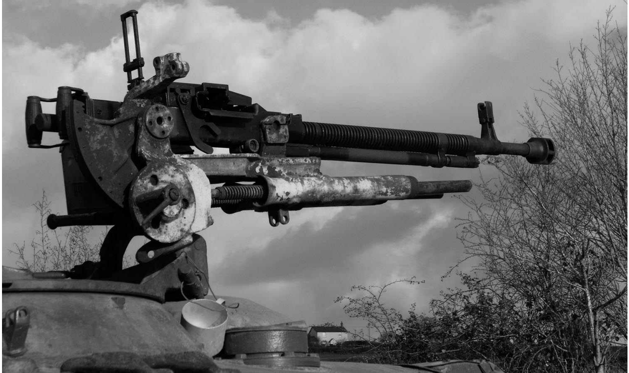
Two views of the anti-aircraft machine-gun mount fitted to the loader's hatch for the 12.7mm DShKM on both the T-54 and T-55. The two long objects just beneath the weapon are equilibrator tubes needed to balance it.
