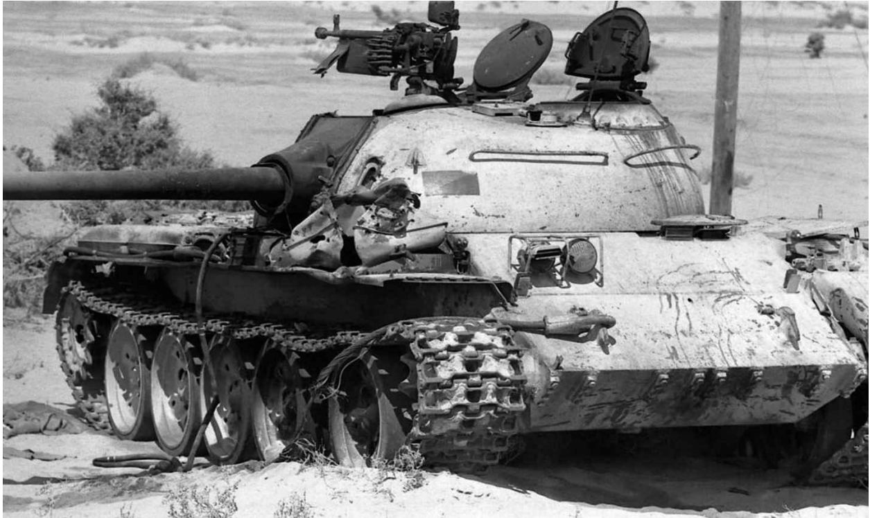
Knocked-out Egyptian T-54. It is painted in a very pale sand colour, and on the left-hand side of the turret is the traditional Egyptian red and green turret flash. The front external fuel tank has exploded.
