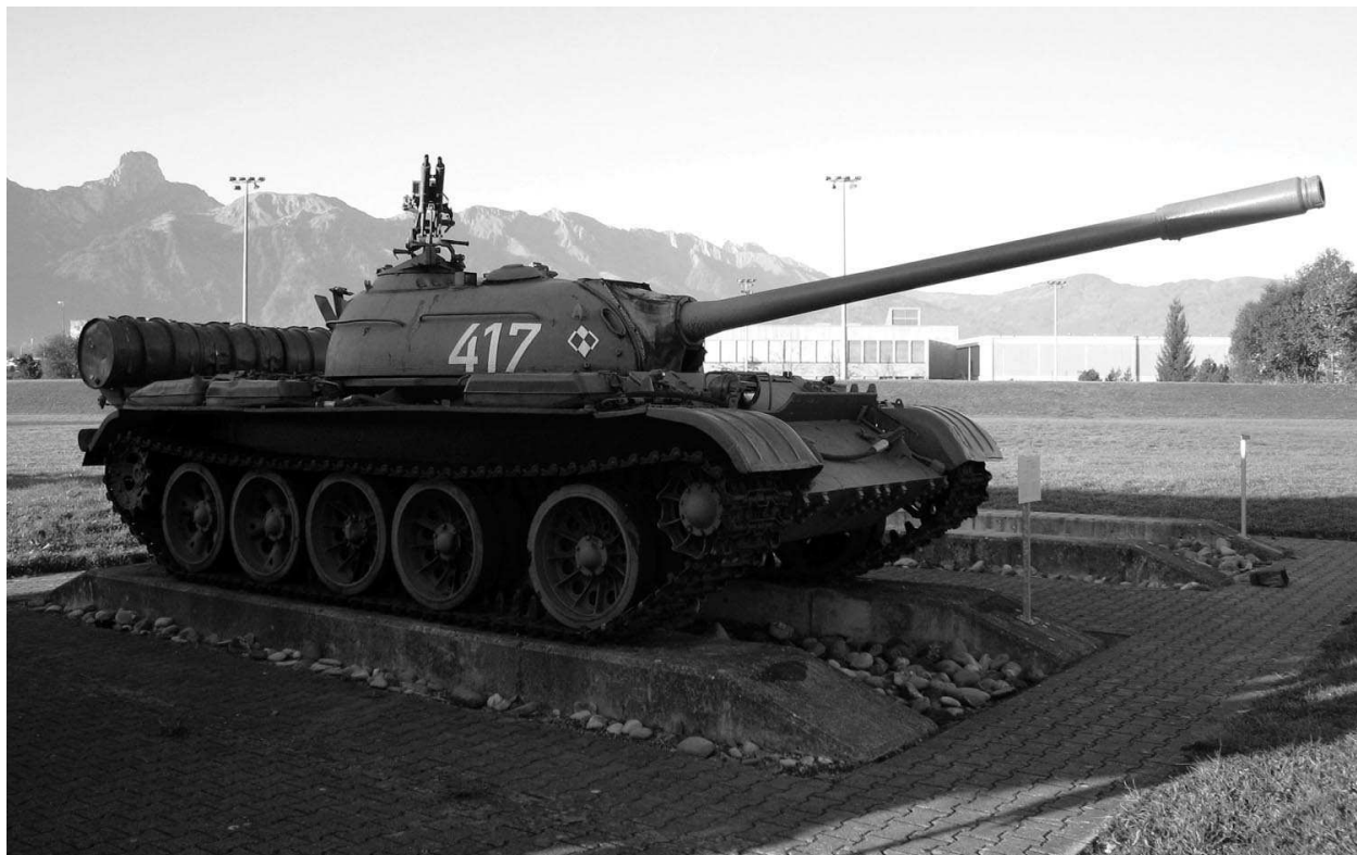
The T-54A or Model 1955 was the second full-rate production model and featured a distinctive fume extractor. It was also built by China, Czechoslovakia and Poland. This preserved example belonged to the Polish Army.
