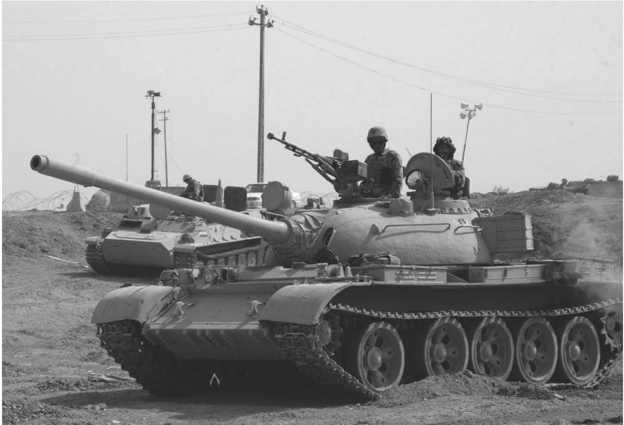
Refurbished Iraqi Army T-55 (it clearly lacks the loader's cupola and ventilator dome), following operation Iraqi Freedom. The back of the turret has been uparmoured and it retains its infra-red lamps, but the laser rangefinder is missing. The smoke is from the exhaust cowl just to the rear of the long stowage bin.
