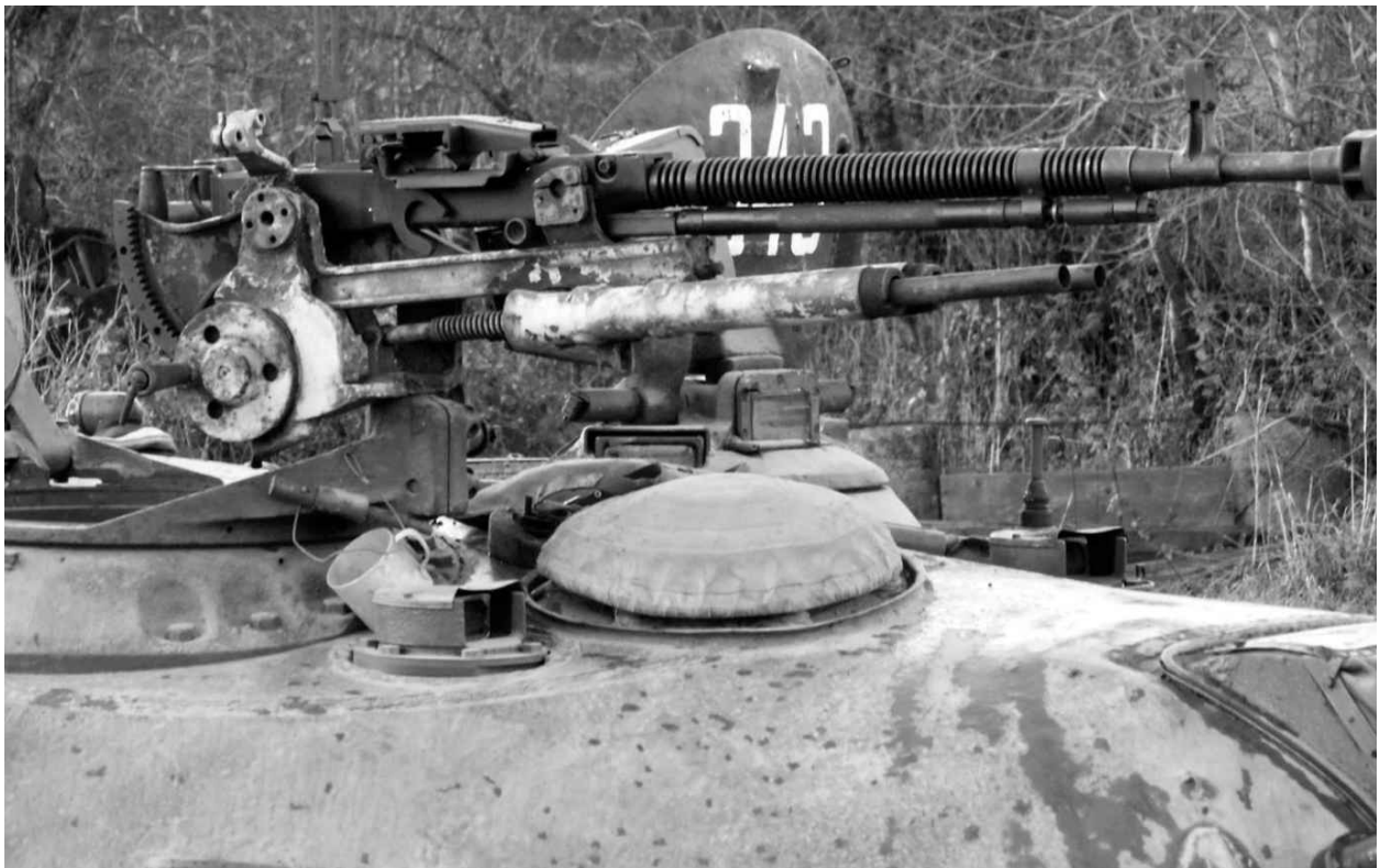
Two views of the anti-aircraft machine-gun mount fitted to the loader's hatch for the 12.7mm DShKM on both the T-54 and T-55. The two long objects just beneath the weapon are equilibrator tubes needed to balance it.
