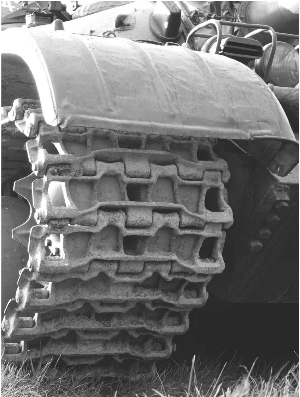
The T-54/55 track shoes are held together by dry pins.
