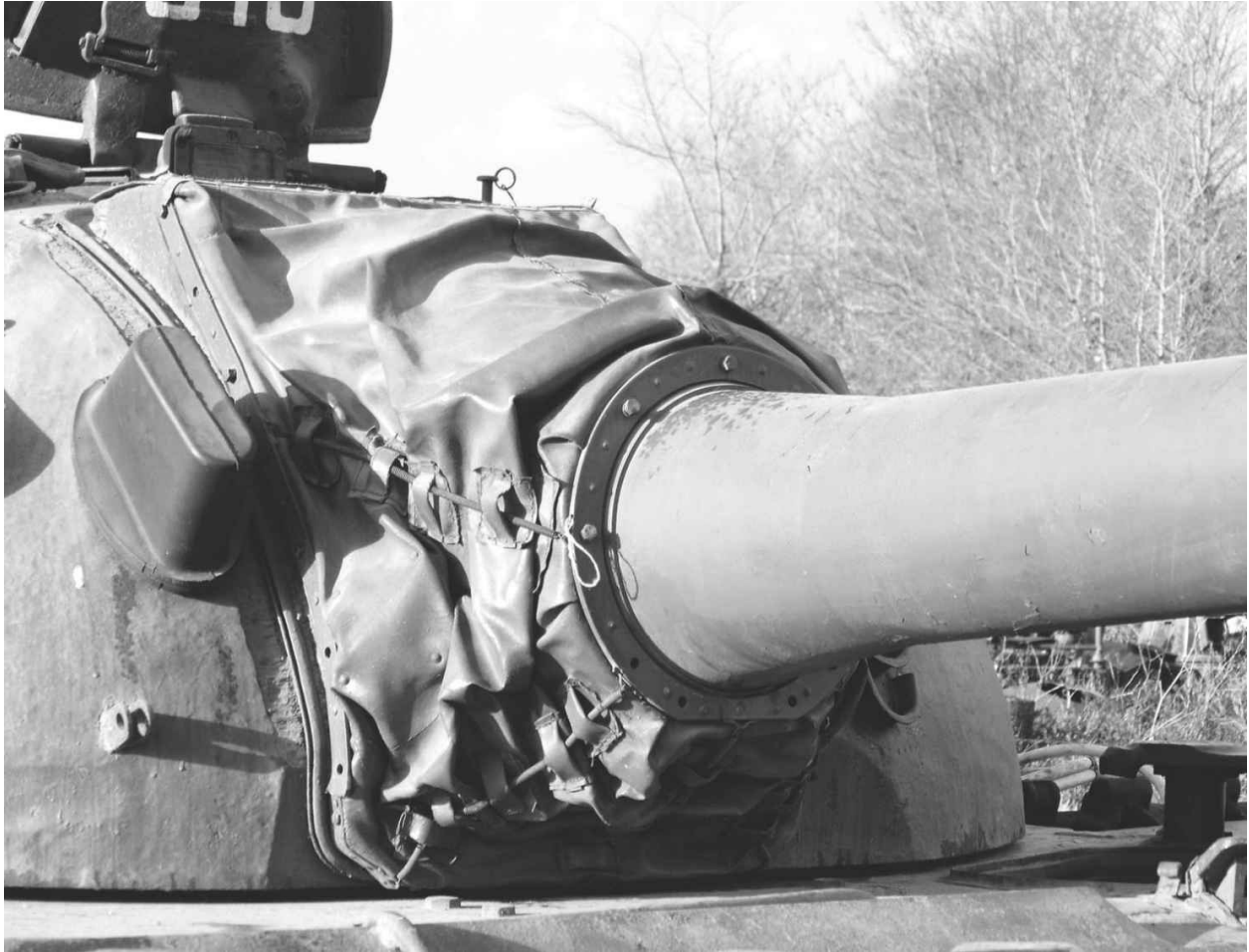
Close-up of the main armament mantlet NBC/rain cover and the coaxial machine gun opening cover.
