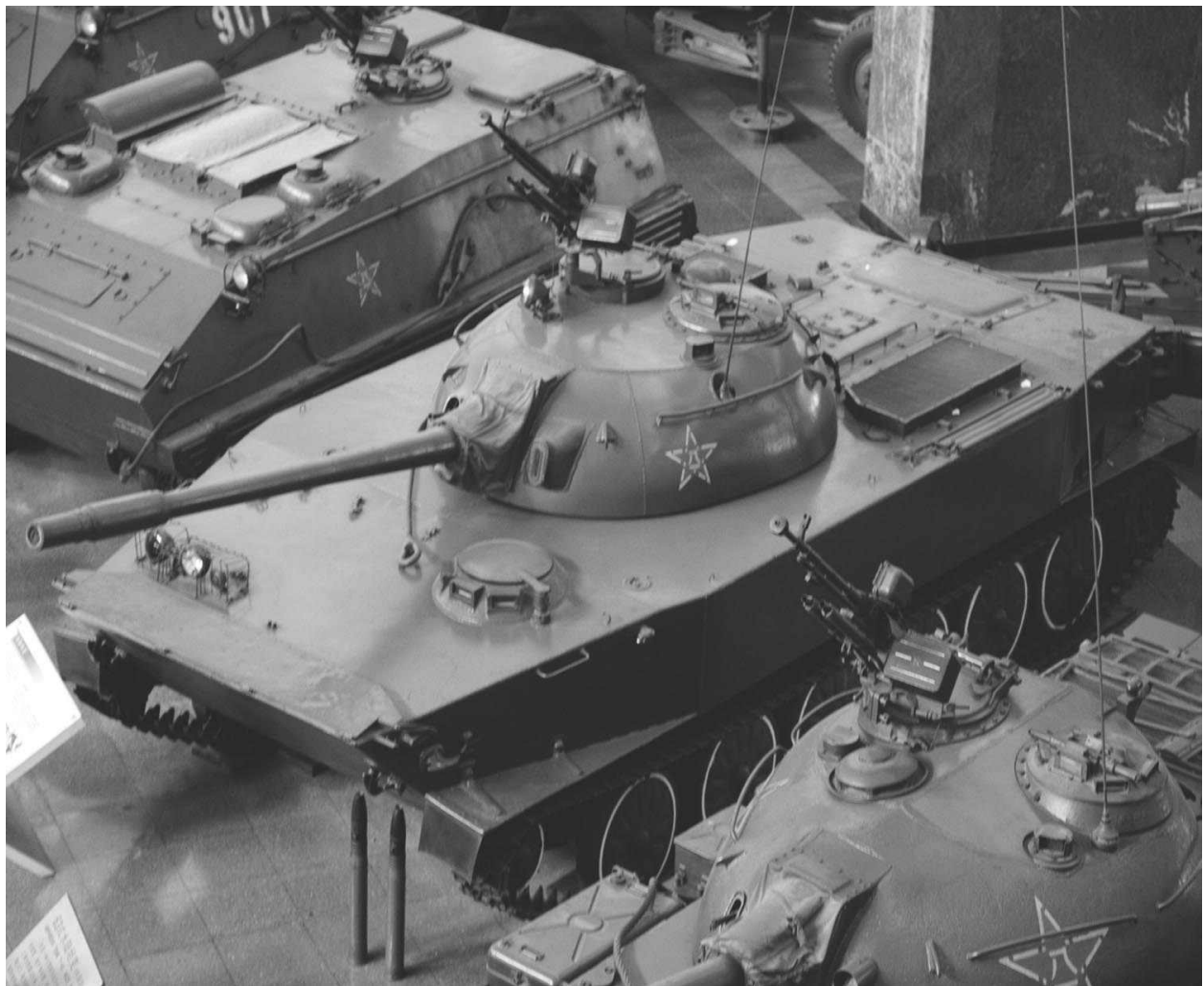
The Type 63 hull and chassis was based on the Soviet PT-76. Note the smaller turret hatch mountings compared to the Type 62 to the right.
