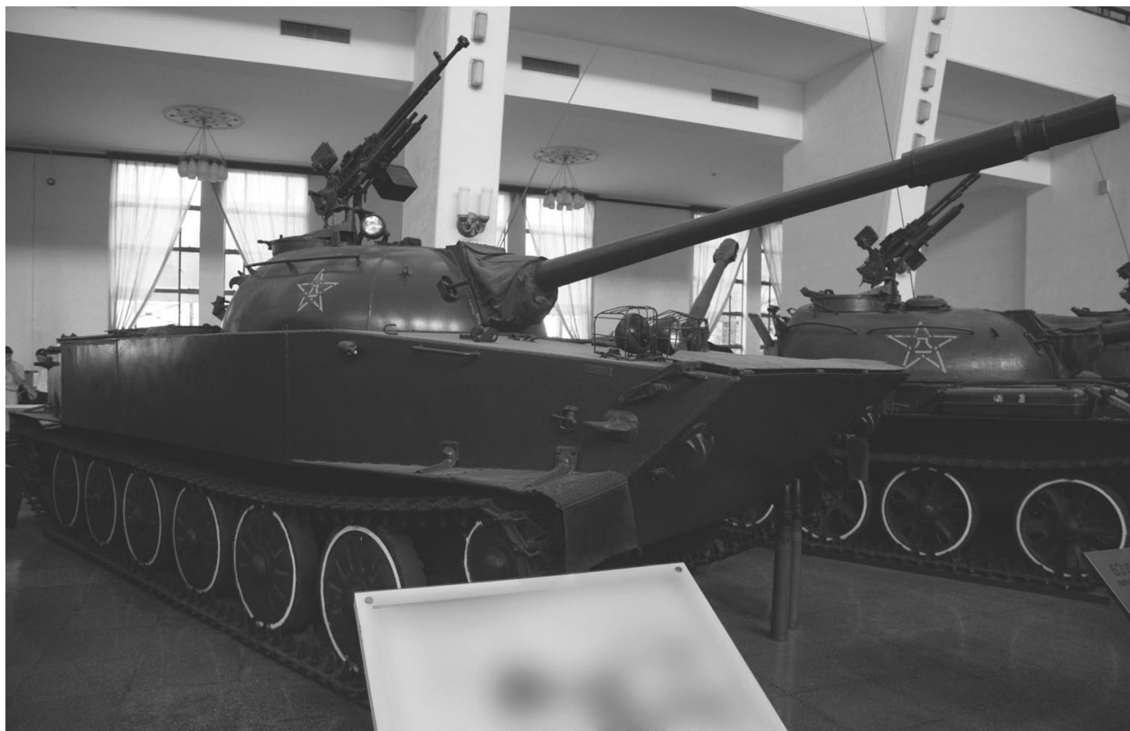
The Chinese Type 63 light amphibious tank used a turret similar to the Type 62, but with a flatter roof, no ventilator dome and single handrails either side.
