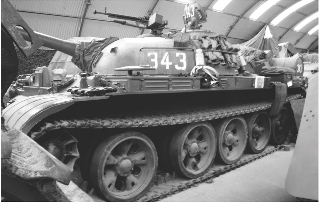
The T-54/55 has a distinct gap between the first and second road wheels. On the right-hand side above the track guards there are three external armoured fuel tanks. On the left are three to four stowage bins for tools and the exhaust outlet.
