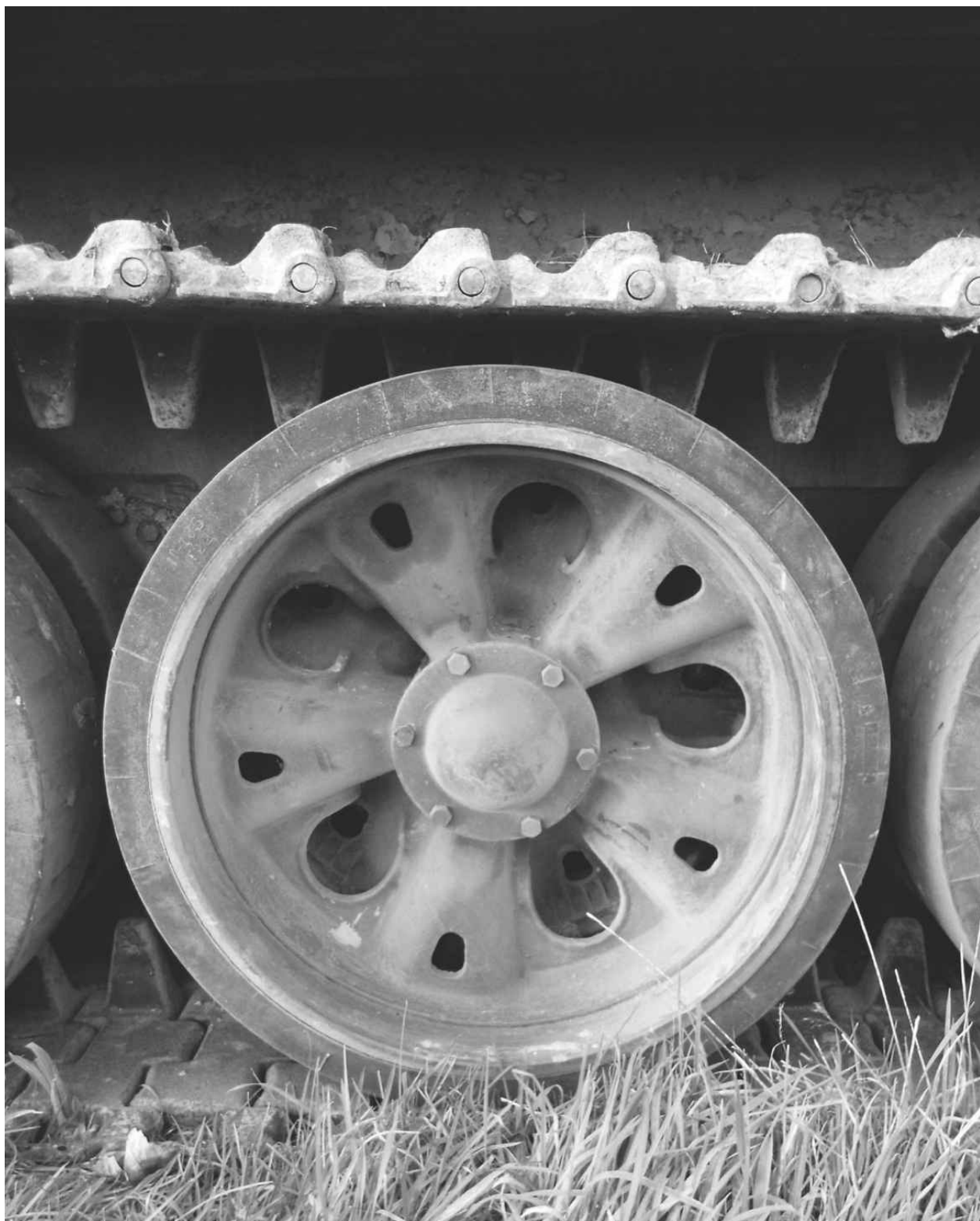
Typical cast double road wheel. These are the later starfish design that replaced the T-34-style spider wheels.
