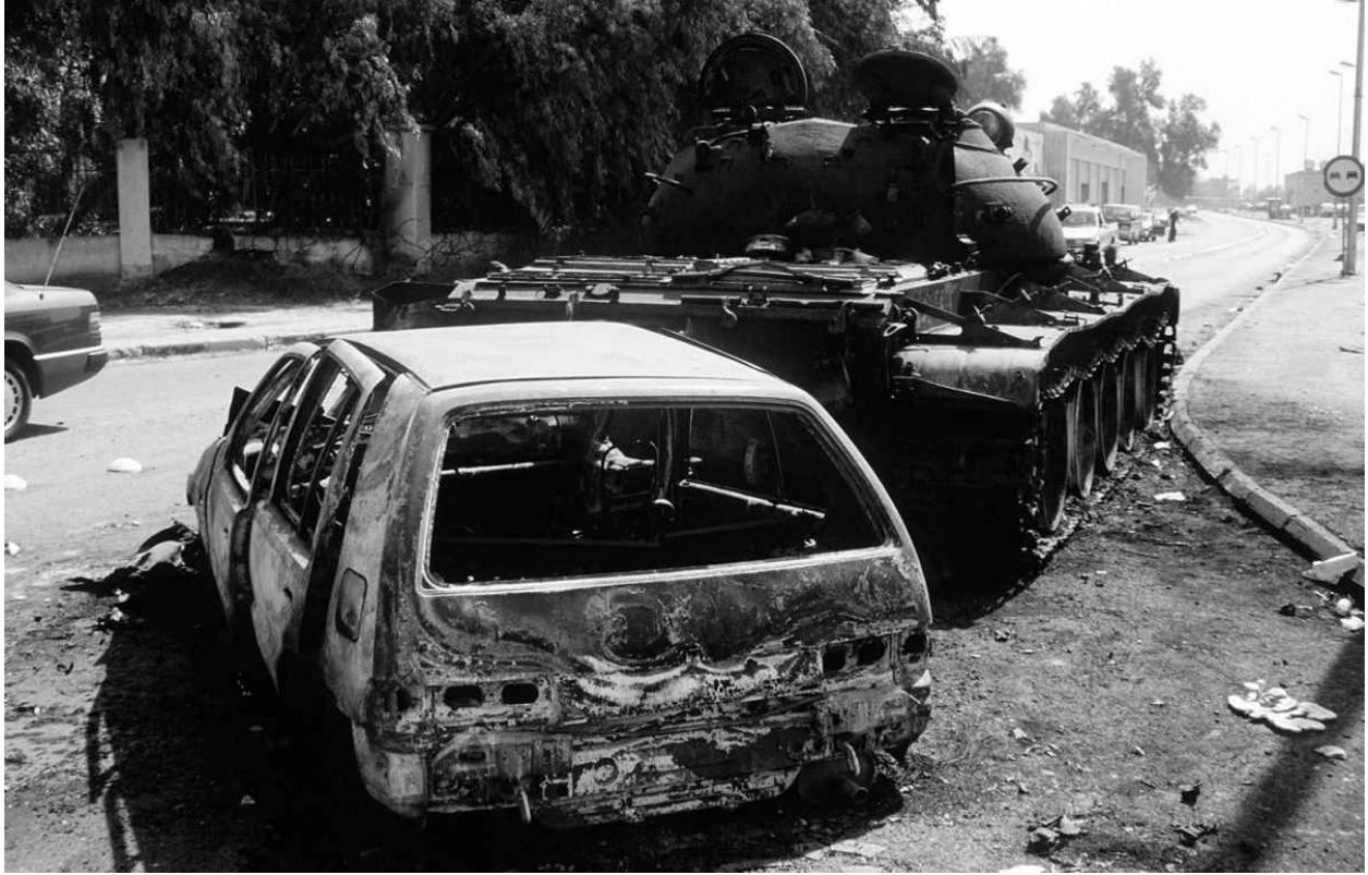
Burned-out Iraqi T-55 on the outskirts of Kuwait City. The rubber tyres on the road wheels have melted in the heat of the fire.
