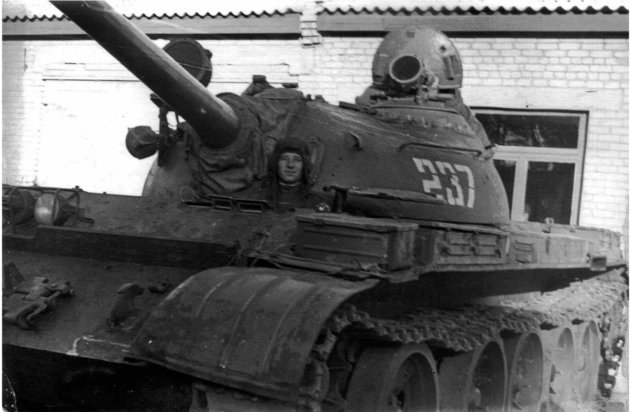
Early T-54 with the spider wheels. It is also fitted with infrared searchlights introduced with the T-54B, but no laser rangefinder.
