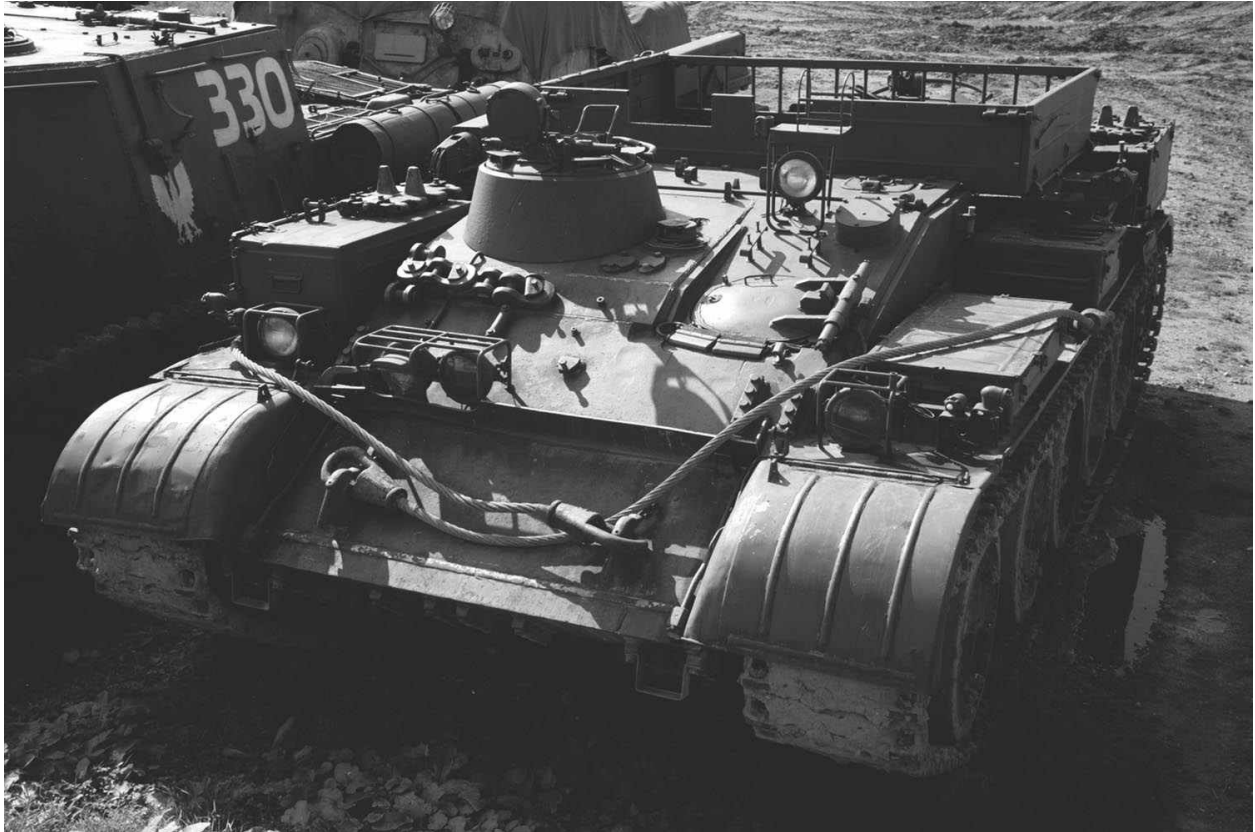
Czechoslovak VT-55A ARV – this example is missing its dozer blade. It is based on the T-55A MBT chassis while an earlier Czech version, the MT-55, drew on the T-55-T ARV.
