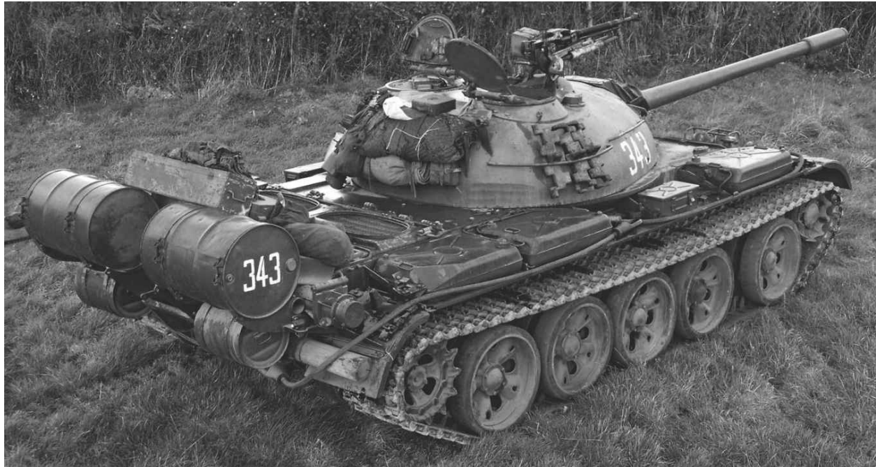
This shot shows the three external armoured fuel tanks fitted on the right-hand side of the tank, as well as the rear-mounted external 200-litre fuel drums. on the Polish version of the T-54A additional fuel cells were also positioned either side of the turret ring.
