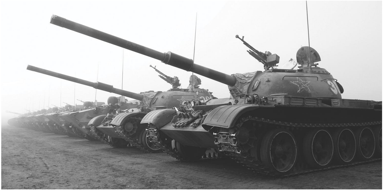
Type 59-IIs armed with 105mm guns. Although the mid-barrel fume extractor is clearly visible these examples do not have thermal sleeves. In 1991 Saddam Hussein ordered up to 600 Type 59s for the Iraqi Army.
