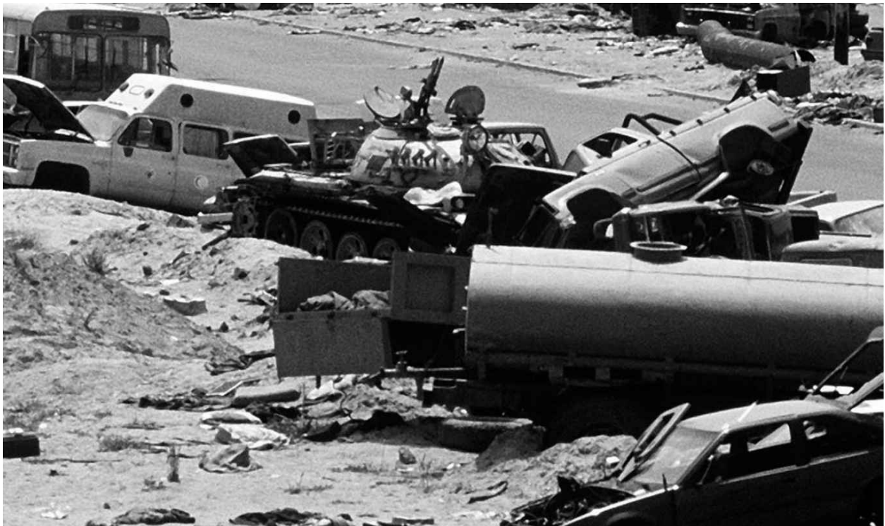
The same but not. Two Iraqi T-55s on the Basra-Kuwait Highway during the Gulf War. The one to the right is a Soviet Model 1970 with the anti-aircraft gun mount over the loader's hatch, while the one to the left is of Polish origin as it has the different-style gunner's aperture. The glacis marking on the second tank is a unit vehicle registration.
