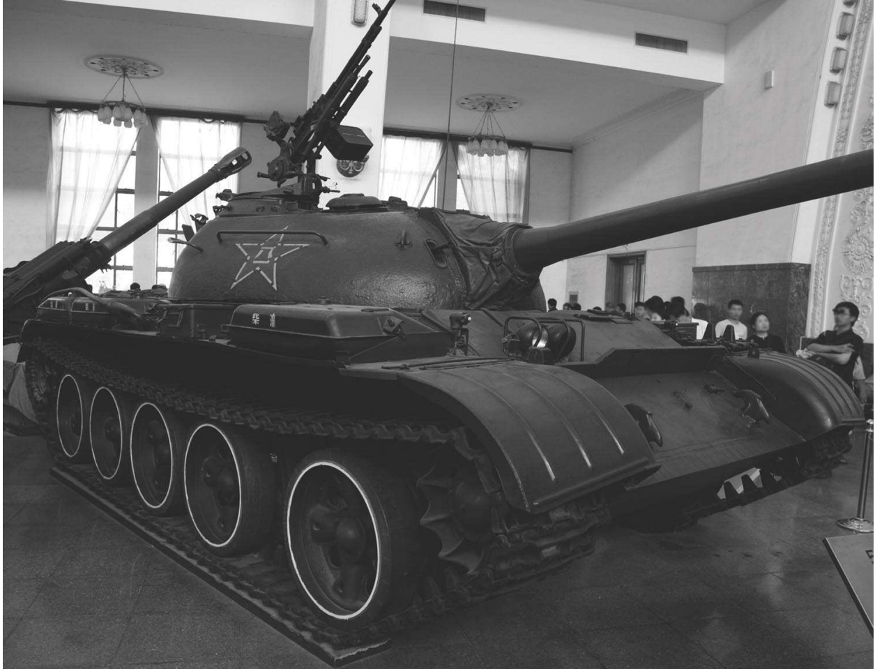
The Chinese subsequently copied the T-54, producing their Type 59/69 MBTs. The initial Type 59, seen here, was essentially the same as the T-54A, while the Type 59-I featured some internal changes and was fitted with a laser rangefinder.
