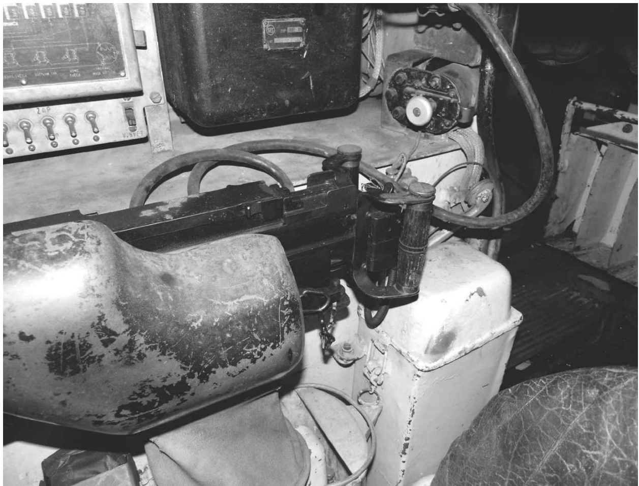
The automatically-operated bow machine gun situated just to the right of the driver. This fires through a small hole in the glacis plate.
