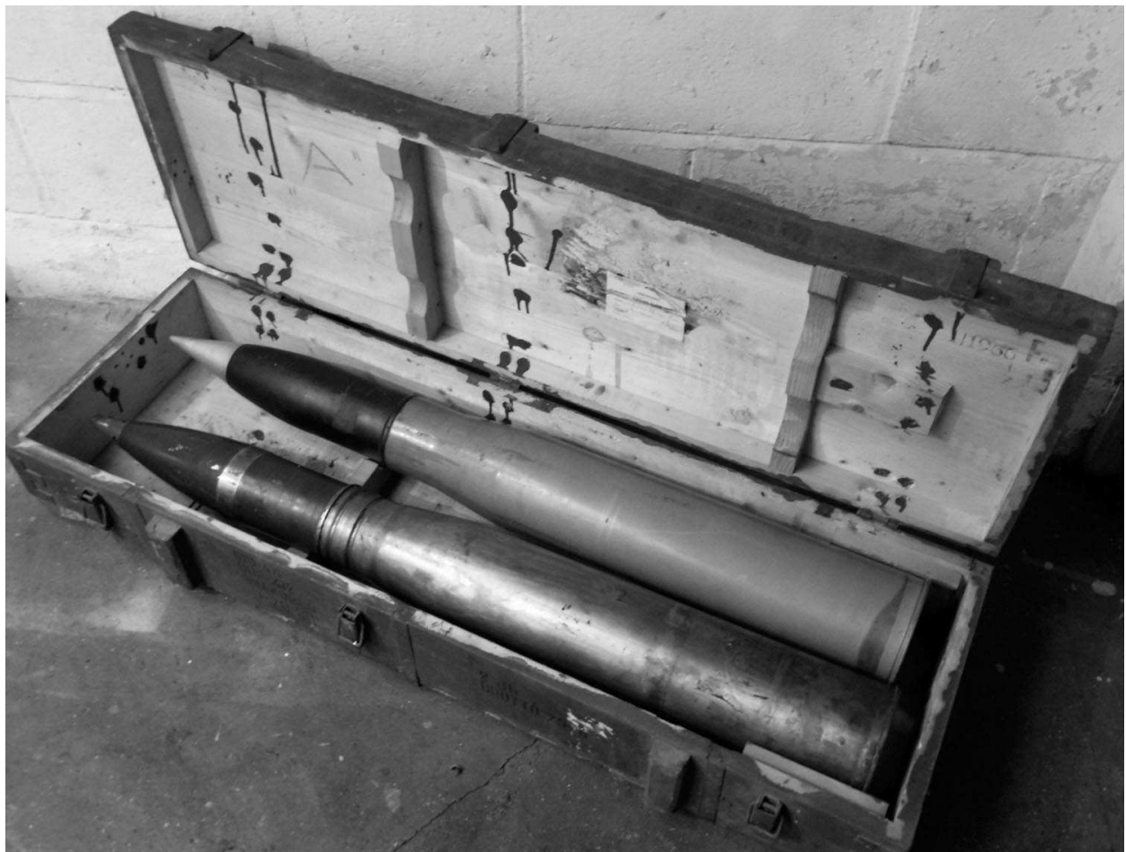
Two types of 109cm long 100-44 D-10 tank gun drill rounds. The first has a brass outer casing with solid steel warhead, the other steel with wood.
