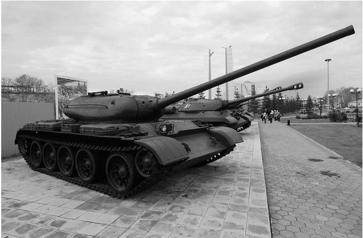
This preserved T-54-1 retains the original spider wheels.
