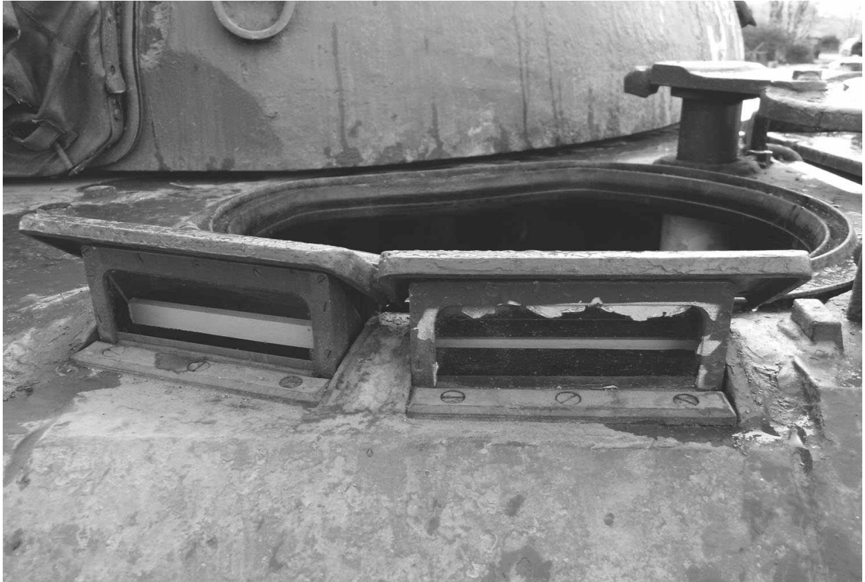
Driver's periscopes. One of these can be substituted for an infra-red periscope to be used with the infra-red light mounted on the right side of the glacis plate.
