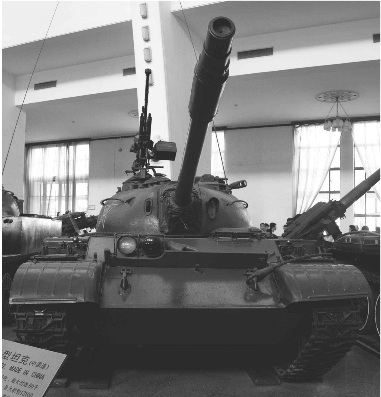
The Type 62 light tank was a scaled-down, lighter version of the Type 59 armed with an 85mm gun, which had a much shorter barrel.
