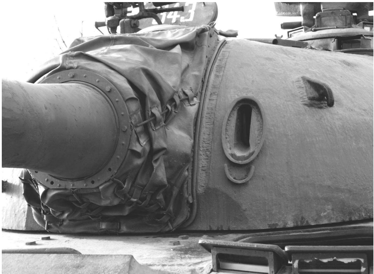
The turret on this Czech-built T-54 also has the distinctive cast oval cover fitting round the gunner's sight aperture plus a lower bracket.
