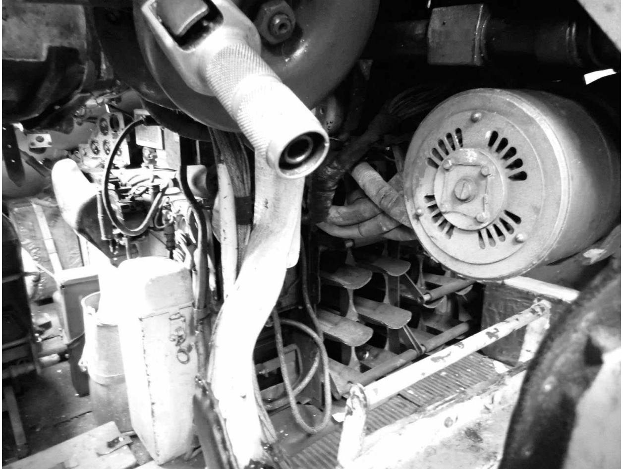
One of the main armament ammunition racks is located just to the right of the driver and the bow machine gun.
