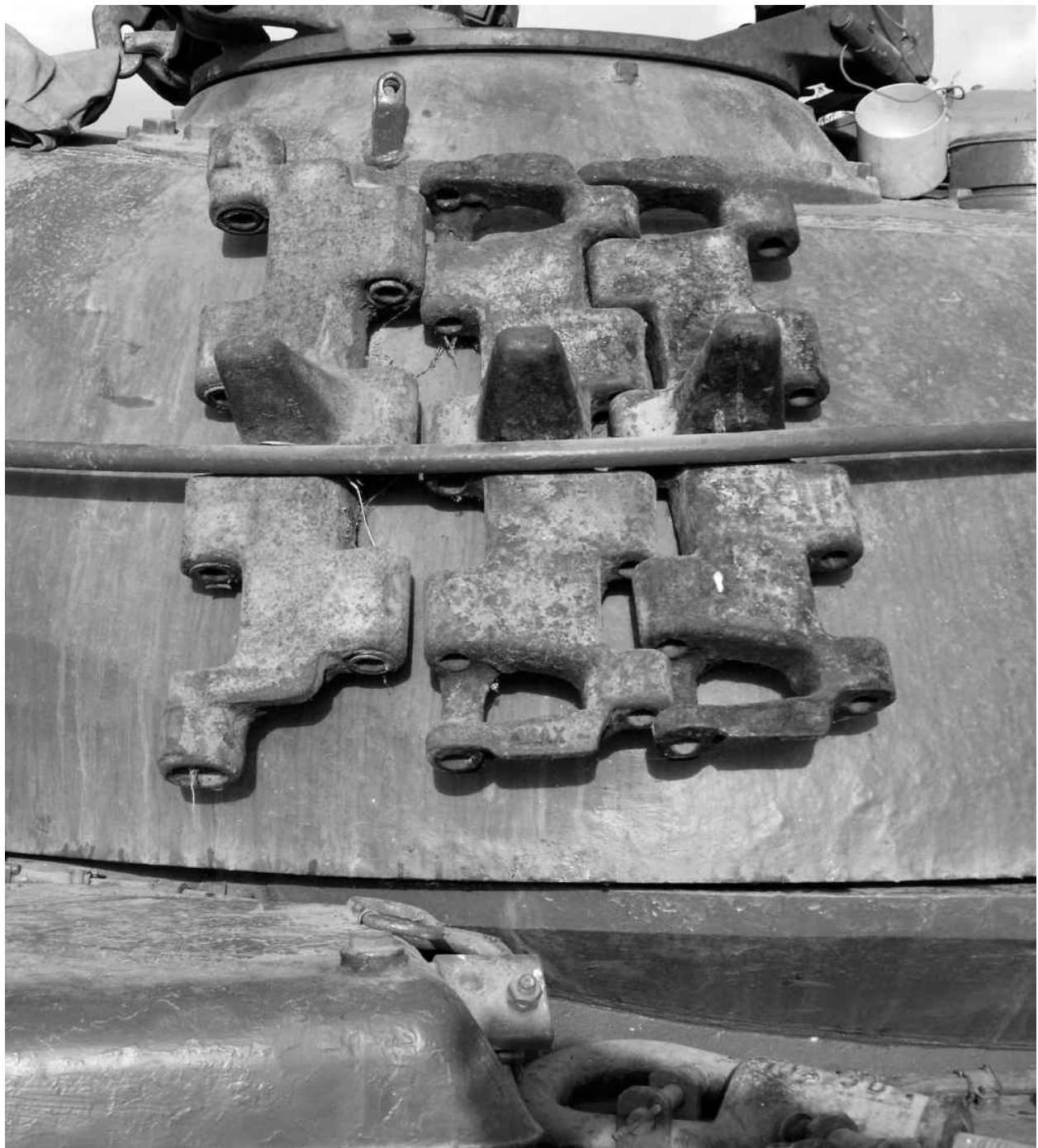
Crude uparmouring using track shoes wedged in the turret handrails.
