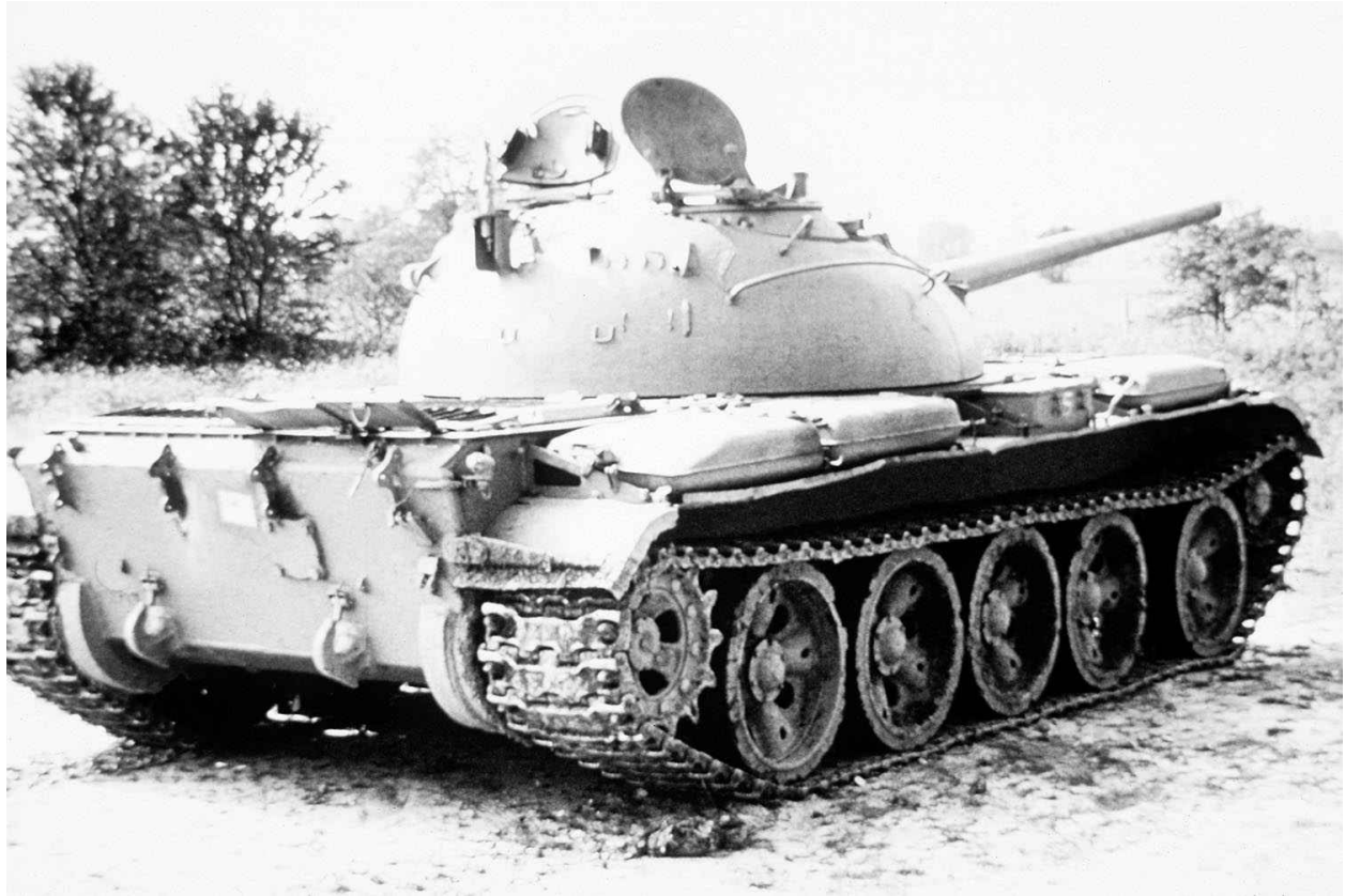
The T-54 Model 1953 introduced a hemispherical turret with no undercuts that became standard on all subsequent T-54/55 models. The twin handrails either side of the turret made their debut with the T-54-1 and were a result of the Soviet Army's paucity of armoured personnel carriers which meant supporting infantry had to hitch a ride.
