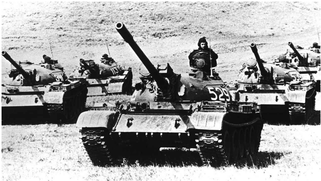
An array of Soviet T-55s on manoeuvres. Only the lead tank and the second from the left are fitted with laser rangefinders over the 100mm gun, which greatly increased its effective range. Note the absence of the loader's cupola with its anti-aircraft machine gun.
