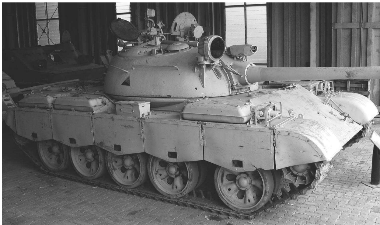
Chinese Type 69-II supplied to the Iraqi Army. Note the laser rangefinder on the top edge of the 100mm gun's mantlet. This was vulnerable to shell splinters and small-arms fire.
