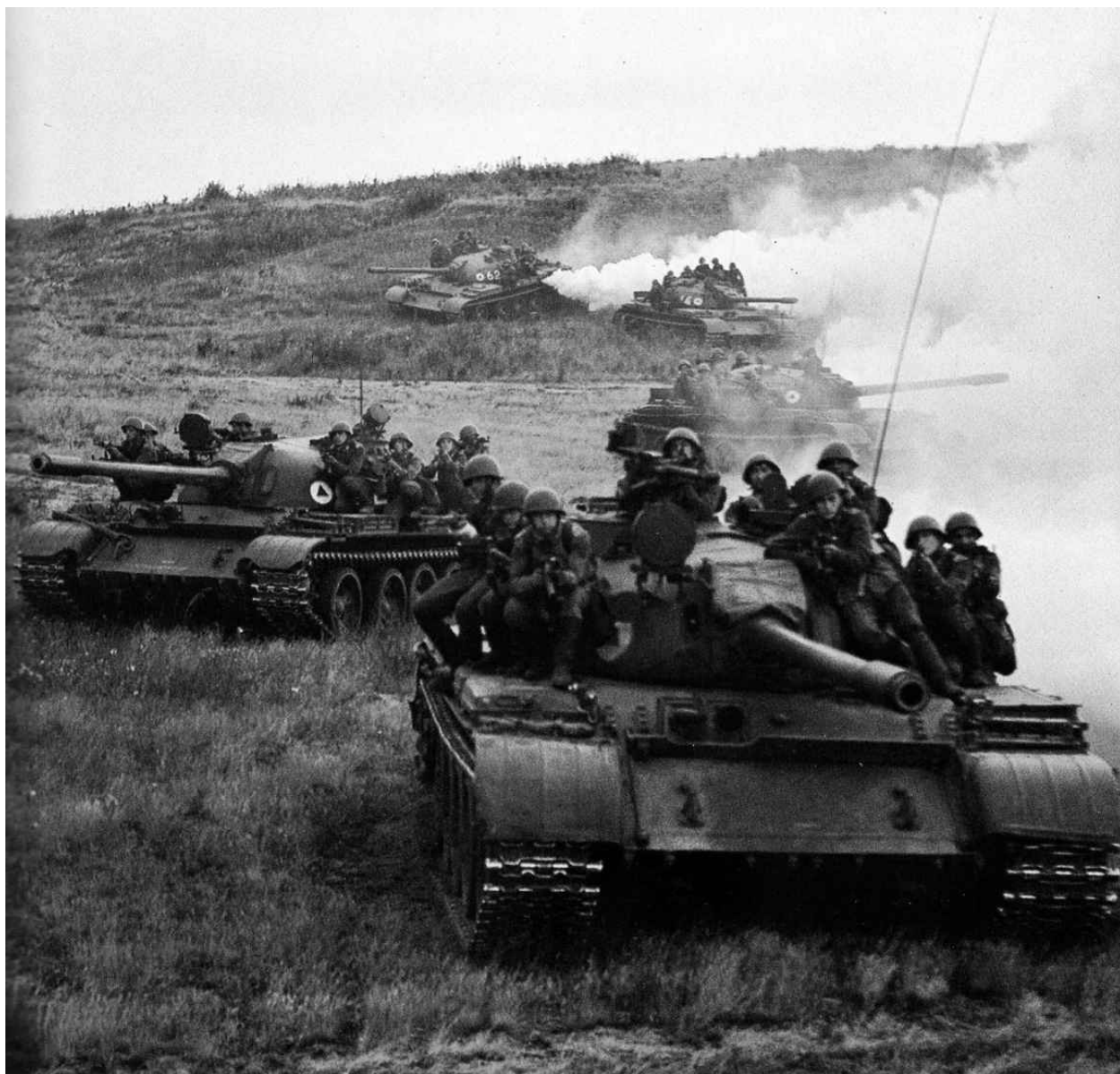
T-55s on exercise with supporting infantry. The T-55A Model 1961 was fitted with an NBC protection system.
