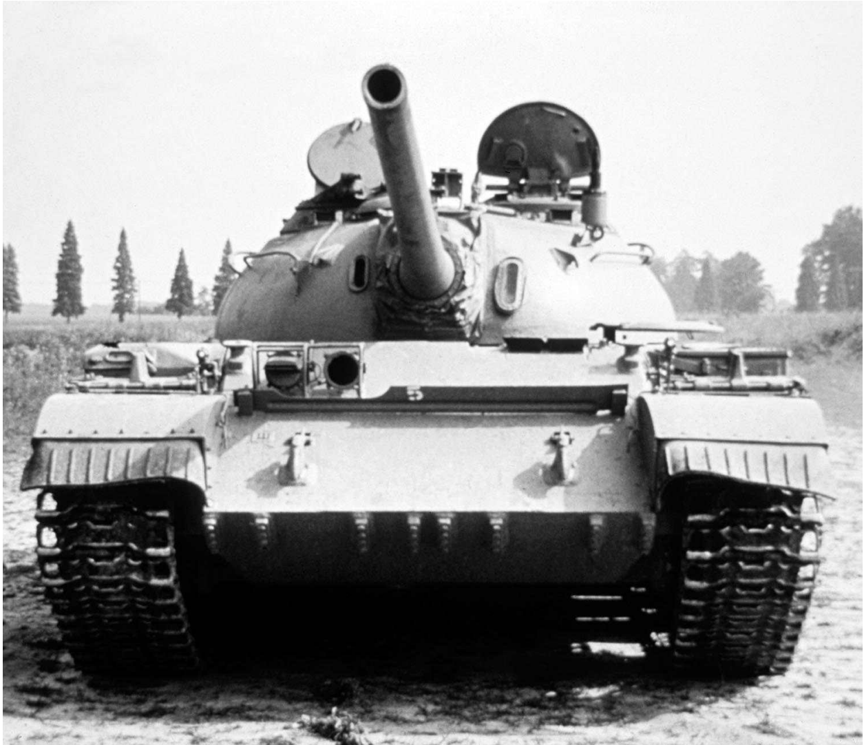
Early T-54 without the fume extractor, which was introduced on the T-54A, or the barrel counterweight. Note the shape of the coaxial machine gun opening and the gunner's sight aperture (left to right), either side of the 100mm gun. On the Czech and Polish-built versions the gunner's aperture is a different shape.
