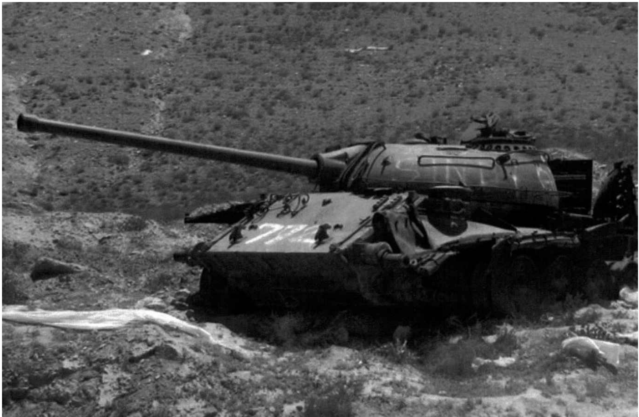
Early-model T-54 in Afghanistan with counterweight on the barrel.
