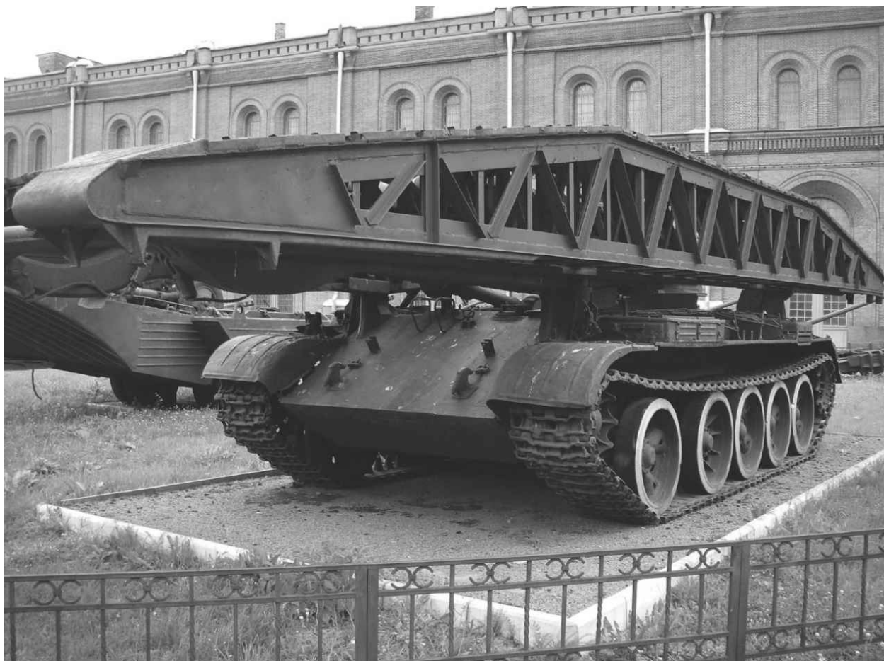
The Soviet-built T-54 MTU-1 bridgelayer was introduced in 1958 to replace an older one based on the T-34. Later versions used the T-55 chassis as well. It took just five minutes to position the bridge.
