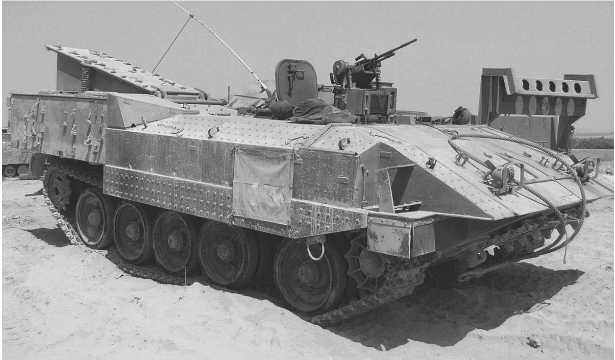
The Israeli Achzarit armoured personnel carrier uses a heavily-converted turretless T-54/55 chassis and entered service in the late 1980s. It can carry a total of ten men including the commander and driver.
