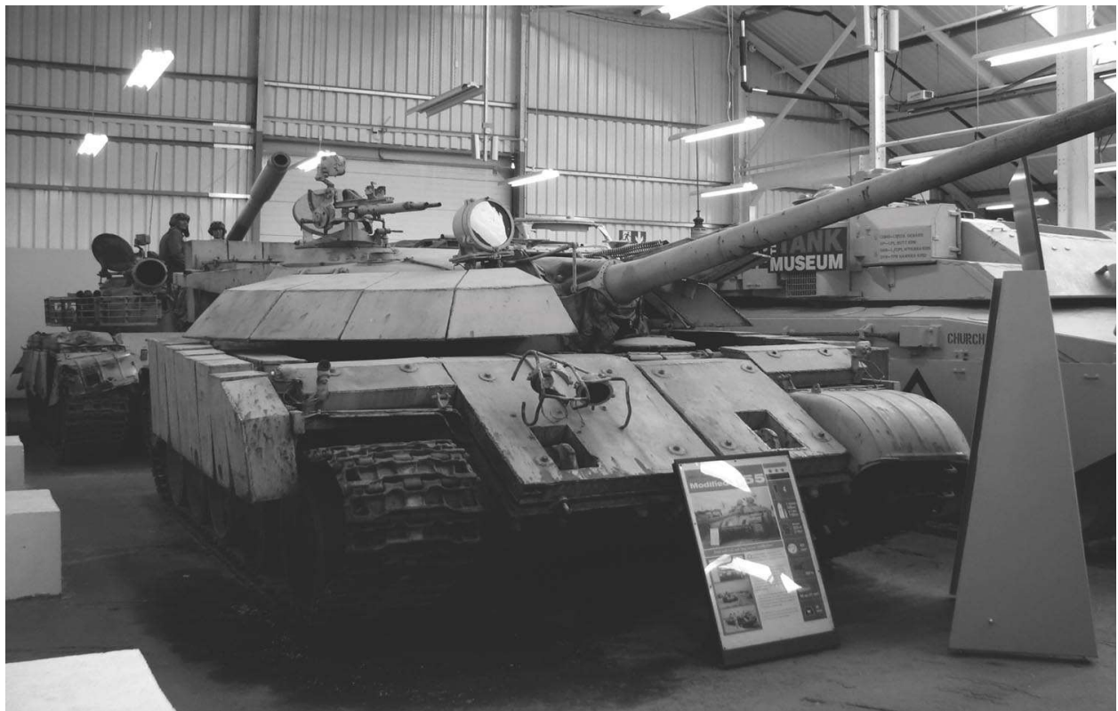
Polish-built T-55 upgraded by the Iraqis with additional frontal passive armour designed to protect it from HEAT rounds.
