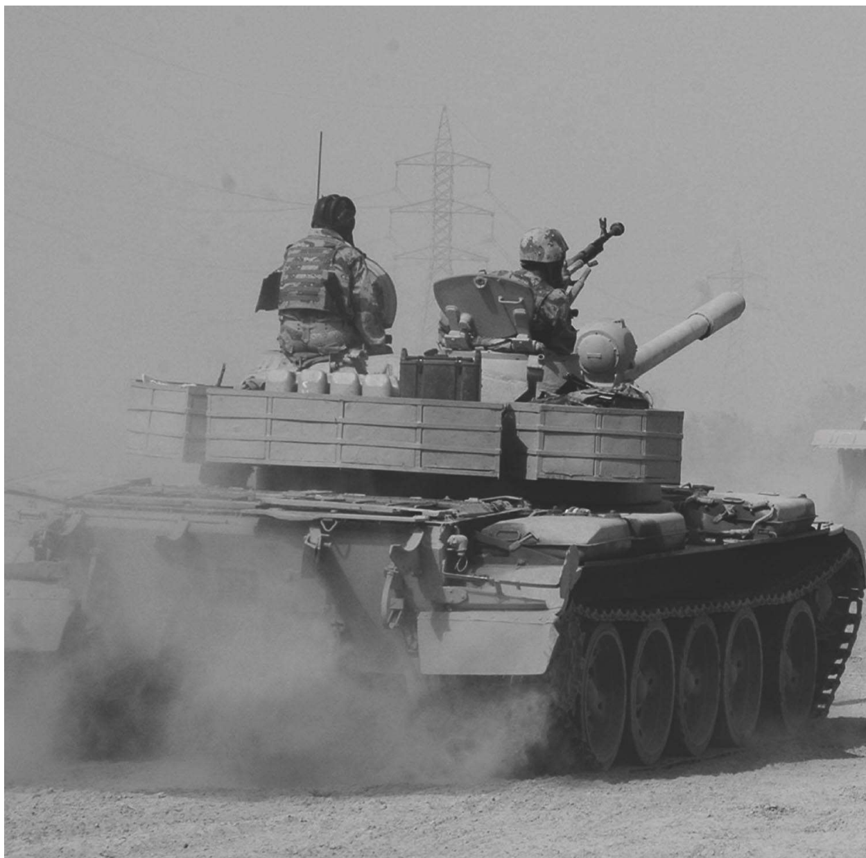
The turret of this refurbished Iraqi T-55 has been fitted with some sort of passive armour system, that looks similar in size and shape to the shields fitted to the Type 69.
