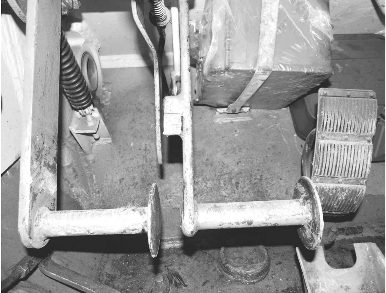
Driver's pedals comprising, left to right, clutch, brake and accelerator. The steering levers are positioned either side.
