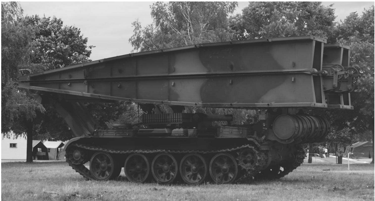
Czech-built MT-55A armoured bridgelayer in travelling configuration – this utilizes a turretless T-55A MBT chassis carrying a scissor bridge. This was exported to at least half a dozen countries
