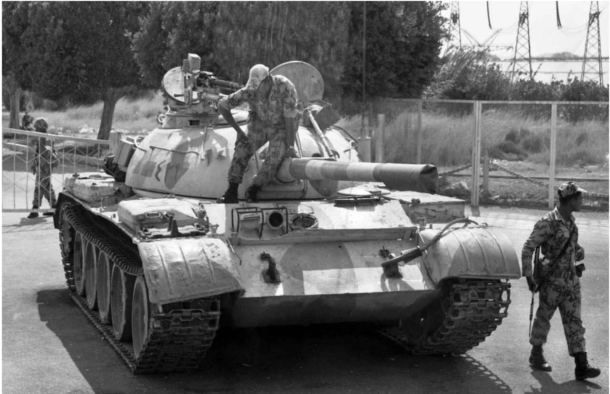
Egyptian T-54 (turret number 421) on guard duty. Note the dust cover on the barrel. It has a two-tone camouflage scheme of sand and light brown.
