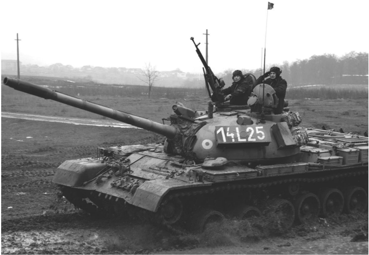
Romanian TR-85 showing the six-wheel configuration and single return roller. It has the Chinese-style laser rangefinder and Polish turret stowage box.
