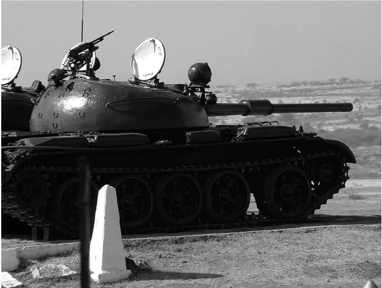
Indian T-54 fitted with a dummy fume extractor making it appear that the 100mm is a 105mm gun. This was done during the 1971 Indo-Pakistan War for recognition purposes as both sides used the T-54/55.
