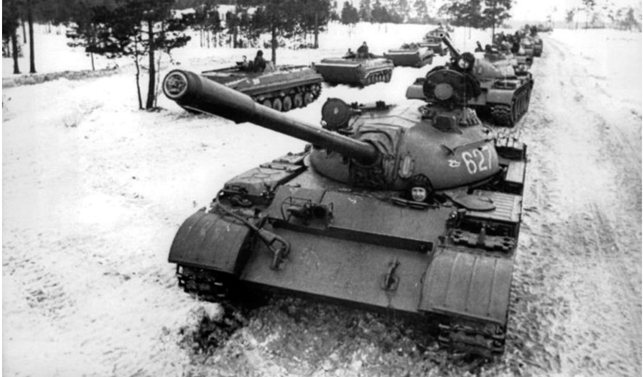
Soviet T-55s, clearly lacking the turret ventilator dome and the loader's cupola. These are probably Model 1961 versions and have the Luna infra-red searchlight. This shows how exposed the commander and driver are with their hatches open.
