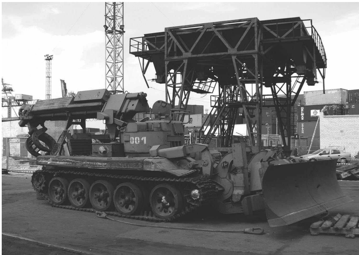
The Soviet IMR was first seen in 1973 and was based on a T-55 chassis. It is equipped with a hydraulic crane with pincher grabs and a dozer blade. Note the large armoured cupola for the crane operator that enabled the vehicle to deploy whilst under fire.
